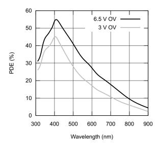
Figure 5: Typical PDE at Peak  $\lambda$  vs. OV
