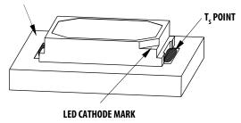
$T_S$  can be easily measured by mounting a thermocouple on the soldering joint as shown in Figure 23. Verify the  $T_S$  of the LED in the final product to ensure that the LEDs are operated within all maximum ratings stated in the data sheet.
