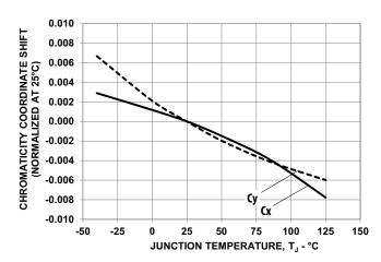
Figure 14: Chromaticity Coordinate Shift vs. Junction Temperature (6500K)
