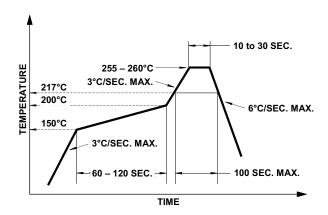
Figure 22: Recommended Board Reflow Direction
