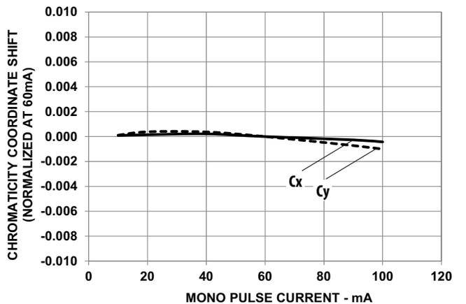
**Figure 9: Chromaticity Coordinate Shift vs. Mono Pulse Current (6500K)**
