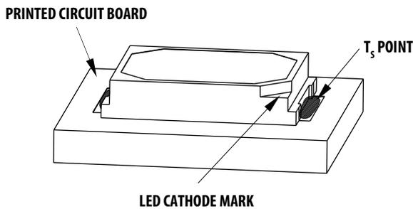
$T_S$  can be easily measured by mounting a thermocouple on the soldering joint as shown in [Figure 23](#). Verify the  $T_S$  of the LED in the final product to ensure that the LEDs are operated within all maximum ratings stated in the data sheet.
