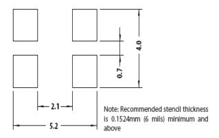
Figure 9: Recommended Soldering Land Pattern
