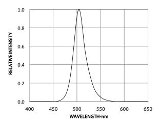
Figure 1: Relative Intensity vs Wavelength
