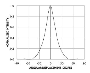
Figure 6a: Radiation Pattern for X axis
