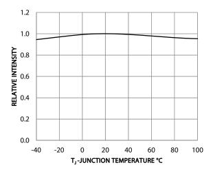
Figure 7: Relative Intensity Shift vs Junction Temperature
