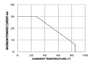
Figure 4: Maximum Forward Current vs Ambient Temperature
