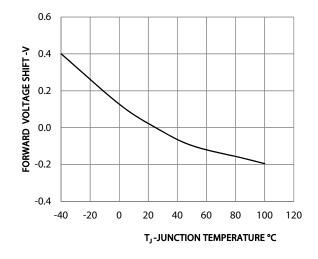
Figure 8: Forward Voltage Shift vs Junction Temperature
