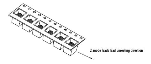
Figure 12 Unit Orientation From Reel
