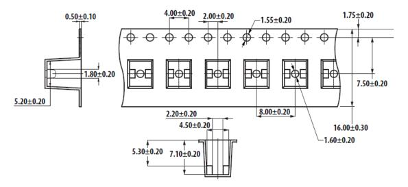
Figure 10 Carrier Tape Dimension
