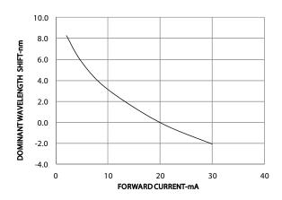
Figure 5: Dominant Wavelength Shift vs Forward Current
