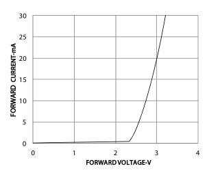
Figure 2: Forward Current vs Forward Voltage
