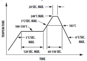
(ii) Lead-free reflow soldering:
