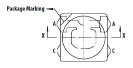
Figure 6b: Component Axis for Radiation Pattern
