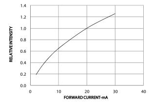
Figure 3: Relative Intensity vs Forward Current
