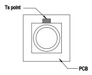
$T_S$  can be easily measured by mounting a thermocouple on the soldering joint as shown in Figure 17, while  $R_{\theta J\text{-}S}$  is provided in the data sheet. Verify the  $T_S$  of the LED in the final product to ensure that the LEDs are operating within all maximum ratings stated in the data sheet.
