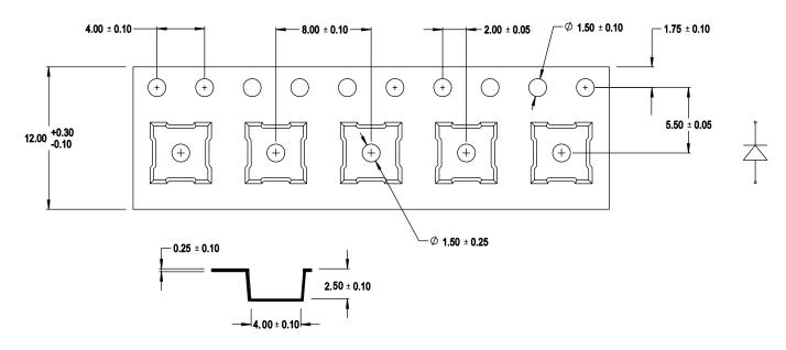
**NOTE:** All dimensions in millimeters (mm).
