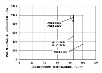
Figure 9: Maximum Forward Current vs. Ambient Temperature for ARE1-8xD0
