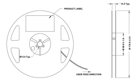
**NOTE:** All dimensions are in millimeters (mm).
