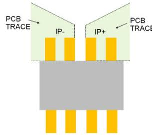
When the connection to the input pin covers only the vertical portion of the input pin, there is a sensitivity variation of about -0.6% versus the recommended PCB trace layout as shown in [Figure 14](#).
