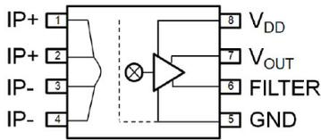
**NOTE:** The connection of a 1-μF bypass capacitor between pins 8 and 5 is recommended.
