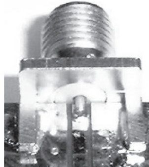
Figure 14 Soldering Details of Connector Fingers to Lower Ground Plane
