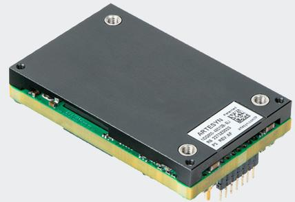
Advanced Energy's Artesyn NDQ900 series quarter-brick non-isolated DC-DC converter provides a single regulated low noise output. It delivers up to 900 W with 12.25 V output voltage and an input range of 40 to 60 VDC. It is designed primarily for use with standard 48 V telecommunications equipment supplies. A PMBus™ interface is also provided for flexible digital control and monitoring. The main application area is in datacom applications.
