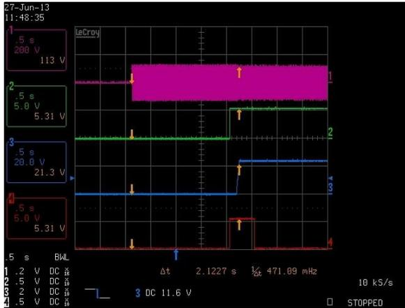
Figure 23: LCM1500Q-T-4 Turn-on delay via AC mains
