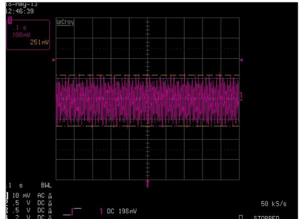
Figure 65: LCM1500W-T-4 Ripple and Noise Measurement
