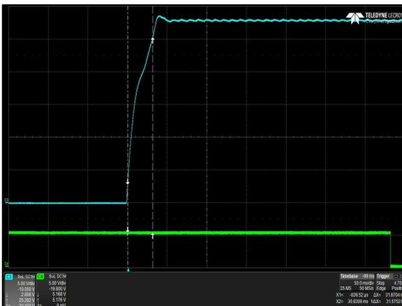
Figure 38: LCM1500R-T-4 Output Voltage Startup
