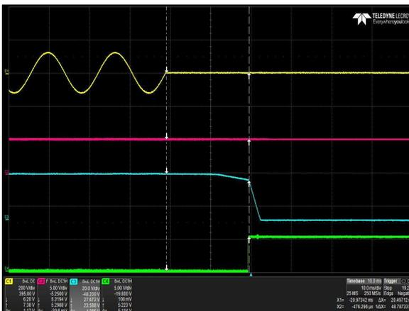
Figure 36: LCM1500R-T-4 Hold-up Time
