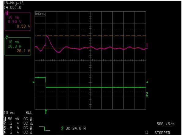
Figure 63: LCM1500W-T-4 Transient Response - Vo Deviation
