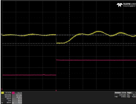
Figure 40: LCM1500R-T-4 Transient Response - Vo Deviation
