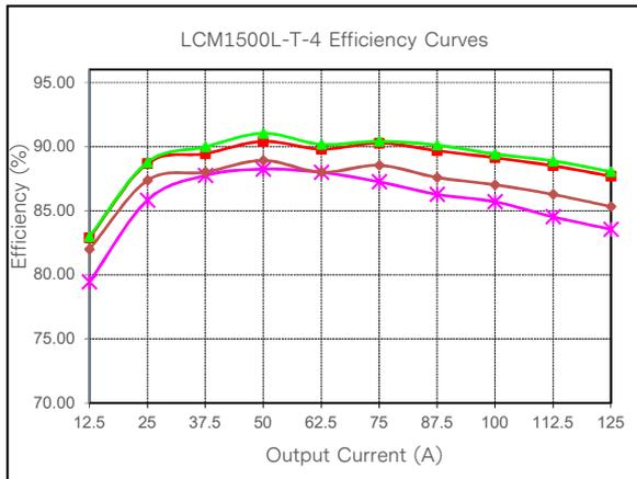
Figure 9: LCM1500L-T-4 Efficiency Curve @ 25°C
