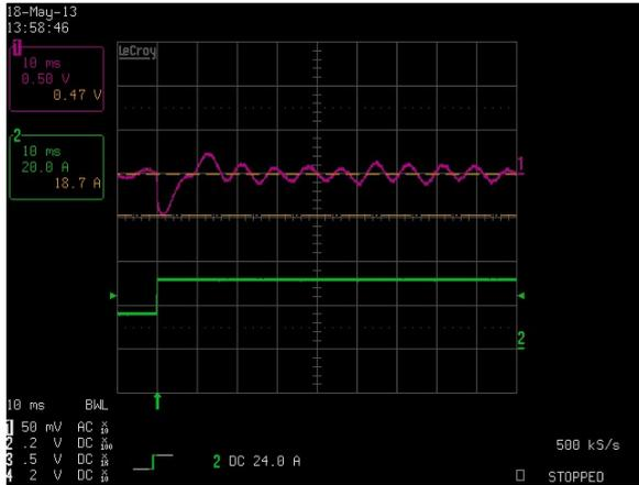
Figure 62: LCM1500W-T-4 Transient Response - Vo Deviation
