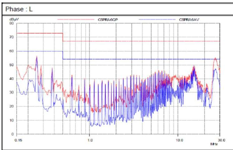
The LCM1500 series have internal EMI filters to ensure the converters' conducted EMI levels comply with EN55022 (FCC Part 15) Class A.
