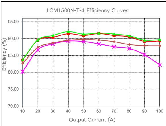
Figure 20: LCM1500N-T-4 Efficiency Curve @ 25°C
