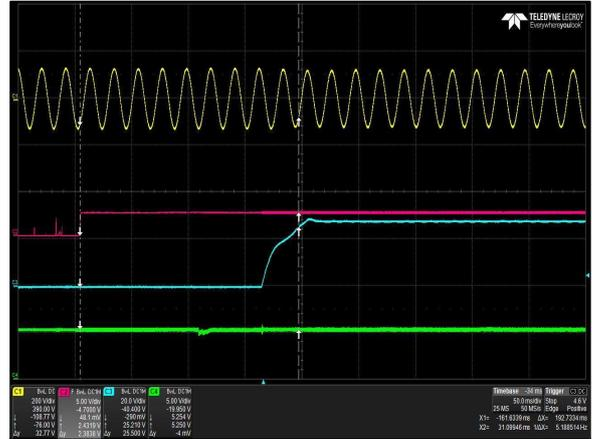
Figure 35: LCM1500R-T-4 Turn-on delay via INH\_EN
