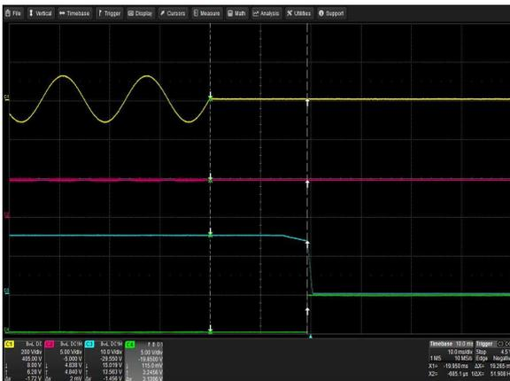
Figure 14: LCM1500N-T-4 Hold-up Time
