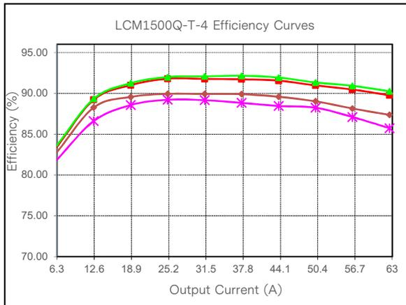
Figure 31: LCM1500Q-T-4 Efficiency Curve @ 25°C
