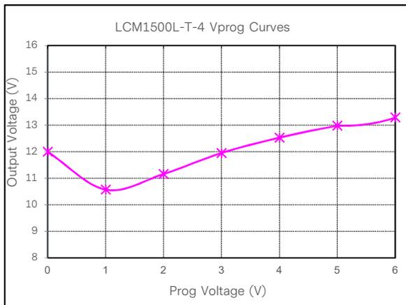
Figure 11: LCM1500L-T-4 Output Voltage Adjustment by Vprog @ 25°C
