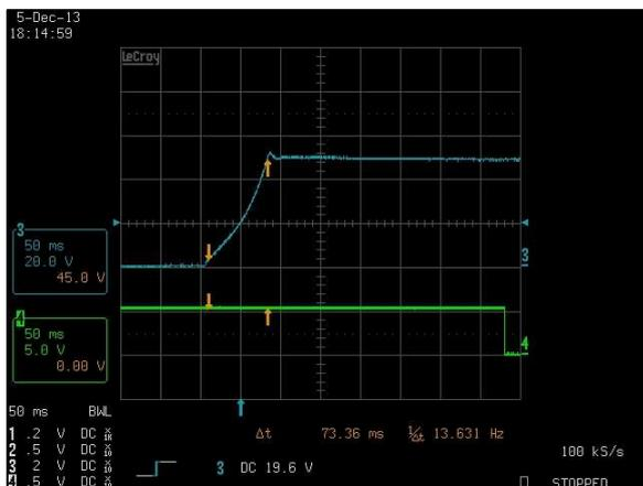
Figure 60: LCM1500W-T-4 Output Voltage Startup
