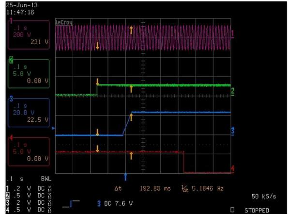
Figure 24: LCM1500Q-T-4 Turn-on delay via INH\_EN
