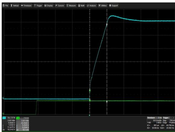
Figure 5: LCM1500L-T-4 Output Voltage Startup
