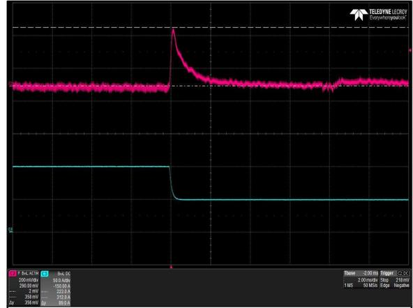
Figure 19: LCM1500N-T-4 Transient Response - Vo Deviation
