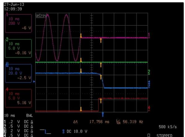
Figure 26: LCM1500Q-T-4 Hold-up Time
