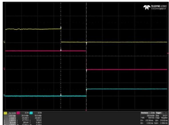
Figure 39: LCM1500R-T-4 Turn Off Characteristic via INH\_EN
