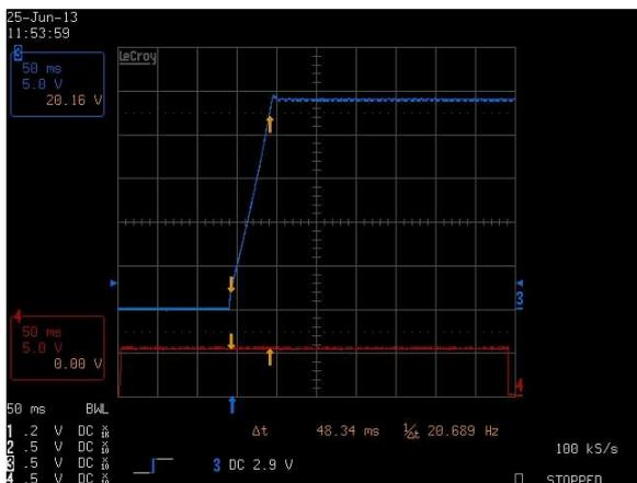
Figure 27: LCM1500Q-T-4 Output Voltage Startup
