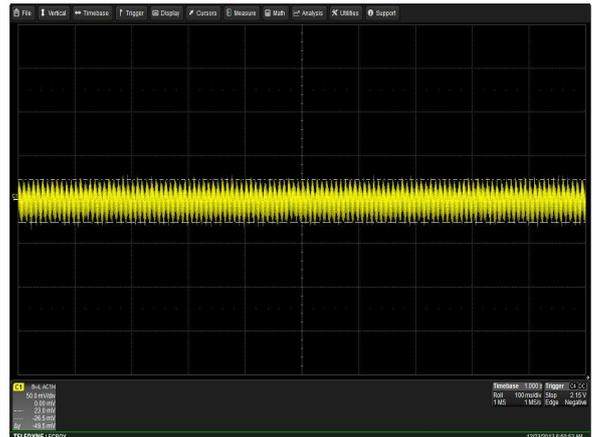
Figure 10: LCM1500L-T-4 Ripple and Noise Measurement
