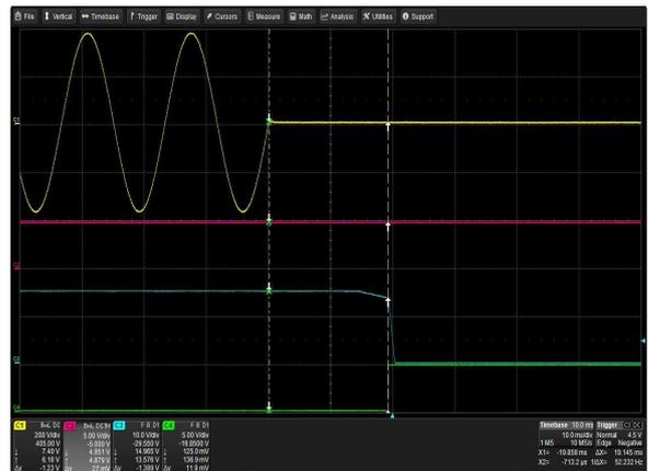
Figure 15: LCM1500N-T-4 Hold-up Time
