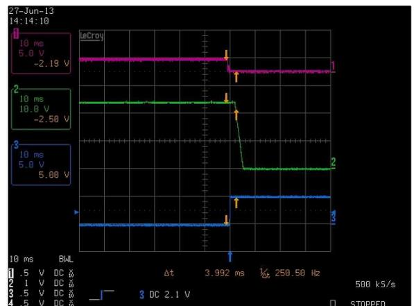
Figure 28: LCM1500Q-T-4 Turn Off Characteristic via INH\_EN
