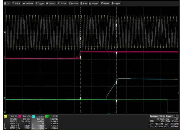
Figure 13: LCM1500N-T-4 Turn-on delay via INH\_EN
