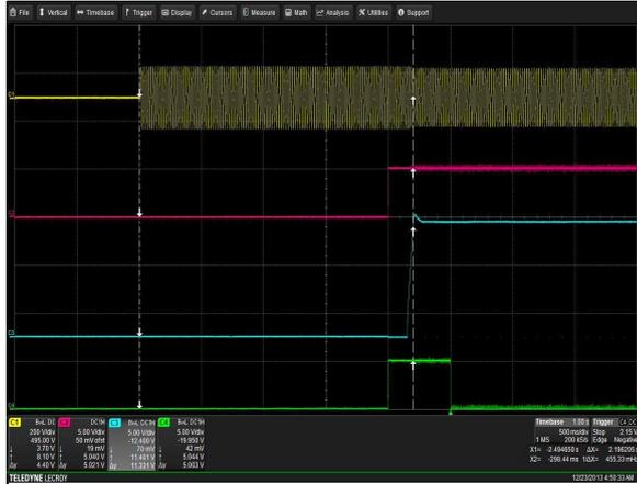
Figure 1: LCM1500L-T-4 Turn-on delay via AC mains
