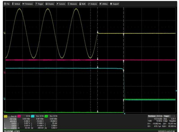
Figure 4: LCM1500L-T-4 Hold-up Time
