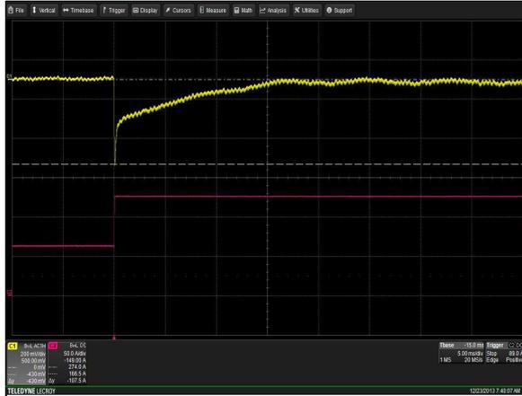
Figure 7: LCM1500L-T-4 Transient Response - Vo Deviation
