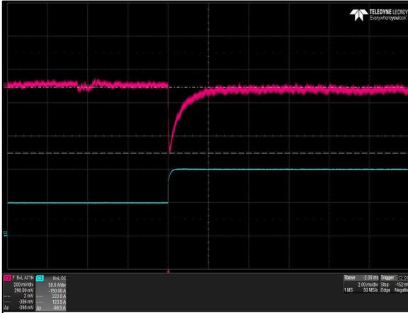
Figure 18: LCM1500N-T-4 Transient Response - Vo Deviation
