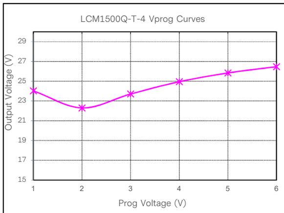
Figure 33: LCM1500Q-T-4 Output Voltage Adjustment by Vprog @ 25°C
