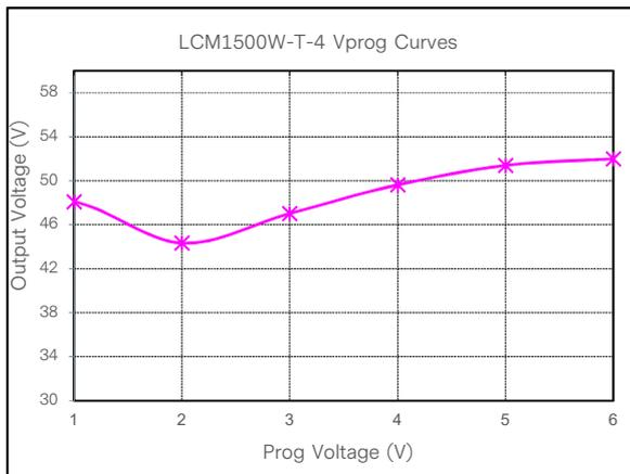
Figure 66: LCM1500W-T-4 Output Voltage Adjustment by Vprog @25°C
