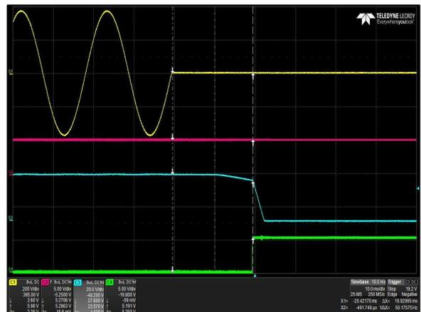
Figure 37: LCM1500R-T-4 Hold-up Time
