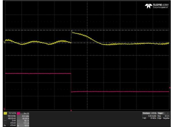
Figure 41: LCM1500R-T-4 Transient Response - Vo Deviation
