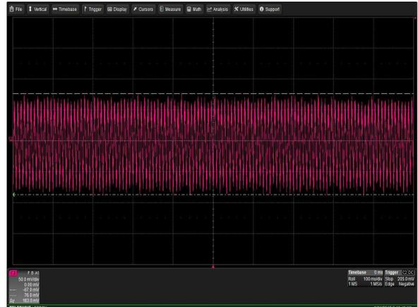
Figure 43: LCM1500R-T-4 Ripple and Noise Measurement
