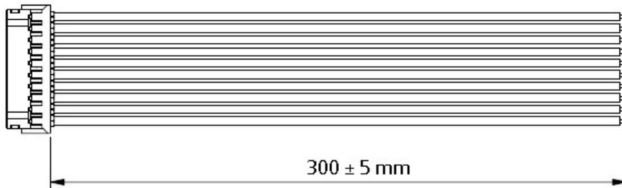
2. Order kit part number 73-788-002 for control connector interface with unloaded housing and 20 pins
