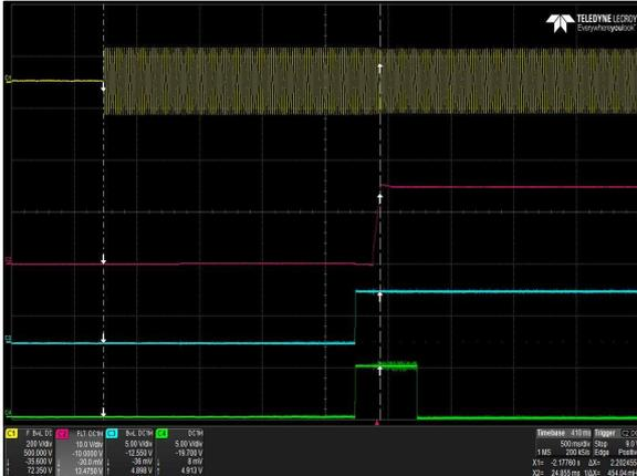
Figure 12: LCM1500N-T-4 Turn-on delay via AC mains
