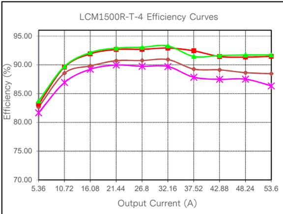
Figure 42: LCM1500R-T-4 Efficiency Curve @ 25°C
