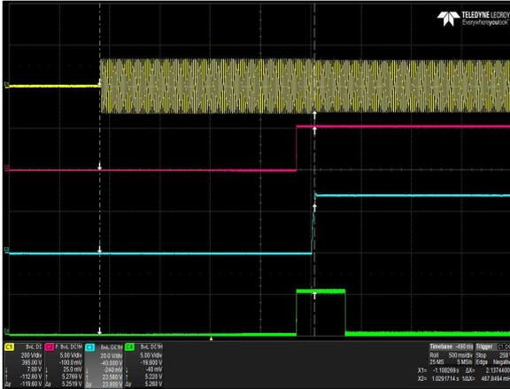
Figure 34: LCM1500R-T-4 Turn-on delay via AC mains
