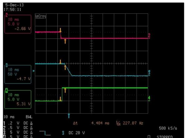
Figure 61: LCM1500W-T-4 Turn Off Characteristic via INH\_EN
