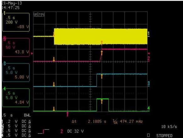
Figure 56: LCM1500W-T-4 Turn-on delay via AC mains
