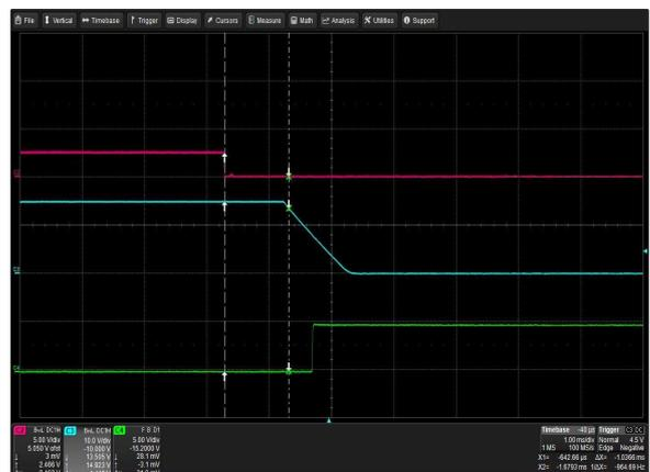
Figure 17: LCM1500N-T-4 Turn Off Characteristic via INH\_EN
