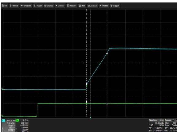
Figure 16: LCM1500N-T-4 Output Voltage Startup
