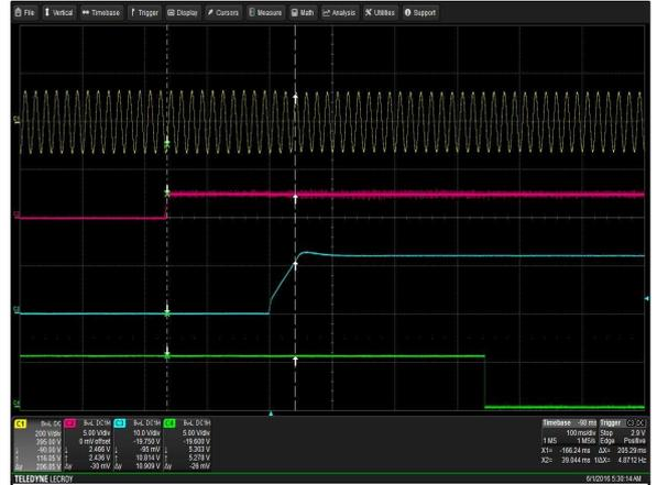
Figure 2: LCM1500L-T-4 Turn-on delay via INH\_EN
