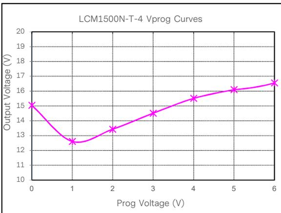
Figure 22: LCM1500N-T-4 Output Voltage Adjustment by Vprog @ 25°C
