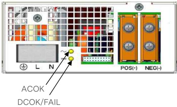
Two user-friendly LEDs for status and diagnostics show status of input power, output power and alarm condition valuable troubleshooting aid to reduce system downtime.
