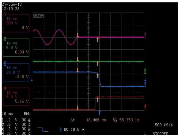
Figure 25: LCM1500Q-T-4 Hold-up Time
