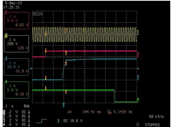
Figure 57: LCM1500W-T-4 Turn-on delay via INH\_EN
