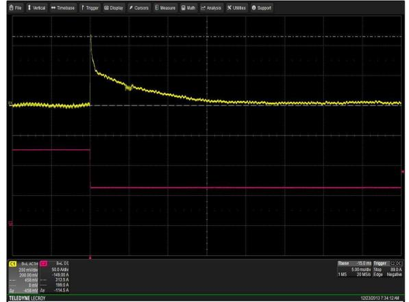
Figure 8: LCM1500L-T-4 Transient Response - Vo Deviation
