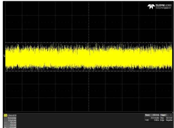
Figure 21: LCM1500N-T-4 Ripple and Noise Measurement
