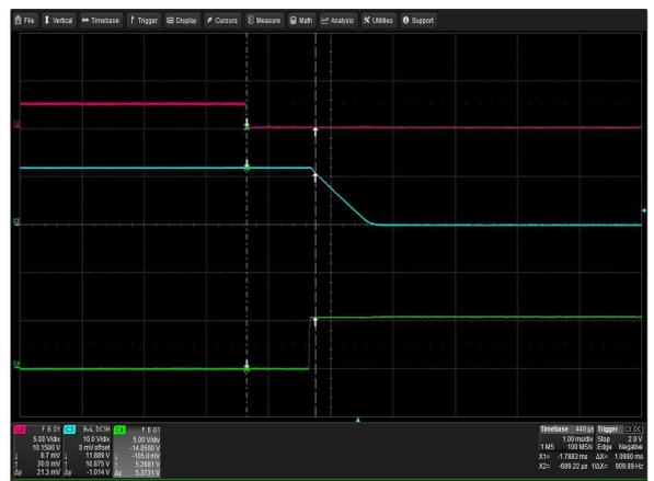
Figure 6: LCM1500L-T-4 Turn Off Characteristic via INH\_EN
