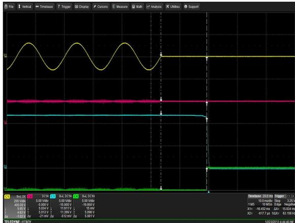
Figure 3: LCM1500L-T-4 Hold-up Time
