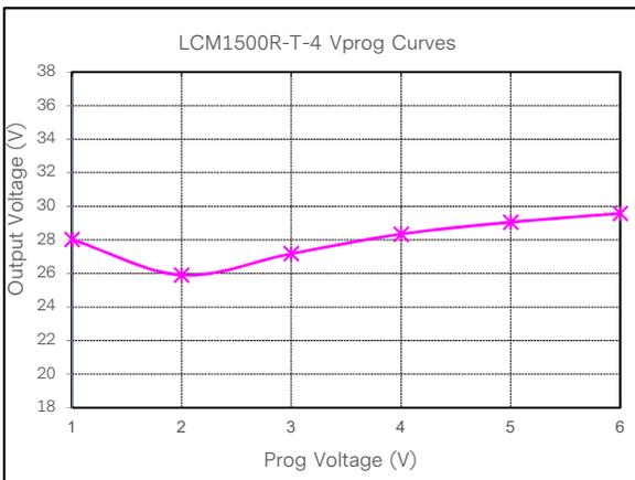
Figure 44: LCM1500R-T-4 Output Voltage Adjustment by Vprog @ 25°C
