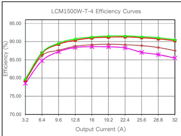
Figure 64: LCM1500W-T-4 Efficiency Curve @ 25°C
