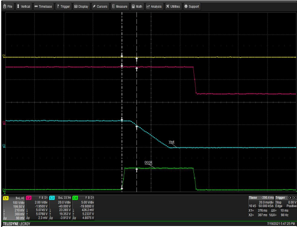
Figure 44: LCM600N DCOK Signal Turn On Delay – Vin = 100Vac Load: Io = 2A (12V), I SB = 0A (5V) Ch 1: AC Mains Ch 2: ACOK Ch 3: Vo Ch 4: DCOK
