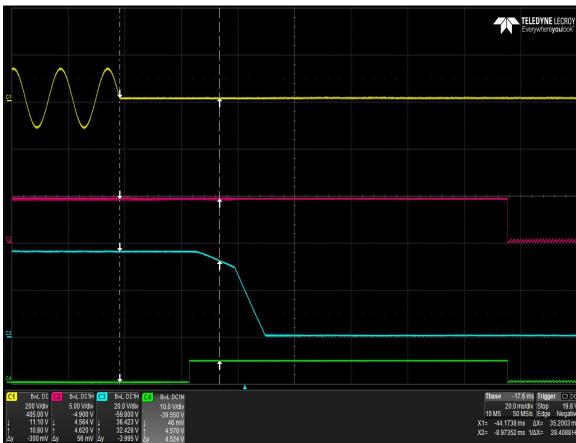
Figure 43: LCC600-36U-9P Hold-up Time Vin = 90Vac / 63Hz / 0° Load: I O = 16.7A (36V), I SB = 1.5A(5V) Ch 1: AC Mains Ch 2: V SB Ch 3: V O CH 4: G_DCOK_C
