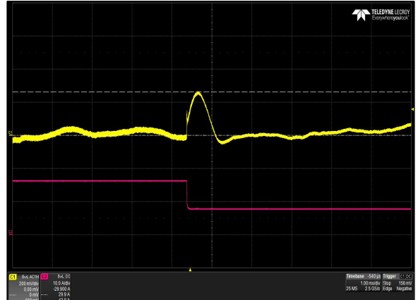
Figure 58: LCC600-36H-9P Transient Response - V_O Deviation 100% to 50% load change 1A/uS slew rate V_{in} = 277V_{ac} Ch 1: V_O Ch 2: I_O
