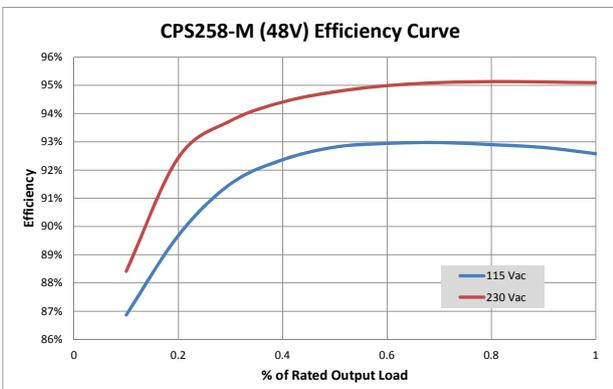
Figure 5. Typical Efficiency for 48 V Output
