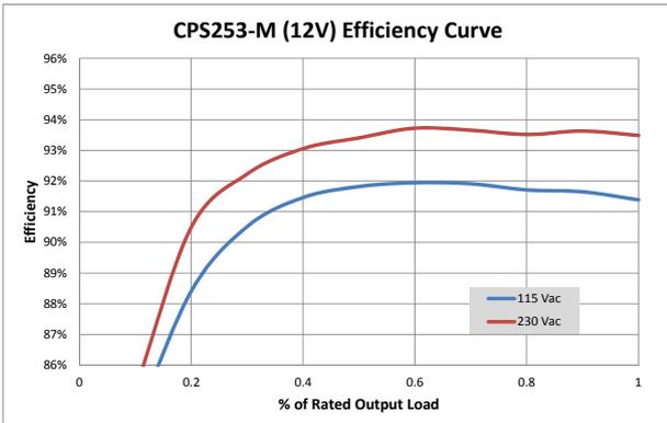
Figure 3. Typical Efficiency for 12 V Output
