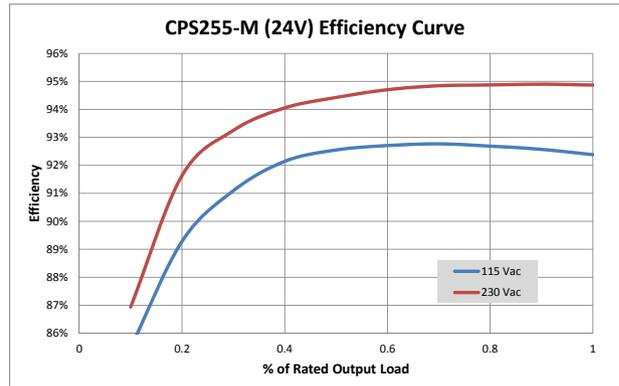
Figure 4. Typical Efficiency for 24 V Output
