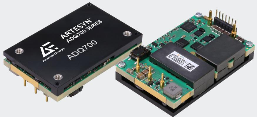
ADQ700 series quarter-brick isolated DC-DC converters produce a single fully regulated 12 V output. Rated at 700 watts, these converters can deliver up to 58 amps output current and have no minimum load requirement. They have an input voltage range of 40 to 60 V and are primarily designed for use with standard 48 V supplies in computing and server applications, as well as regulated 48V supplies in communications equipment.
