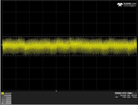
Figure 6: LPS363-M Ripple and Noise Measurement
