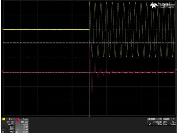
Figure 33: LPS366-M Inrush Current
