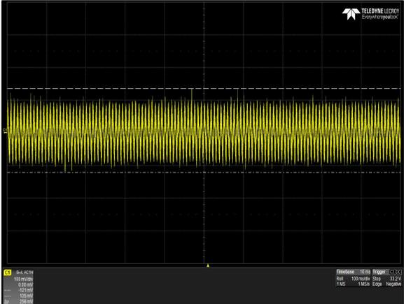
Figure 36: LPS366-M Ripple and Noise Measurement
