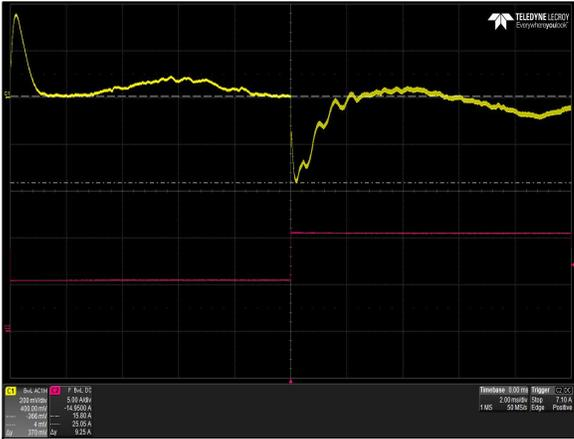
Figure 38: LPS366-M Transient Response – Vo Deviation
