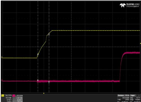
Figure 25: LPS365-M Output Voltage Startup Characteristic
