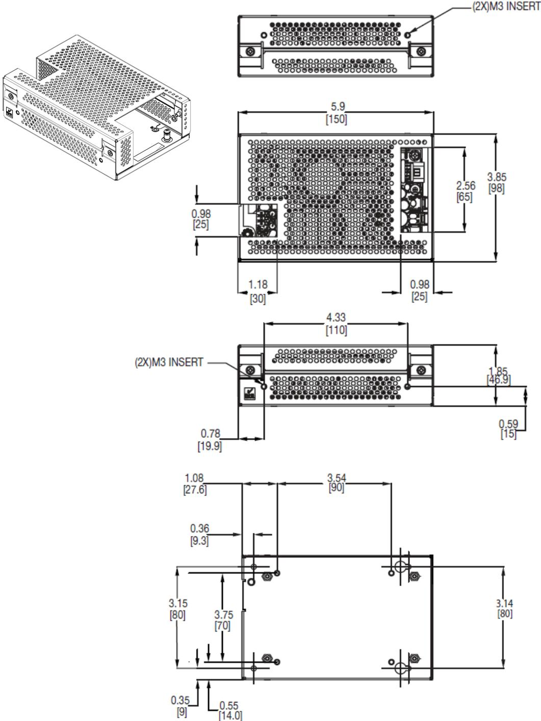
Note: All dimensions in inches (mm), tolerance is 0.02" (±0.5mm)
