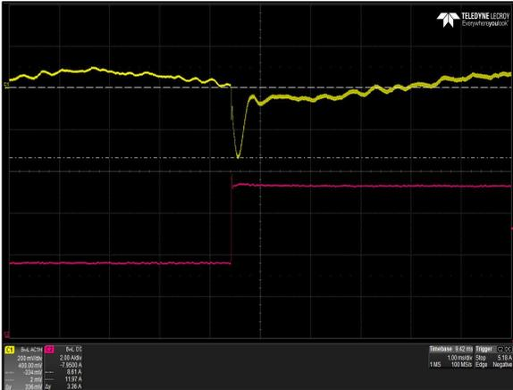
Figure 48: LPS368-M Transient Response – Vo Deviation
