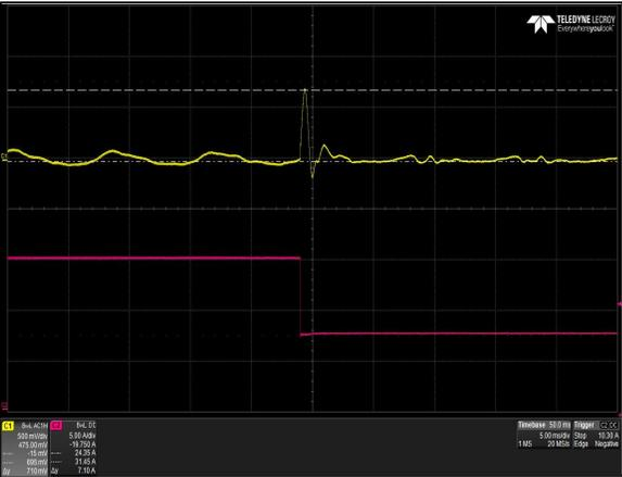
Figure 27: LPS365-M Transient Response – Vo Deviation
