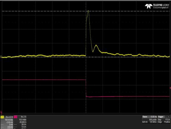
Figure 17: LPS364-M Transient Response – Vo Deviation
