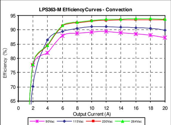
Figure 9: LPS363-M Efficiency Curves @ 25 degC
