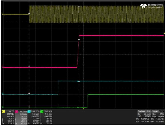
Figure 41: LPS368-M Turn-on delay
