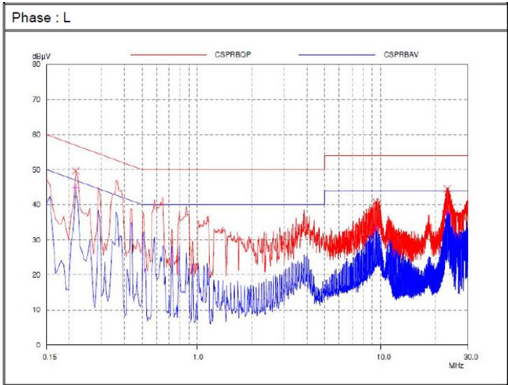
The LPS360-M series power supply have internal EMI filters to ensure the convertor’s conducted EMI levels comply with EN55032 (FCC Part 15) Class B and EN55032 (CISPR 22) Class B limits. The EMI measurements are performed with resistive loads under forced air convection at maximum rated loading.
