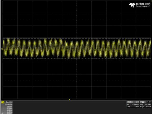
Figure 16: LPS364-M Ripple and Noise Measurement
