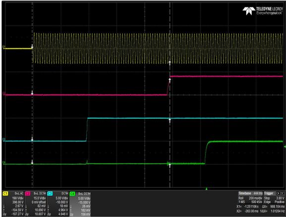
Figure 1: LPS363-M Turn-on delay
