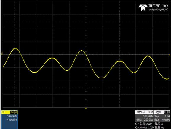
Figure 34: LPS366-M Input Current Waveform
