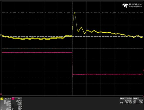
Figure 47: LPS368-M Transient Response – Vo Deviation
