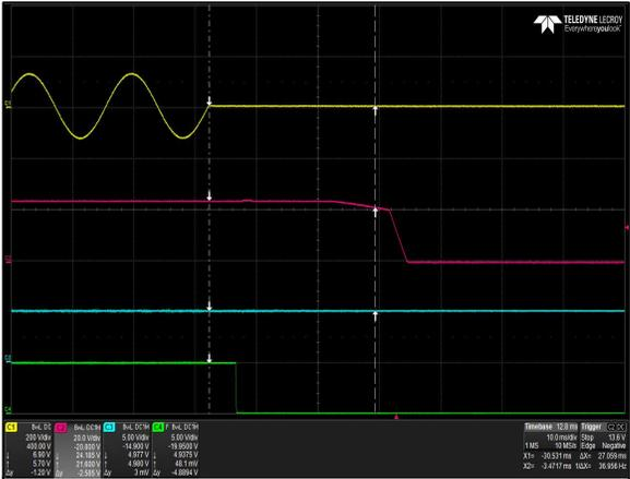
Figure 22: LPS365-M Hold-up Time (time to decay)
