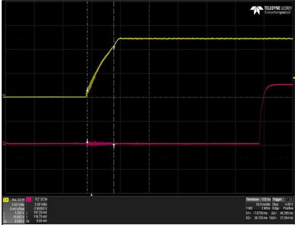
Figure 5: LPS363-M Output Voltage Startup Characteristic
