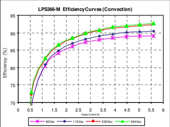
Figure 39: LPS366-M Efficiency Curves @ 25 degC
