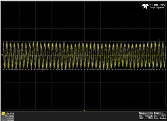
Figure 36: LPS365-M Ripple and Noise Measurement
