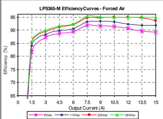
Figure 30: LPS365-M Efficiency Curves @ 25 degC
