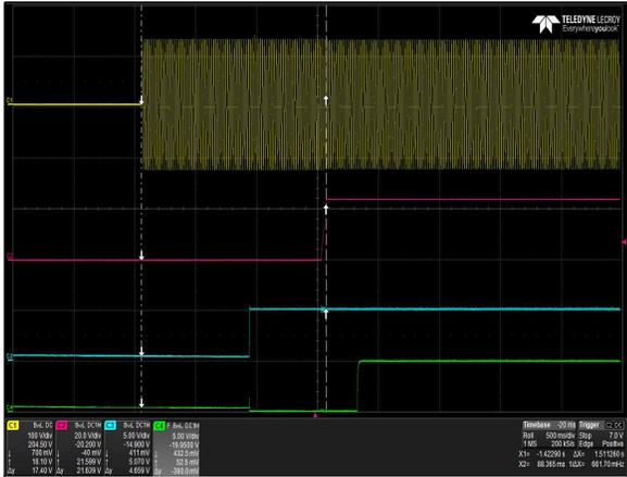
Figure 21: LPS365-M Turn-on delay
