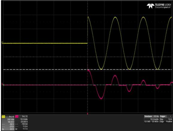
Figure 3: LPS363-M Inrush Current
