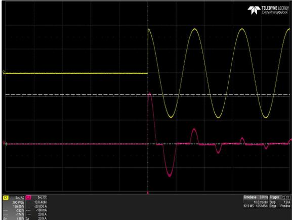
Figure 13: LPS364-M Inrush Current
