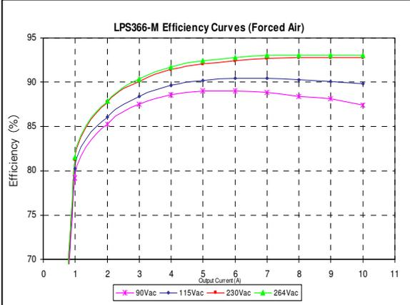
Figure 40: LPS366-M Efficiency Curves @ 25 degC
