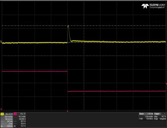
Figure 7: LPS363-M Transient Response – Vo Deviation
