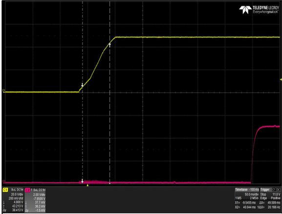
Figure 45: LPS368-M Output Voltage Startup Characteristic
