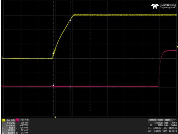
Figure 15: LPS364-M Output Voltage Startup Characteristic
