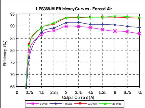
Figure 50: LPS368-M Efficiency Curves @ 25 degC
