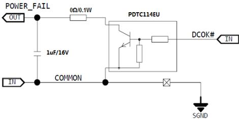
Power Fail signal circuit diagram
