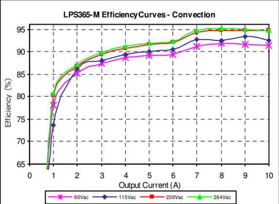
Figure 29: LPS365-M Efficiency Curves @ 25 degC
