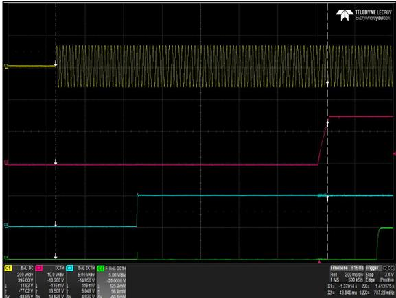
Figure 11: LPS364-M Turn-on delay
