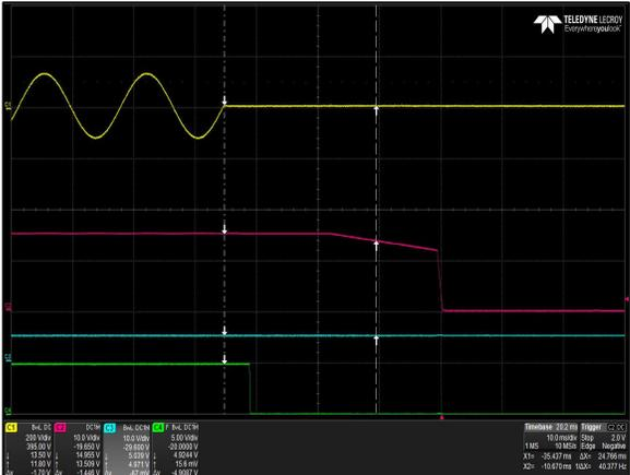
Figure 12: LPS364-M Hold-up Time (time to decay)
