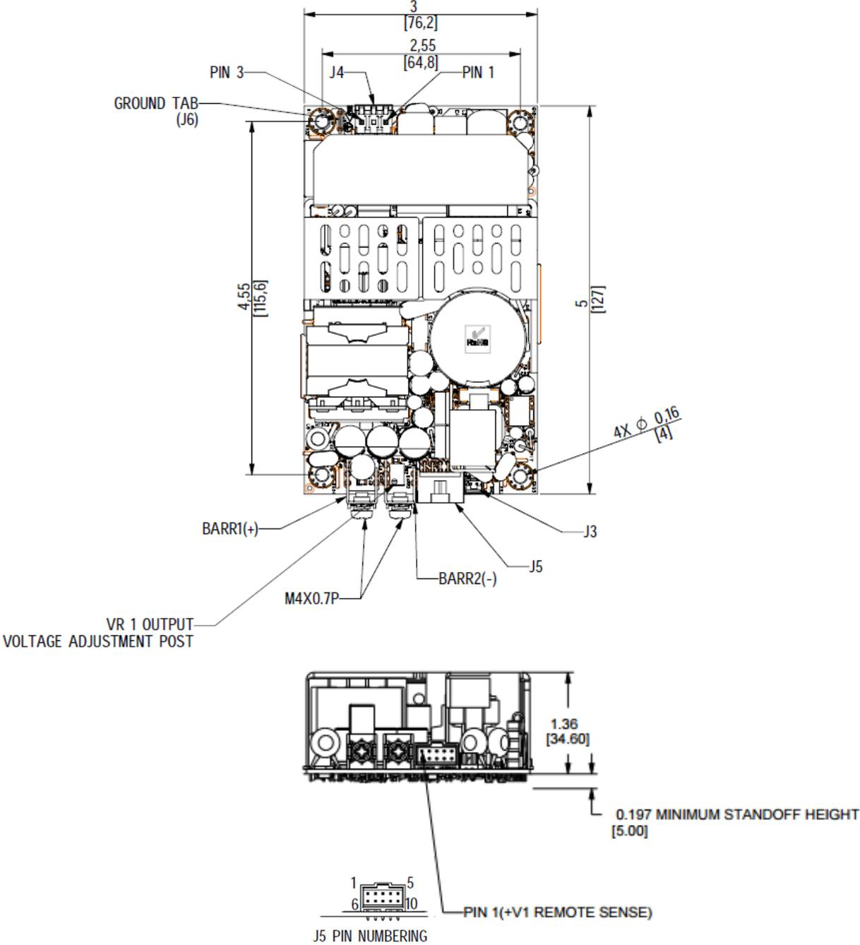
Note: All dimensions in inches (mm), tolerance is 0.02" ( $\pm 0.5$ mm)
