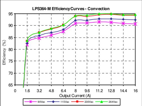
Figure 19: LPS364-M Efficiency Curves @ 25 degC
