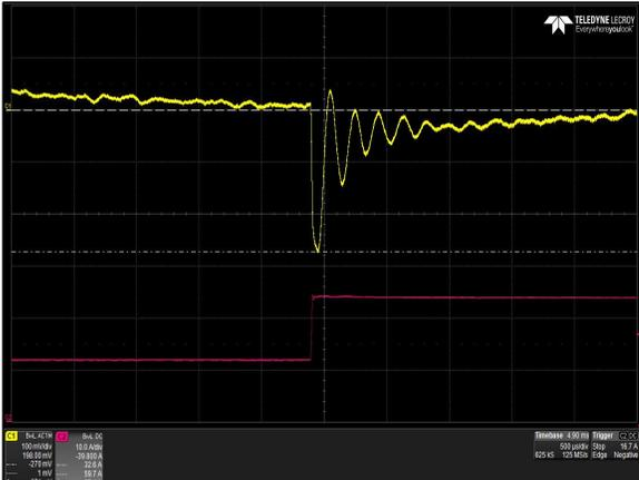
Figure 18: LPS364-M Transient Response – Vo Deviation
