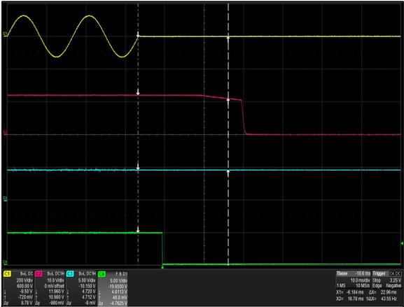
Figure 2: LPS363-M Hold-up Time (time to decay)
