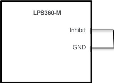
Inhibit the power supply connection
