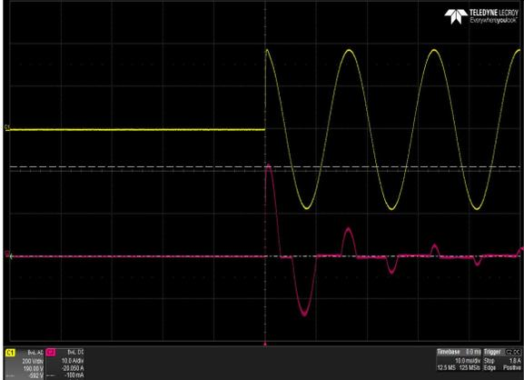
Figure 23: LPS365-M Inrush Current
