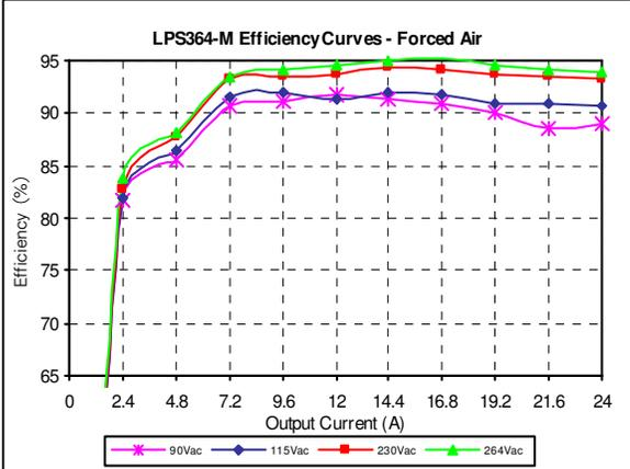
Figure 20: LPS364-M Efficiency Curves @ 25 degC
