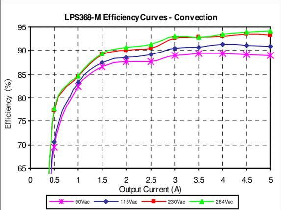
Figure 49: LPS368-M Efficiency Curves @ 25 degC
