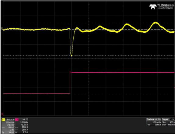
Figure 28: LPS365-M Transient Response – Vo Deviation
