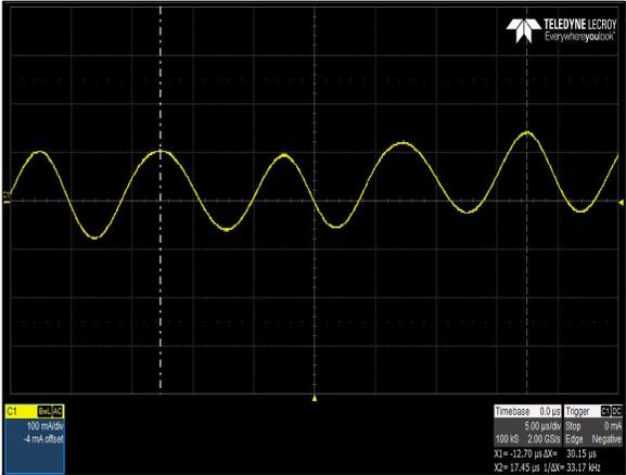
Figure 44: LPS368-M Input Current Waveform
