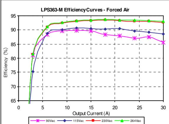
Figure 10: LPS363-M Efficiency Curves @ 25 degC
