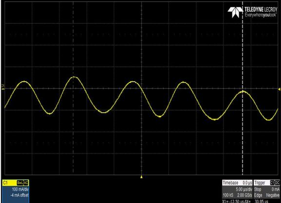
Figure 24: LPS365-M Input Current Waveform
