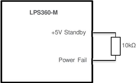
Power Fail signal circuit diagram
