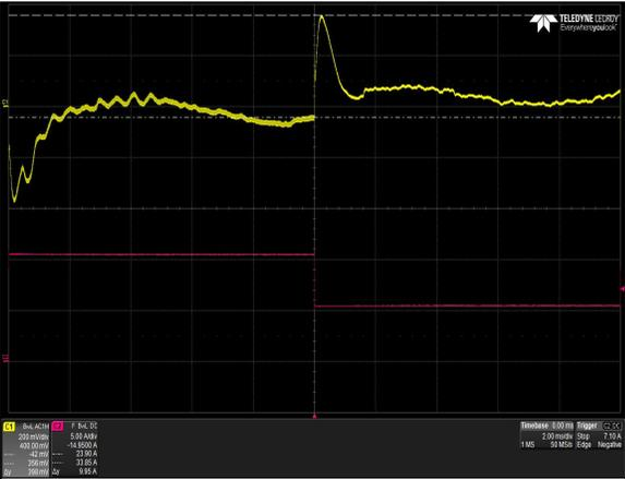
Figure 37: LPS366-M Transient Response – Vo Deviation
