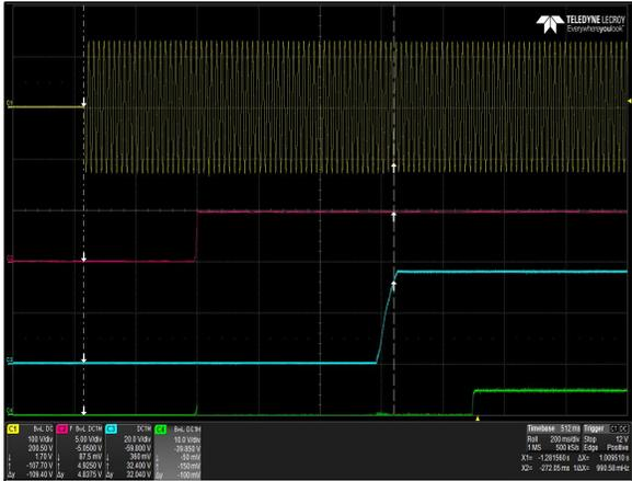
Figure 31: LPS366-M Turn-on delay
