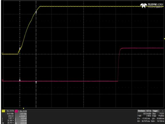
Figure 35: LPS366-M Output Voltage Startup Characteristic
