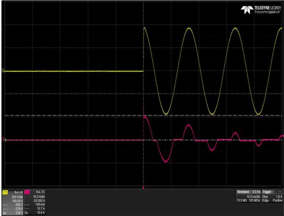
Figure 43: LPS368-M Inrush Current
