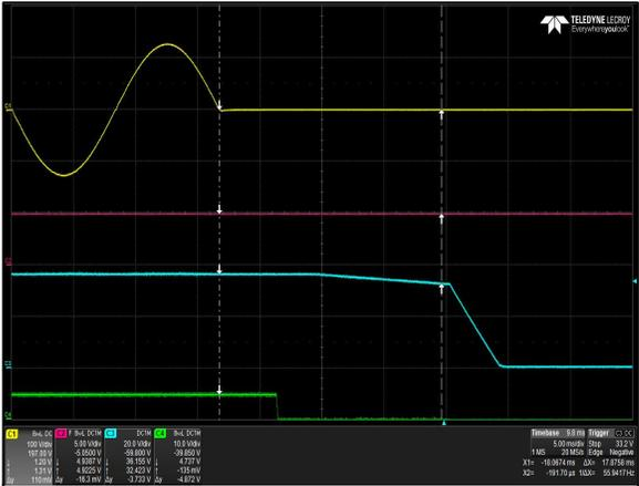
Figure 32: LPS366-M Hold-up Time (time to decay)
