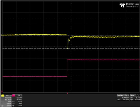
Figure 8: LPS363-M Transient Response – Vo Deviation
