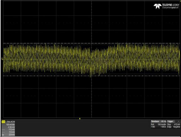
Figure 46: LPS368-M Ripple and Noise Measurement
