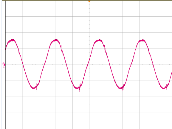
Figure 1: AVD85B-48S12 Output Ripple Waveform 1uS/div Ch 4: I_{IN} (20mA/div)
