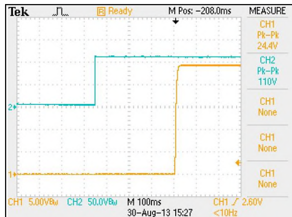
Figure 69: ERM03H110 Output Voltage Startup Characteristic by Vin Vin = 110Vdc Load: Io = 3.125A Ch1: Vo Ch2: Vin
