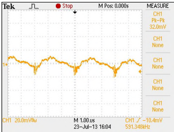
Figure 30: ERM03H72 Ripple and Noise Measurement Vin = 72Vdc Load: Io = 3.125A Ch 1: Vo
