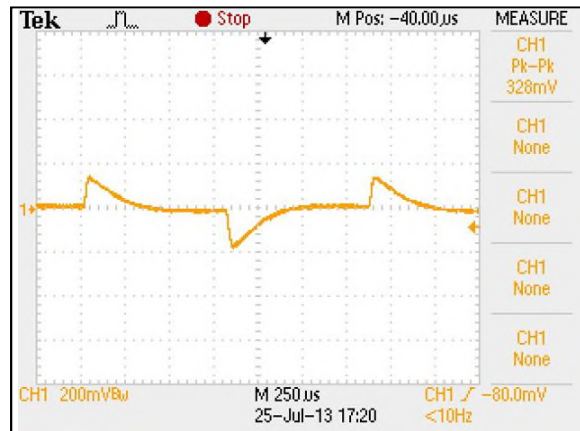
Figure 4: ERM15A72 Transient Response Vin = 72Vdc Load: Io = 100% to 75% load change Ch 1: Vo
