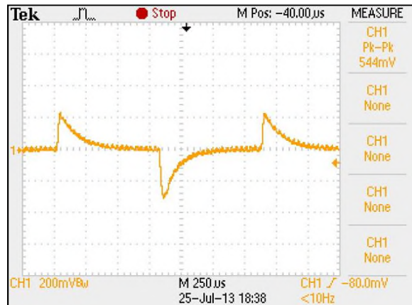
Figure 67: ERM03H110 Transient Response Vin = 110Vdc Load: Io = 100% to 75% load change Ch 1: Vo
