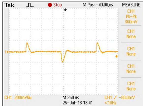
Figure 49: ERM06B110 Transient Response Vin = 110Vdc Load: Io = 100% to 75% load change Ch 1: Vo
