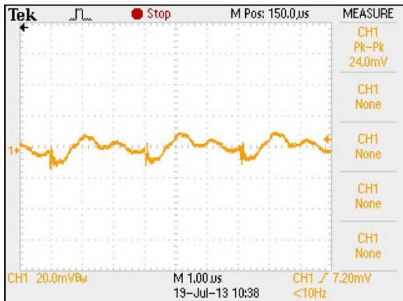
Figure 48: ERM06B110 Ripple and Noise Measurement Vin = 110Vdc Load: Io = 6.25A Ch 1: Vo
