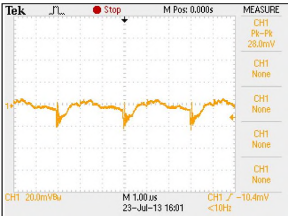
Figure 12: ERM06B72 Ripple and Noise Measurement Vin = 72Vdc Load: Io = 6.25A Ch 1: Vo
