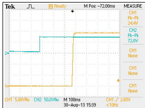
Figure 33: ERM03H72 Output Voltage Startup Characteristic by Vin Vin = 72Vdc Load: Io = 3.125A Ch1: Vo Ch2: Vin
