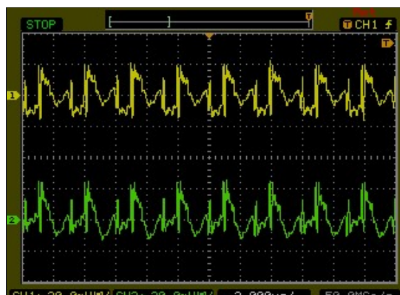
Figure 57: AXA00CC18-L Ripple and Noise Measurement Vin = 24Vdc Load: Io = \pm 0.67 A Ch 1: Vo1 Ch2: Vo2
