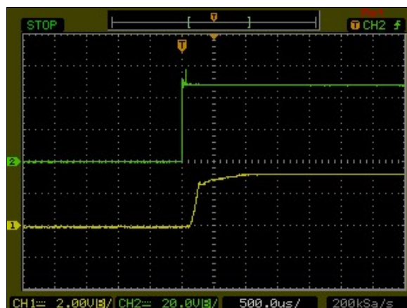
Figure 69: AXA04F36-L Output Voltage Startup Characteristic by Vin Vin = 48Vdc Load: Io = 4.5A Ch1: Vo Ch2: Vin
