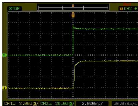
Figure 78: AXA04A36-L Output Voltage Startup Characteristic by Vin Vin = 48Vdc Load: Io = 4A Ch1: Vo Ch2: Vin
