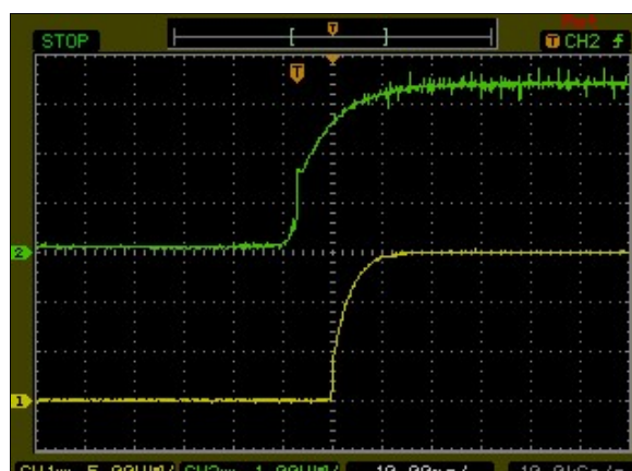
Figure 59: AXA00CC18-L Output Voltage Startup Characteristic by ON/OFF Vin = 24Vdc Load: Io = \pm 0.67 A Ch1: Vo Ch2: Remote On/Off
