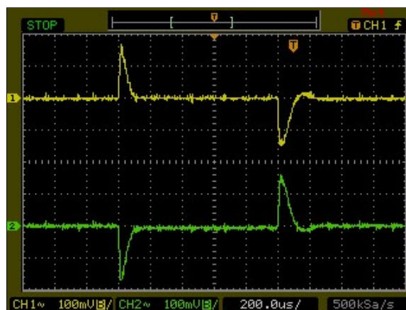
Figure 102: AXA00BB36-L Transient Response Vin = 48Vdc Load: Io = 100% to 75% load change Ch 1: Vo1 Ch2:Vo2
