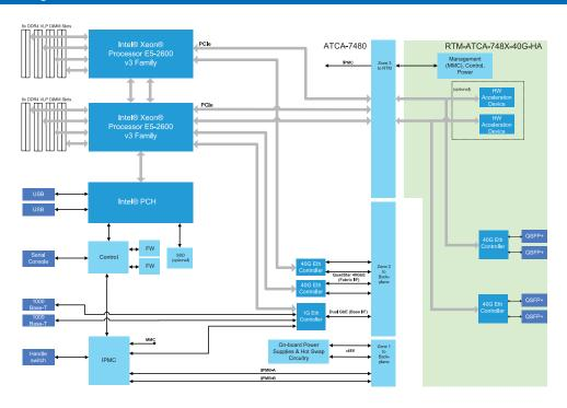
The ATCA-7480 features two Intel® Xeon® E5-2600 v3 family processors with high bandwidth data paths to all memory and I/O resources. The board power and cooling design has been optimized for processor derivatives supporting highest core count per socket (max. 12 cores per CPU) and highest available clock frequencies (up to 2.5GHz at 12 cores). Depending on the applications need, derivatives with lower core count and frequency selections can be used.
