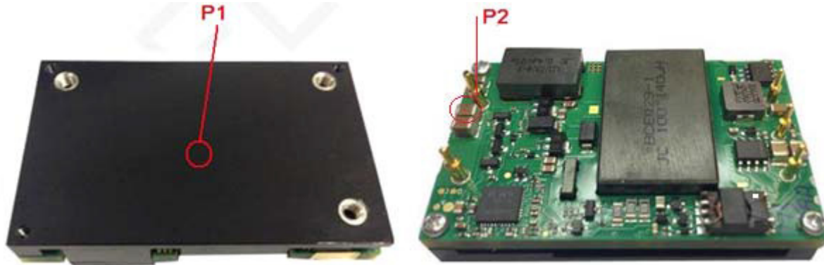
Figure 24 Temperature test point
