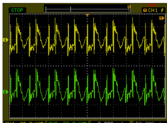
Figure 110: AXA00CC36-L Ripple and Noise Measurement Vin = 48Vdc Load: Io = \pm 0.67 A Ch 1: Vo
