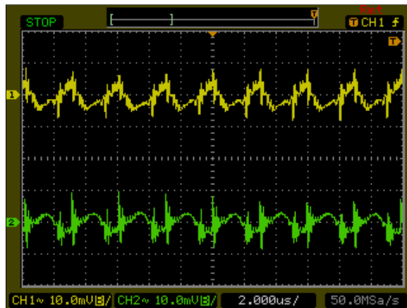
Figure 48: AXA00BB18-L Ripple and Noise Measurement Vin = 24Vdc Load: I_o = \pm 0.835 A Ch 1: Vo1 Ch2: Vo2
