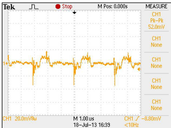
Figure 30: ERM02H72 Typical Output Ripple and Noise. Vin = 72Vdc Load: Io = 2.08A Ch 1: Vo
