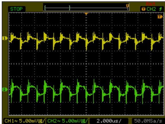
Figure 57: ATA00BB18-L Ripple and Noise Measurement Vin = 24Vdc, Load: Io = ±0.125A, Ta = 25 °C Ch 1: V1 Ch 2: V2
