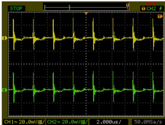
Figure 264: ATA00AA36S-L Ripple and Noise Measurement Vin = 48Vdc, Load: Io = ±0.3A, Ta = 25 °C Ch 1: V1 Ch 2: V2
