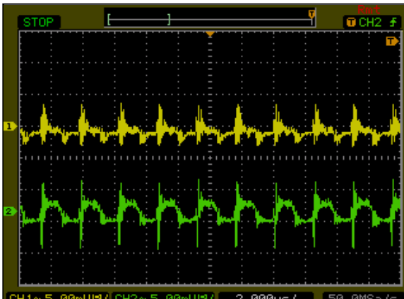
Figure 66: ATA00CC18-L Ripple and Noise Measurement Vin = 24Vdc, Load: Io = \pm 0.1 A, Ta = 25 °C Ch 1: V1 Ch 2: V2
