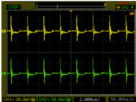
Figure 120: ATA00AA36-L Ripple and Noise Measurement Vin = 48Vdc, Load: Io = \pm 0.3A , Ta = 25 °C Ch 1: V1 Ch 2: V2
