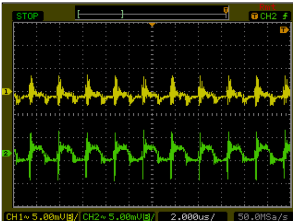
Figure 210: ATA00CC18S-L Ripple and Noise Measurement Vin = 24Vdc, Load: Io = ±0.1A, Ta = 25 °C Ch 1: V1 Ch 2: V2
