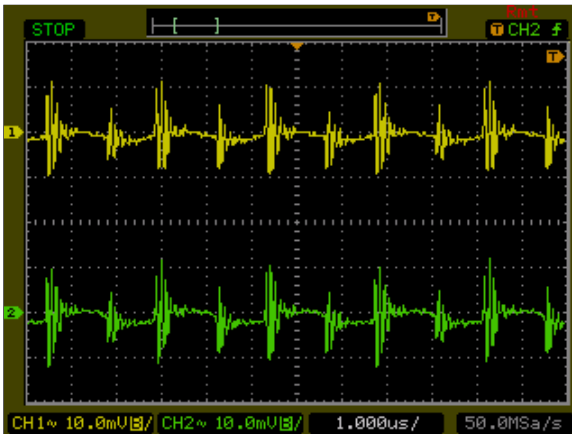
Figure 273: ATA00BB36S-L Ripple and Noise Measurement Vin = 48Vdc, Load: Io = \pm 0.125 A, Ta = 25 °C Ch 1: V1 Ch 2: V2
