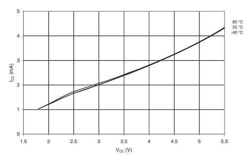
$\textbf{Figure 20-4.} \quad \text{Active Supply Current vs. } V_{\text{CC}} \text{ (Internal Calibrated Oscillator, 1 MHz)}$
