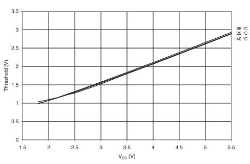
Figure 20-88.  $V_{IL}$ : Input Threshold Voltage vs.  $V_{CC}$  (I/O Pin, Read as '0')
