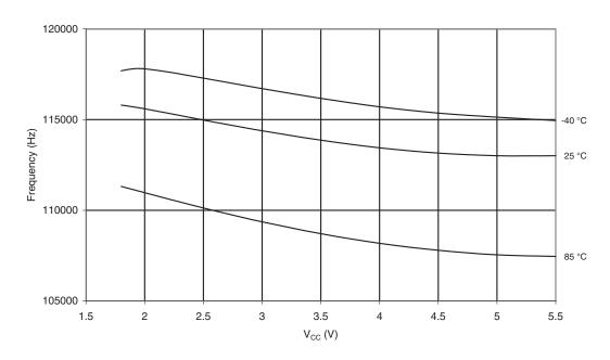
Figure 20-99. Frequency of Watchdog Oscillator vs. Temperature
