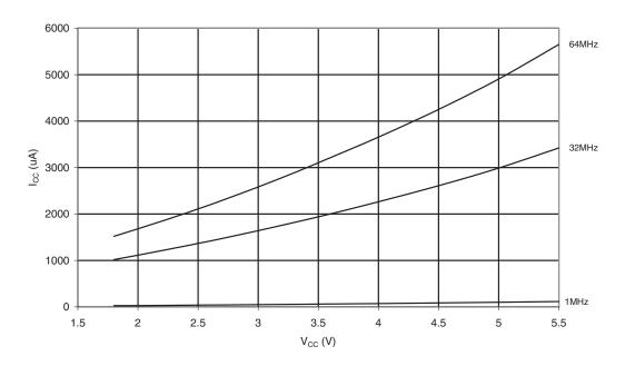
Figure 20-120. Brownout Detector Current vs.  $V_{\rm CC}$
