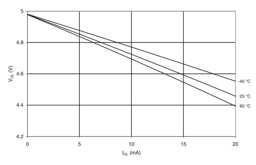
Figure 20-134.V<sub>OL</sub>: Output Voltage vs. Sink Current (Reset Pin as I/O, V<sub>CC</sub> = 5V)
