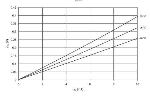
Figure 20-79.  $V_{OL}$ : Output Voltage vs. Sink Current (I/O Pin,  $V_{CC}$  = 5V)
