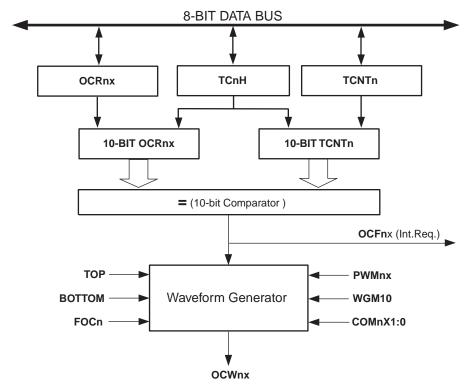
The OCR1x Registers are double buffered when using any of the Pulse Width Modulation (PWM) modes. For the normal mode of operation, the double buffering is disabled. The double buffering synchronizes the update of the OCR1x Compare Registers to either top or bottom of the counting sequence. The synchronization prevents the occurrence of odd-length, non-sym-
