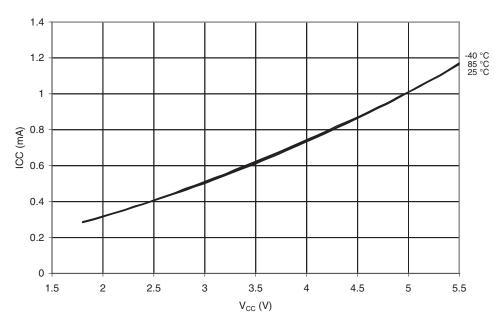
Figure 20-111.Idle Supply Current vs.  $V_{CC}$  (Internal Calibrated Oscillator, 1 MHz)
