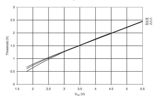
Figure 20-38.  $V_{IH}$ - $V_{IL}$ : Input Hysteresis vs.  $V_{CC}$  (I/O Pin)
