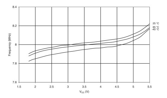
Figure 20-101. Frequency of Calibrated 8.0 MHz Oscillator vs. Temperature
