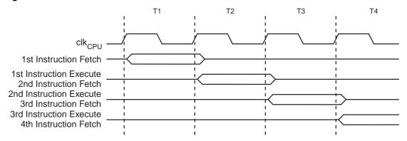
Figure 4-5 shows the internal timing concept for the Register File. In a single clock cycle an ALU operation using two register operands is executed, and the result is stored back to the destination register.
