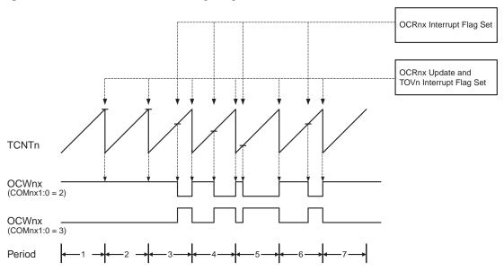
The Timer/Counter Overflow Flag (TOV1) is set each time the counter reaches TOP. If the interrupt is enabled, the interrupt handler routine can be used for updating the compare value.
