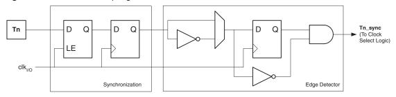
The synchronization and edge detector logic introduces a delay of 2.5 to 3.5 system clock cycles from an edge has been applied to the T0 pin to the counter is updated.
