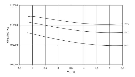
Figure 20-150. Frequency of Watchdog Oscillator vs. Temperature
