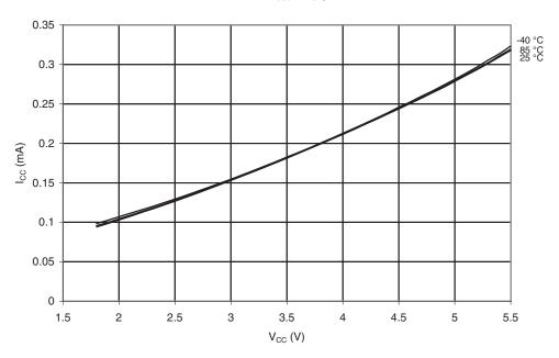
$\textbf{Figure 20-112.} \\ \textbf{Idle Supply Current vs. } \\ \textbf{V}_{\text{CC}} \text{ (Internal Calibrated Oscillator, 128 kHz)} \\$
