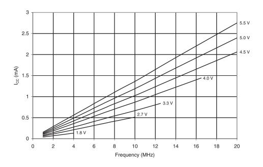
Figure 20-59. Idle Supply Current vs.  $V_{CC}$  (Internal Calibrated Oscillator, 8 MHz)
