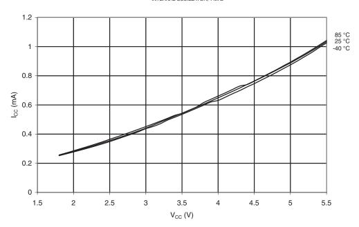
Figure 20-56. Active Supply Current vs.  $V_{CC}$  (Internal Calibrated Oscillator, 128 kHz)
