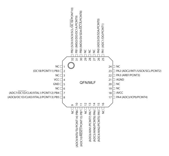
Note: To ensure mechanical stability the center pad underneath the QFN/MLF package should be soldered to ground on the board.
