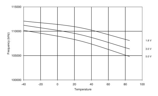
Figure 20-151. Frequency of Calibrated 8.0 MHz Oscillator vs.  $V_{CC}$
