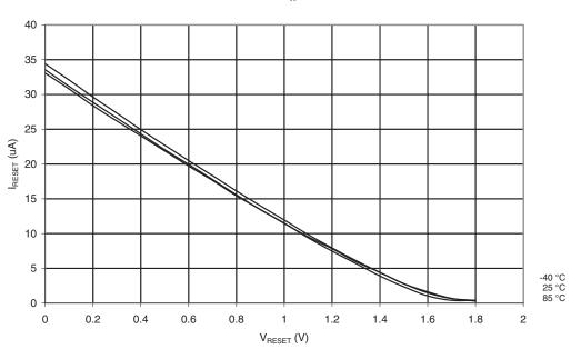
Figure 20-126. Pull-Up Resistor Current vs. Input Voltage (Reset Pin,  $V_{CC} = 3V$ )
