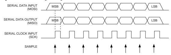
Figure 19-4. Serial Programming Timing
