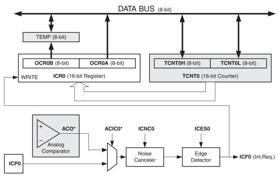
Figure 11-4. Input Capture Unit Block Diagram
