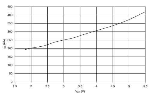
Figure 20-17. Timer/Counter1 Current vs. V<sub>CC</sub>
