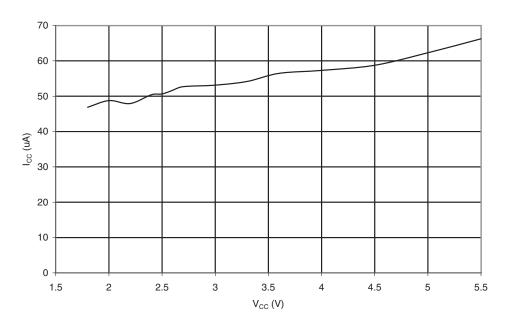
Figure 20-67. ADC Current vs.  $V_{CC}$  (AREF =  $AV_{CC}$ )
