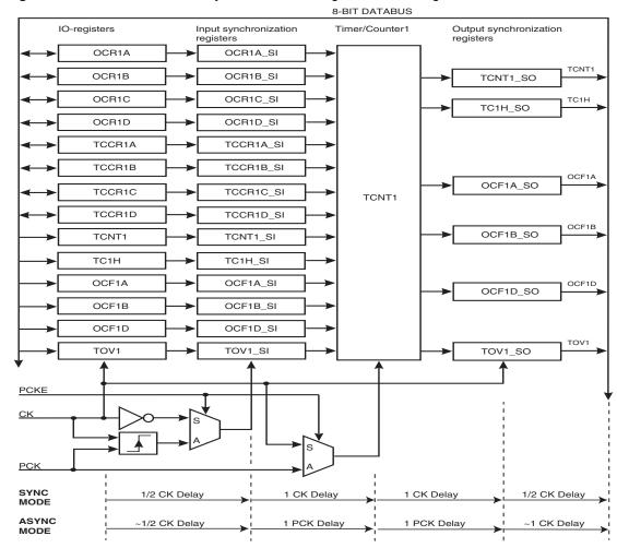
Figure 12-2. Timer/Counter1 Synchronization Register Block Diagram.
