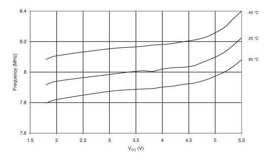
Figure 20-152. Frequency of Calibrated 8.0 MHz Oscillator vs. Temperature
