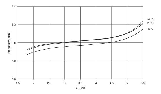
Figure 20-50. Frequency of Calibrated 8.0 MHz Oscillator vs. Temperature
