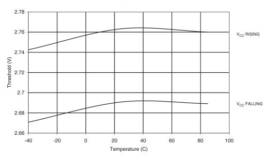
Figure 20-146.BOD Threshold vs. Temperature (BOD Level set to 1.8V)
