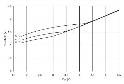
Figure 20-40.  $V_{\rm IL}$ : Input Threshold Voltage vs.  $V_{\rm CC}$  (Reset Pin, Read as '0')
