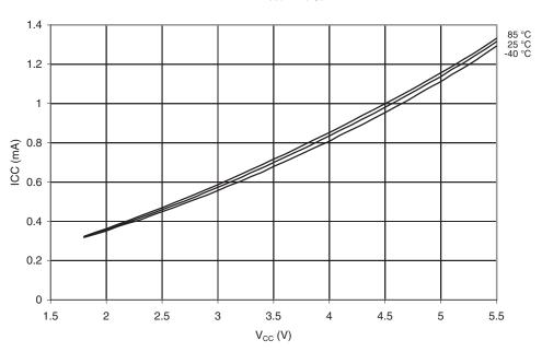
Figure 20-60. Idle Supply Current vs.  $V_{\text{CC}}$  (Internal Calibrated Oscillator, 1 MHz)
