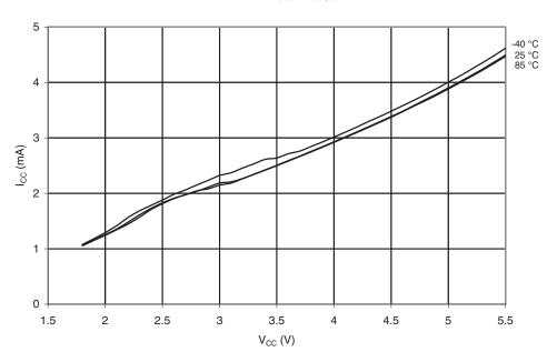
Figure 20-106. Active Supply Current vs. V<sub>CC</sub> (Internal Calibrated Oscillator, 1 MHz)
