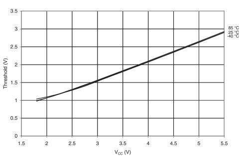
Figure 20-139. $V_{IL}$ : Input Threshold Voltage vs.  $V_{CC}$  (I/O Pin, Read as '0')
