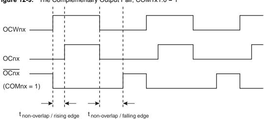
Figure 12-9. The Complementary Output Pair, COM1x1:0 = 1
