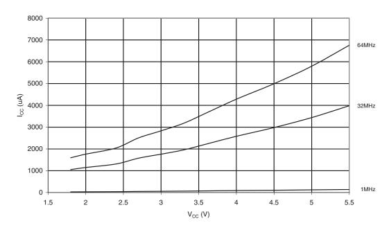
Figure 20-18. Brownout Detector Current vs.  $V_{\text{CC}}$
