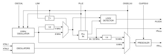
The internal PLL is enabled when CKSEL fuse bits are programmed to '0001' and the PLLE bit of PLLCSR is set. The internal oscillator and the PLL are switched off in power down and stand-by sleep modes.
