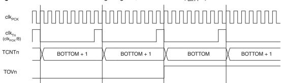
Figure 12-18. Timer/Counter Timing Diagram, with Prescaler (f<sub>clkT1</sub>/8)
