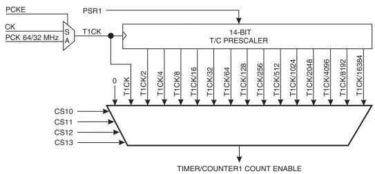
In the asynchronous clocking mode the clock selections are from PCK to PCK/16384 and stop, and in the synchronous clocking mode the clock selections are from CK to CK/16384 and stop. The clock options are illustrated in Figure 12-3 and desribed in "TCCR1B – Timer/Counter1 Control Register B" on page 113.
