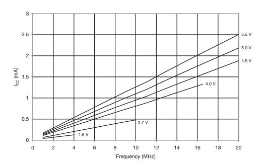
$\textbf{Figure 20-8.} \quad \text{Idle Supply Current vs. } V_{\text{CC}} \text{ (Internal Calibrated Oscillator, 8 MHz)}$
