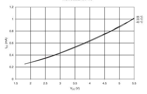
Figure 20-5. Active Supply Current vs.  $V_{CC}$  (Internal Calibrated Oscillator, 128 kHz)
