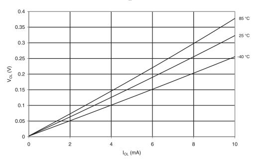
Figure 20-130.V<sub>OL</sub>: Output Voltage vs. Sink Current (I/O Pin, V<sub>CC</sub> = 5V)
