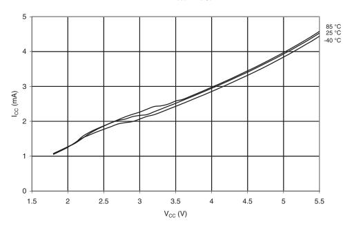
$\textbf{Figure 20-55.} \ \, \textbf{Active Supply Current vs.} \ \, \textbf{V}_{\text{CC}} \, (\textbf{Internal Calibrated Oscillator}, \, 1 \, \text{MHz})$
