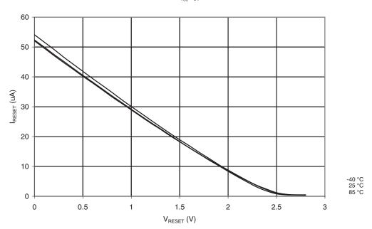
Figure 20-127. Pull-Up Resistor Current vs. Input Voltage (Reset Pin,  $V_{CC} = 5V$ )
