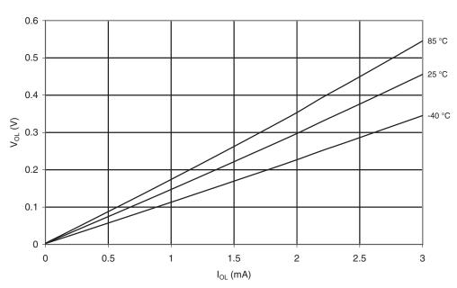
Figure 20-135.V<sub>OL</sub>: Output Voltage vs. Sink Current (Reset Pin as I/O, T = 25°C)
