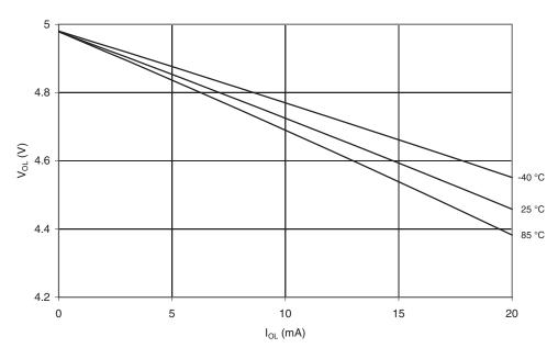
Figure 20-83.  $V_{OL}$ : Output Voltage vs. Sink Current (Reset Pin as I/O,  $V_{CC}$  = 5V)
