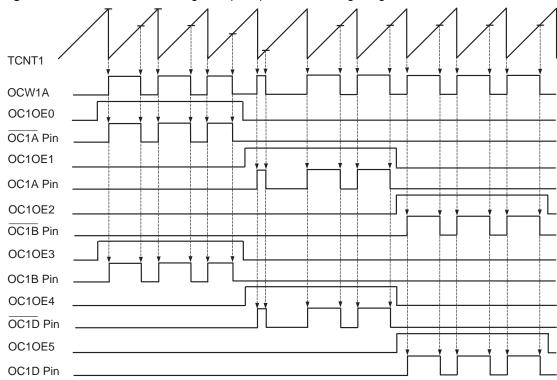
Figure 12-14. PWM6 Mode, Single-slope Operation, Timing Diagram
