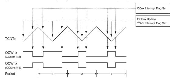
Figure 12-13. Phase and Frequency Correct PWM Mode, Timing Diagram
