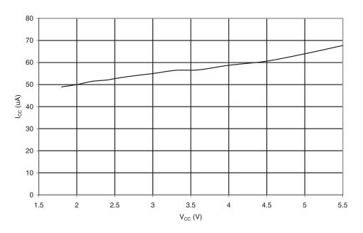
Figure 20-118.ADC Current vs.  $V_{CC}$  (AREF =  $AV_{CC}$ )
