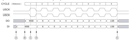
Figure 13-3. Three-wire Mode, Timing Diagram
