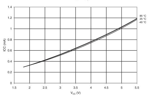
Figure 20-9. Idle Supply Current vs.  $V_{\text{CC}}$  (Internal Calibrated Oscillator, 1 MHz)
