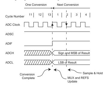
Figure 15-7. ADC Timing Diagram, Free Running Conversion
