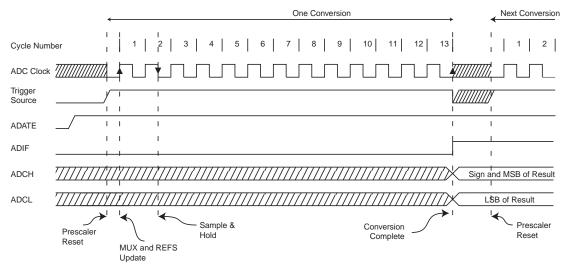
Figure 15-6. ADC Timing Diagram, Auto Triggered Conversion
