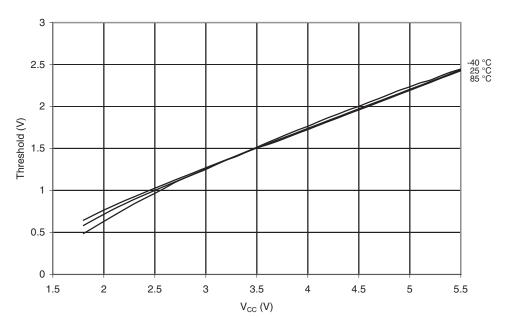
Figure 20-140.V $_{\rm IH}$ -V $_{\rm IL}$ : Input Hysteresis vs. V $_{\rm CC}$  (I/O Pin)
