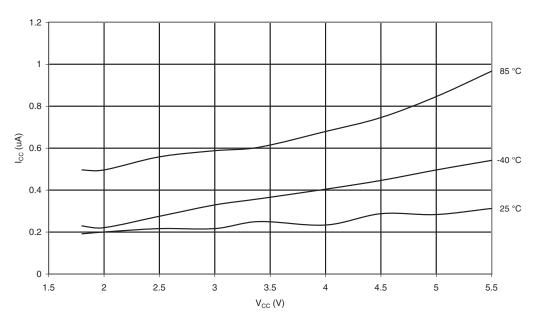
Figure 20-63. Power-down Supply Current vs.  $V_{CC}$  (Watchdog Timer Enabled)
