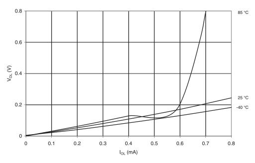
Figure 20-33.  $V_{OL}$ : Output Voltage vs. Sink Current (Reset Pin as I/O, T = 25°C)
