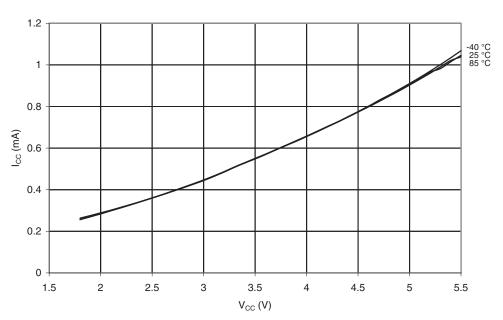
Figure 20-107. Active Supply Current vs.  $V_{CC}$  (Internal Calibrated Oscillator, 128 kHz)
