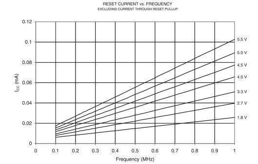
Figure 20-116.Reset Supply Current vs. Frequency (1 - 20 MHz, Excluding Current Through the Reset Pull-up)
