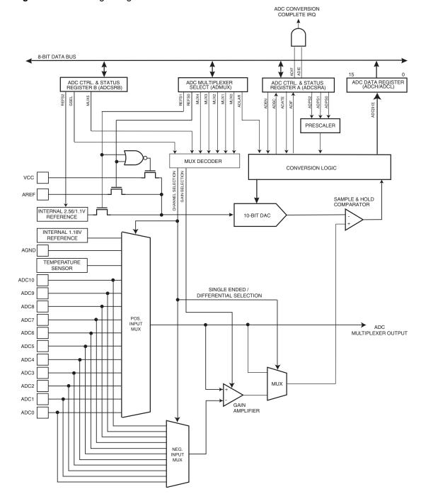
Figure 15-1. Analog to Digital Converter Block Schematic
