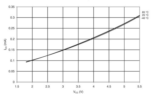
Figure 20-10. Idle Supply Current vs. V<sub>CC</sub> (Internal Calibrated Oscillator, 128 kHz)
