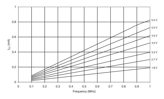
Figure 20-104. Active Supply Current vs. Frequency (1 - 20 MHz)
