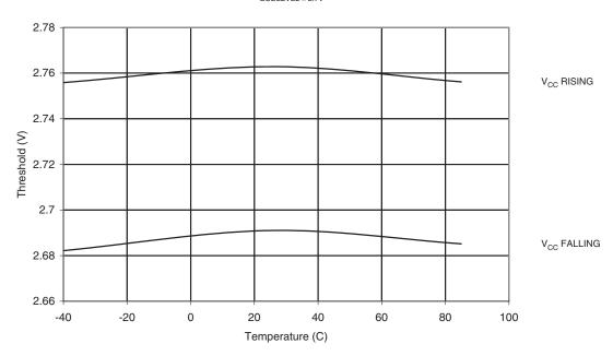
Figure 20-44. BOD Threshold vs. Temperature (BOD Level set to 1.8V)
