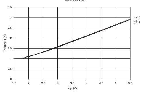
Figure 20-37.  $V_{IL}$ : Input Threshold Voltage vs.  $V_{CC}$  (I/O Pin, Read as '0')
