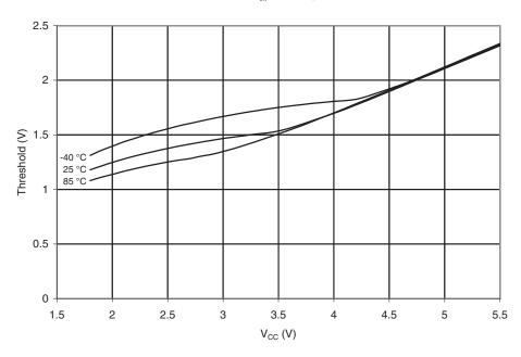
Figure 20-142.V $_{\rm IL}$ : Input Threshold Voltage vs. V $_{\rm CC}$  (Reset Pin, Read as '0') RESET INPUT THRESHOLD VOLTAGE vs. VCC  $_{\rm V}_{\rm IL}$ , PIN READ AS '0'
