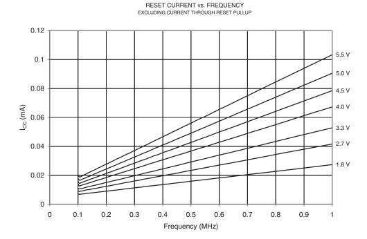
**Figure 20-14.** Reset Supply Current vs. Frequency (1 - 20 MHz, Excluding Current Through the Reset Pull-up)
