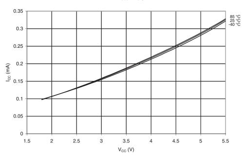
Figure 20-61. Idle Supply Current vs. V<sub>CC</sub> (Internal Calibrated Oscillator, 128 kHz)
