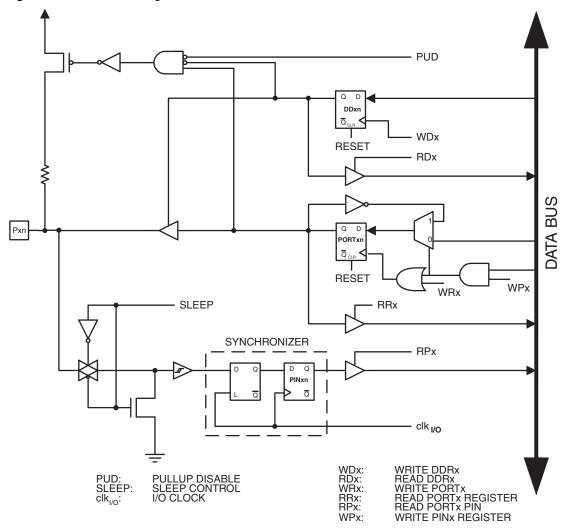
Note: 1. WRx, WPx, WDx, RRx, RPx, and RDx are common to all pins within the same port. clk<sub>I/O</sub>, SLEEP, and PUD are common to all ports.
