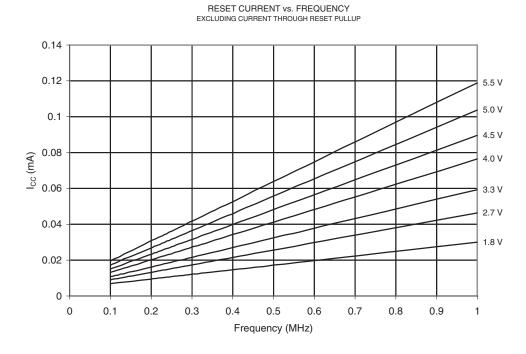
**Figure 20-65.** Reset Supply Current vs. Frequency (1 - 20 MHz, Excluding Current Through the Reset Pull-up)
