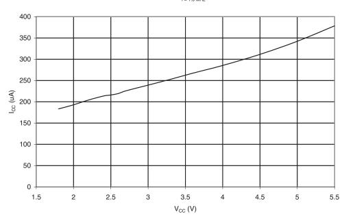
Figure 20-119.Timer/Counter1 Current vs. V<sub>CC</sub>
