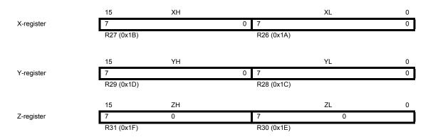
In different addressing modes these address registers function as automatic increment and automatic decrement (see the instruction set reference for details).
