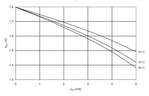
Figure 20-30. V<sub>OH</sub>: Output Voltage vs. Source Current (I/O Pin, V<sub>CC</sub> = 3V)
