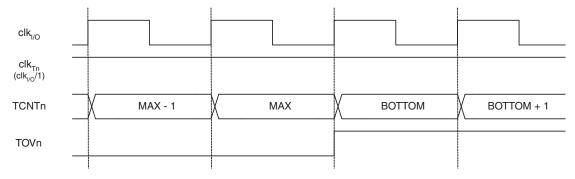
Figure 11-8 shows the same timing data, but with the prescaler enabled.
