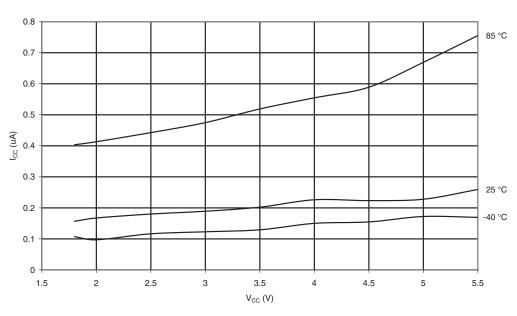
Figure 20-114. Power-down Supply Current vs.  $V_{CC}$  (Watchdog Timer Enabled)
