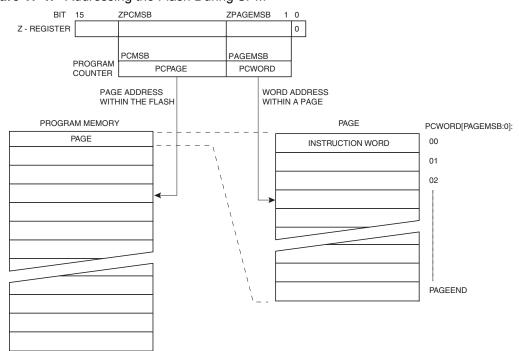
Figure 17-1. Addressing the Flash During SPM
