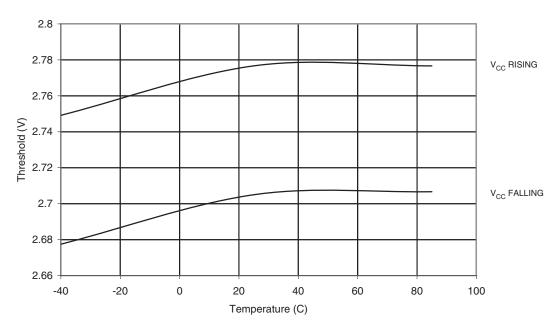
Figure 20-95. BOD Threshold vs. Temperature (BOD Level set to 1.8V)
