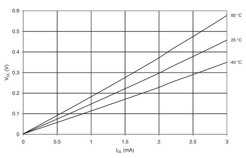
Figure 20-84.  $V_{OL}$ : Output Voltage vs. Sink Current (Reset Pin as I/O, T = 25°C)
