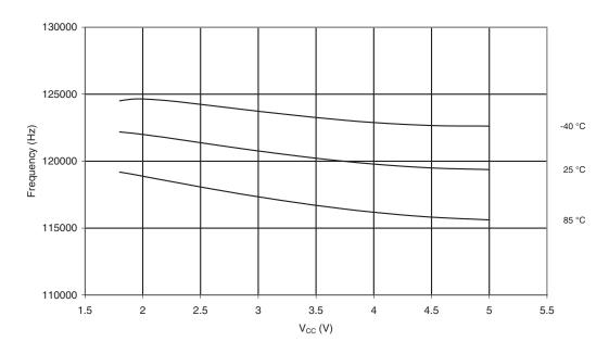
Figure 20-48. Frequency of Watchdog Oscillator vs. Temperature
