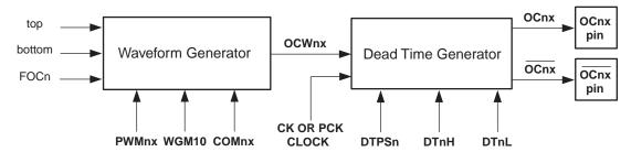
The tasks are shared as follows: the Waveform Generator generates the output (OCW1x) and the Dead Time Generator generates the non-overlapping PWM output pair from the output. Three Dead Time Generators are provided, one for each PWM output. The non-overlap time is adjustable and the PWM output and it's complementary output are adjusted separately, and independently for both PWM outputs.
