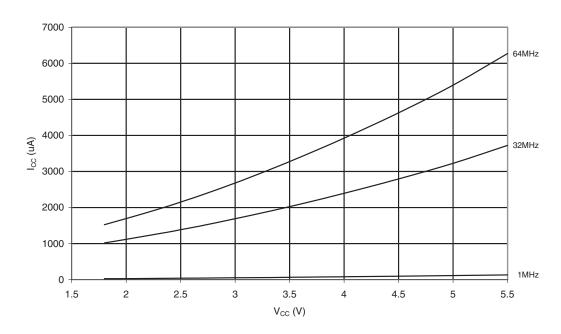
Figure 20-69. Brownout Detector Current vs.  $V_{\text{CC}}$
