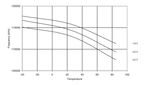
Figure 20-100. Frequency of Calibrated 8.0 MHz Oscillator vs.  $V_{CC}$
