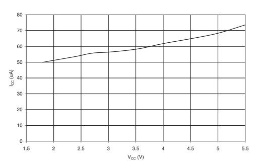
Figure 20-16. ADC Current vs.  $V_{CC}$  (AREF =  $AV_{CC}$ )
