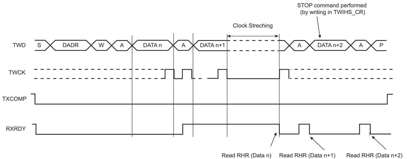
RXRDY is used as receive ready for the DMA receive channel.
