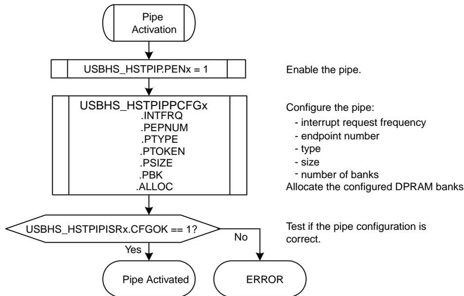
As long as the pipe is not correctly configured ( $\text{USBHS\_HSTPIISRx.CFGOK} = 0$ ), the controller cannot send packets to the device through this pipe.
