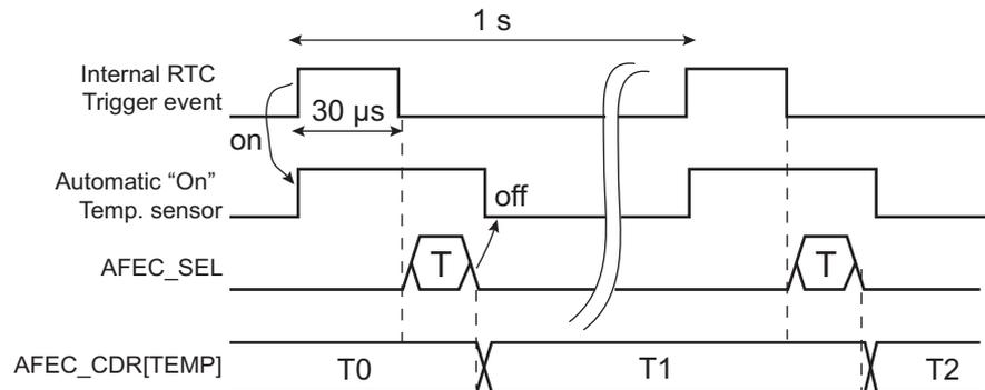
Moreover, it is possible to raise a flag only if there is predefined change in the temperature measurement. The user can define a range of temperature or a threshold in AFEC\_TEMPCLR and the mode of comparison in AFEC\_TEMPMPR. These values define the way the TEMPCHG flag will be raised in AFEC\_ISR.
