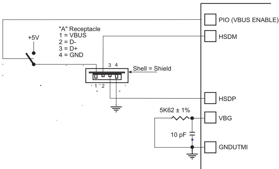
2. The schematic below shows a typical USB High Speed device connection: For more information, refer to [Section 37. "USB High-Speed Interface \(USBHS\)"](#).
