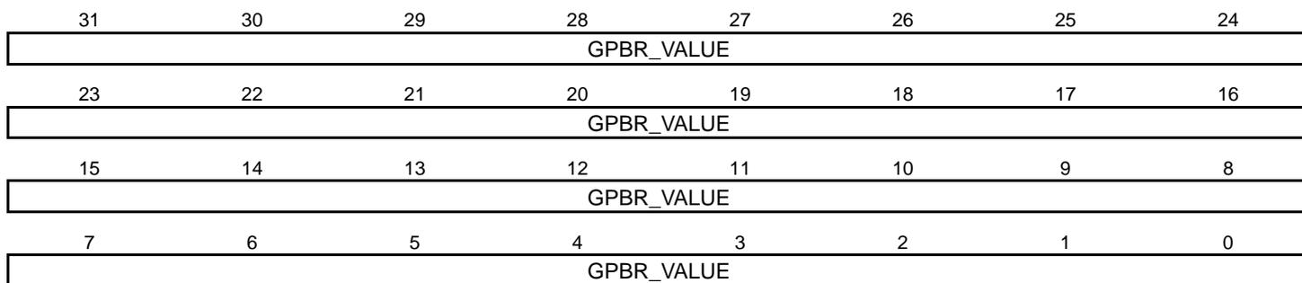
These registers are reset at first power-up and on each loss of VDDIO.
