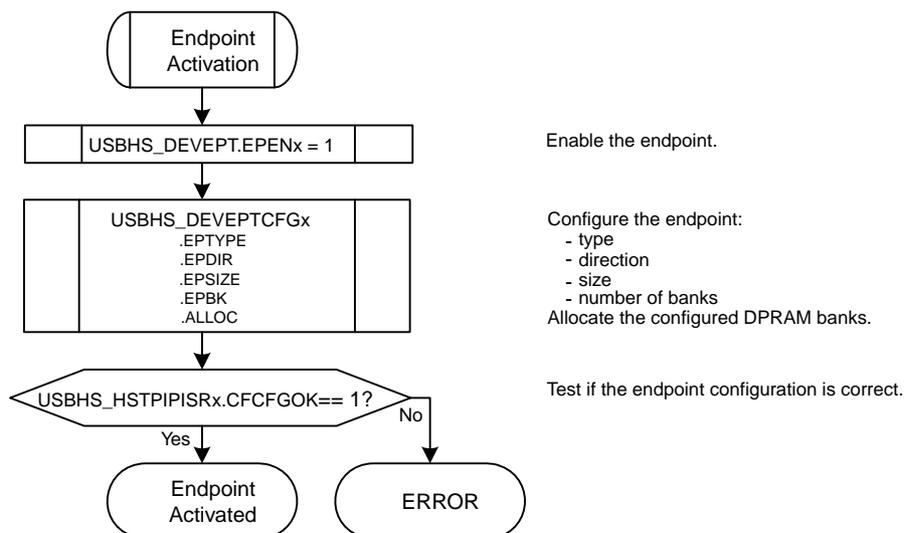
As long as the endpoint is not correctly configured (USBHS\_HSTPIISRx.CFGOK = 0), the controller does not acknowledge the packets sent by the host to this endpoint.
