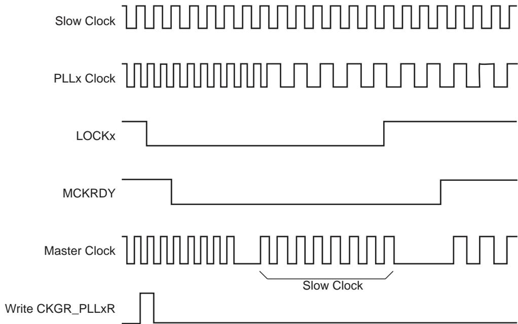
**Figure 31-9. Programmable Clock Output Programming**
