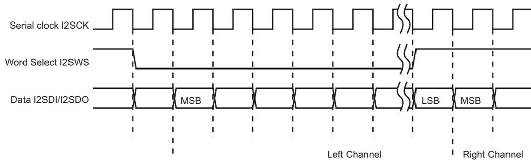
Data bits are sent on the falling edge of the serial clock and sampled on the rising edge of the serial clock. The word select line indicates the channel in transmission, a low level for the left channel and a high level for the right channel.
