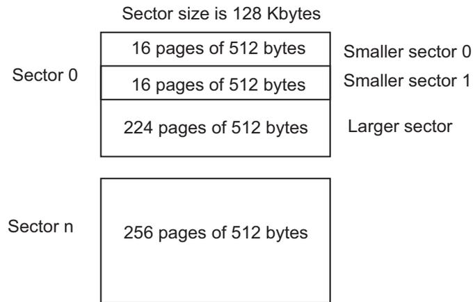
[Figure 10-3](#) illustrates the organization of the Flash depending on its size.
