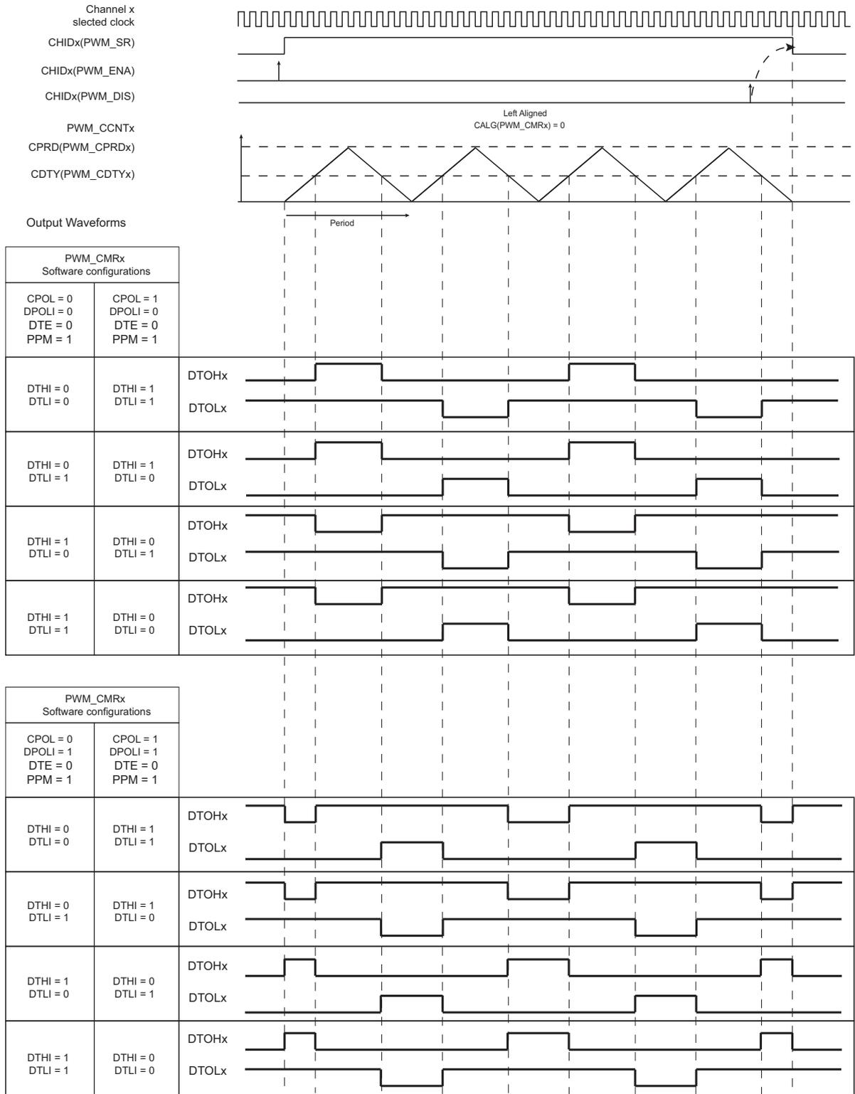
The PWM Push-Pull mode can be useful in transformer-based power converters, such as a half-bridge converter. The Push-Pull mode prevents the transformer core from being saturated by any direct current.
