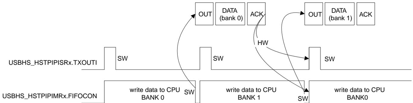
**Figure 37-23. Example of an OUT Pipe with two Data Banks and a Bank Switching Delay**
