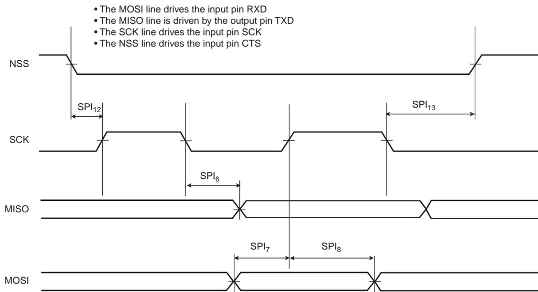
Figure 56-28. USART SPI Slave Mode (Mode 0 or 3)
