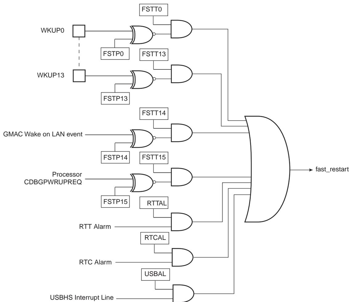
Each wake-up input pin and alarm can be enabled to generate a fast startup event by setting the corresponding bit in PMC\_FSMR.
