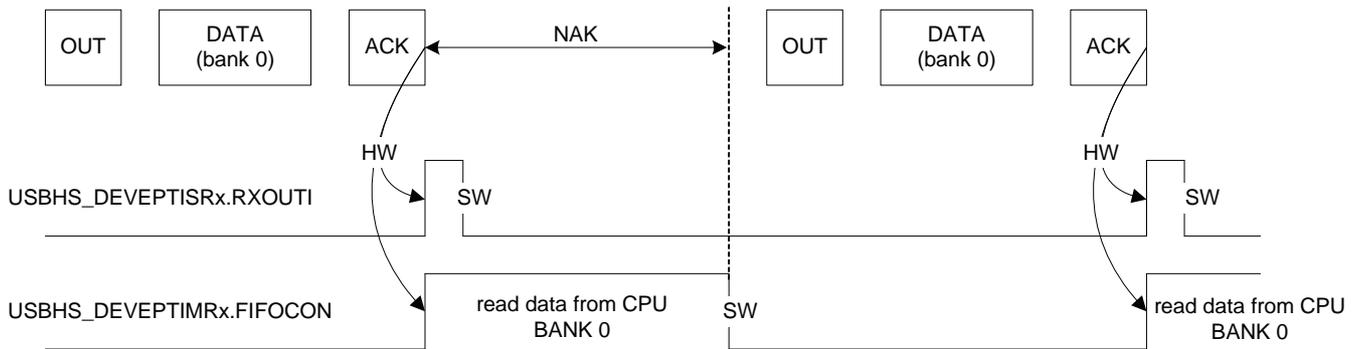
**Figure 37-15. Example of an OUT Endpoint with two Data Banks**
