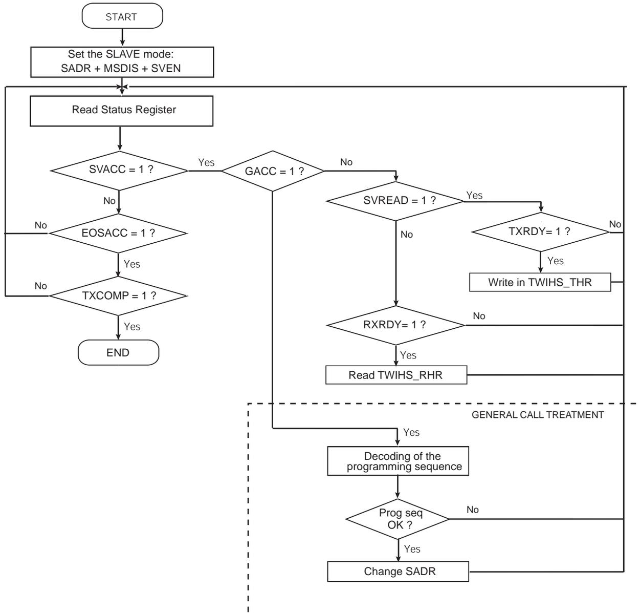
Figure 42-44. Read Write Flowchart in Slave Mode with SMBus PEC
