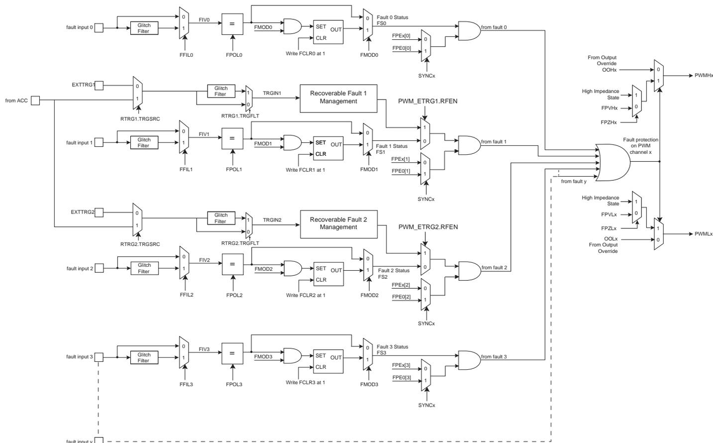
The polarity level of the fault inputs is configured by the FPOL field in the [PWM Fault Mode Register \(PWM\\_FMR\)](#). For fault inputs coming from internal peripherals such as ADC or Timer Counter, the polarity level must be FPOL = 1. For fault inputs coming from external GPIO pins the polarity level depends on the user's implementation.
