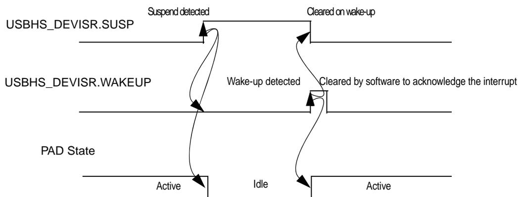
The USBHS\_DEVISR.SUSP bit is set and the Wake-Up Interrupt (USBHS\_DEVISR.WAKEUP) bit is cleared when a USB “Suspend” state has been detected on the USB bus. This event automatically puts the USB pad in Idle state. The detection of a non-idle event sets USBHS\_DEVISR.WAKEUP, clears USBHS\_DEVISR.SUSP and wakes up the USB pad.
