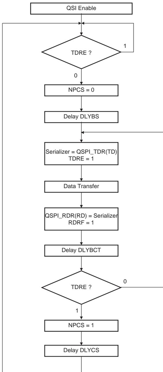
Figure 41-7 shows Transmit Data Register Empty (TDRE), Receive Data Register Full (RDRF) and Transmission Register Empty (TXEMPTY) status flags behavior within the QSPI\_SR during an 8-bit data transfer in Fixed mode, without DMA.
