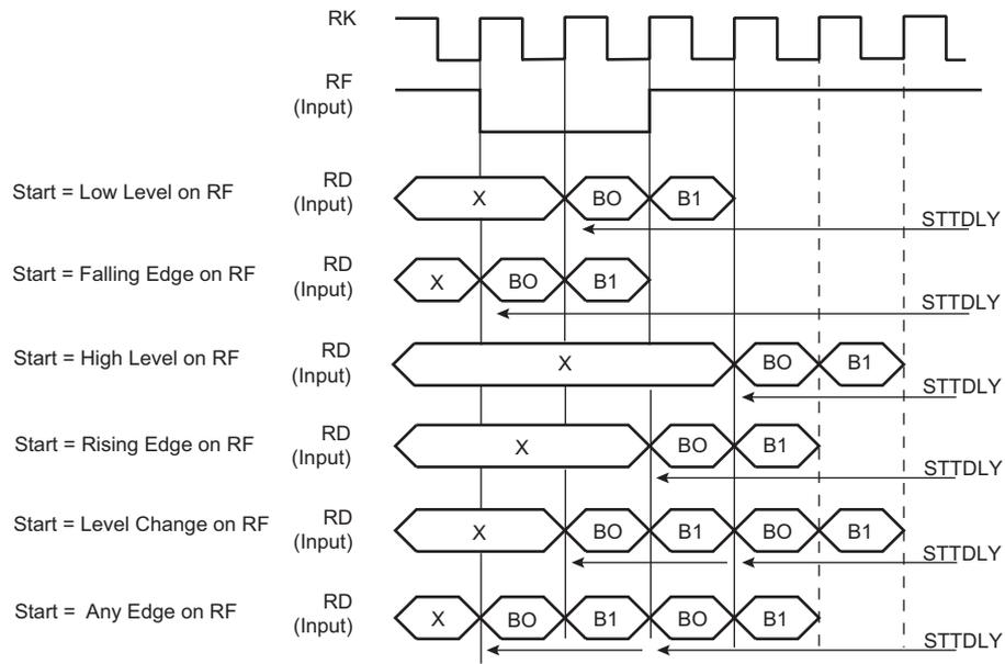
transfer either by writing a new Compare 0, or by receiving continuously until Compare 1 occurs. This selection is done with the STOP bit in the SSC\_RCMR.
