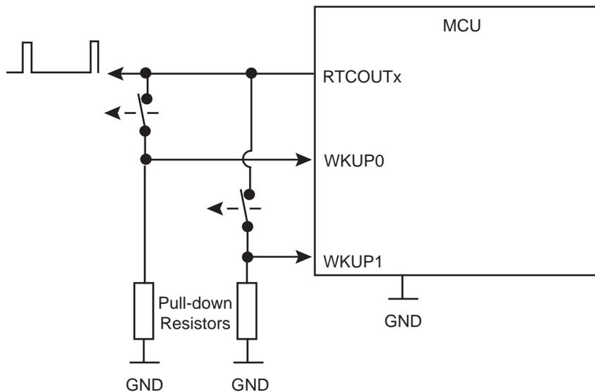
The debouncing period duration is configurable. The period is set for all debouncers (i.e., the duration cannot be adjusted for each debouncer). The number of successive identical samples to wake up the system can be configured from 2 up to 8 in the LPDBC field of SUPC\_WUMR. The period of time between two samples can be configured by programming the TPERIOD field in the RTC\_MR. Power parameters can be adjusted by modifying the period of time in the THIGH field in RTC\_MR.
