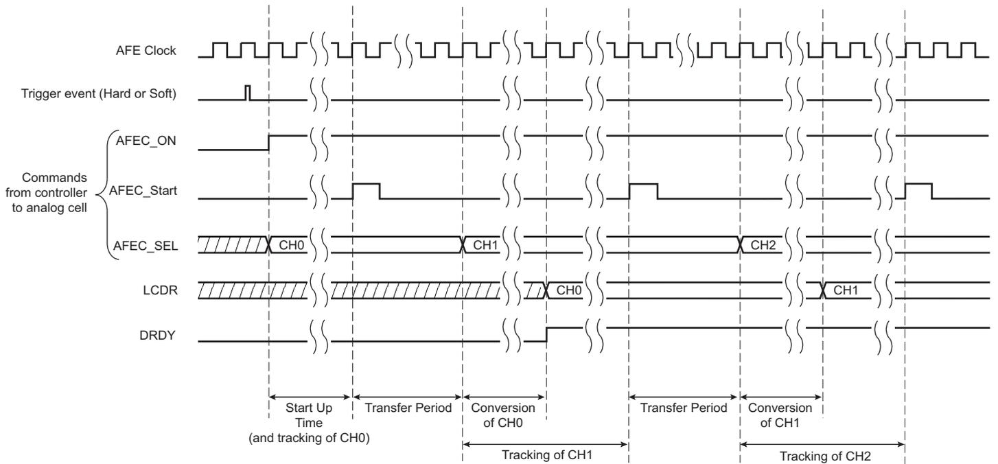
**Figure 50-3. Sequence of AFE Conversions when Tracking Time < Conversion Time**
