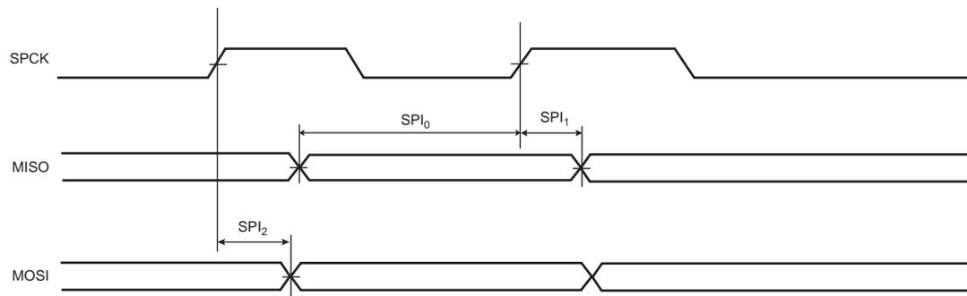
**Figure 56-21. SPI Master Mode with (CPOL = 0 and NCPHA=1) or (CPOL=1 and NCPHA= 0)**
