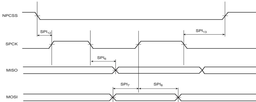
**Figure 56-23. SPI Slave Mode with (CPOL = NCPHA = 0) or (CPOL= NCPHA= 1)**
