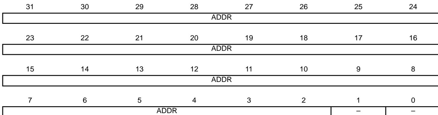
This register holds the start address of the transmit buffer queue (transmit buffers descriptor list). The Transmit Buffer Queue Base Address Register must be initialized before transmit is started through bit 9 of the Network Control Register. Once transmission has started, any write to the Transmit Buffer Queue Base Address Register is illegal and therefore ignored.
