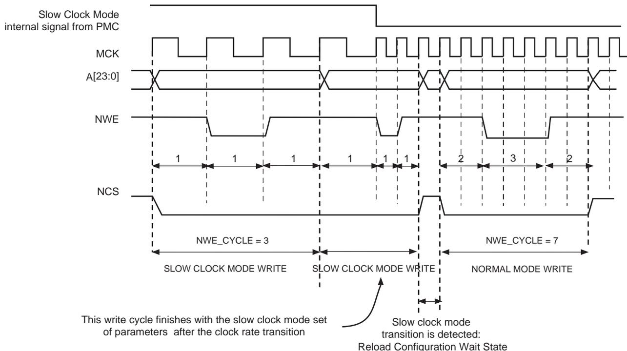
**Figure 34-32. Recommended Procedure to Switch from Slow Clock Mode to Normal Mode or from Normal Mode to Slow Clock Mode**
