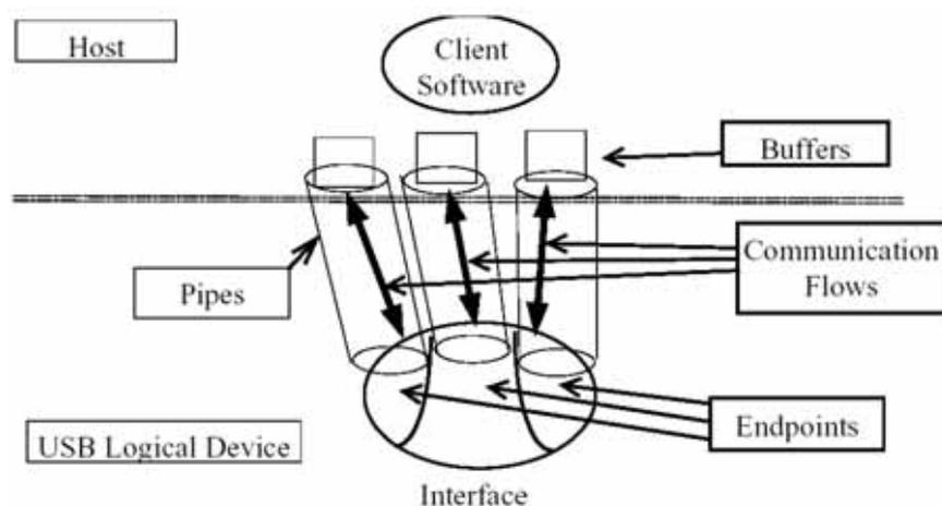
In Host mode, the USBHS associates a pipe to a device endpoint, considering the device configuration descriptors.
