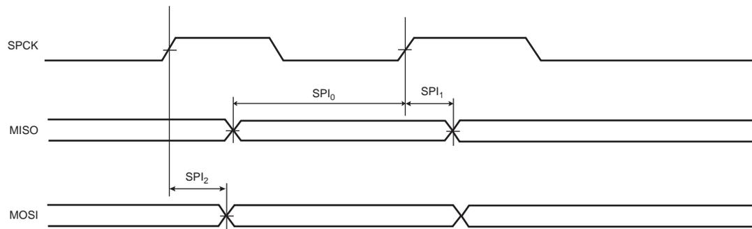
**Figure 56-47. SPI Master Mode with (CPOL = 0 and NCPHA=1) or (CPOL=1 and NCPHA= 0)**
