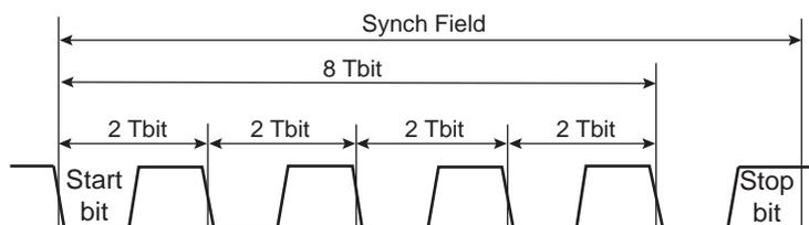
The time measurement is made by a 19-bit counter clocked by the sampling clock (see [Section 45.6.1 "Baud Rate Generator"](#)).
