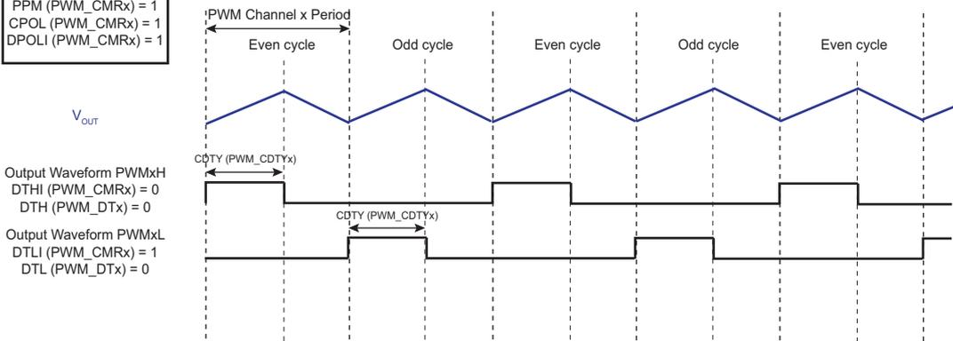
Figure 49-14. Half-Bridge Converter Application: Feedback Regulation
