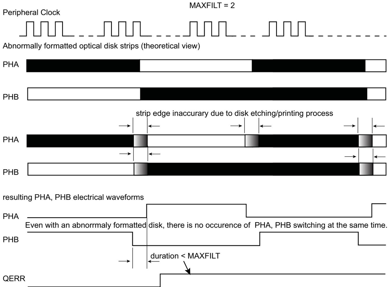
MAXFILT must be tuned according to several factors such as the peripheral clock frequency, type of rotary sensor and rotation speed to be achieved.
