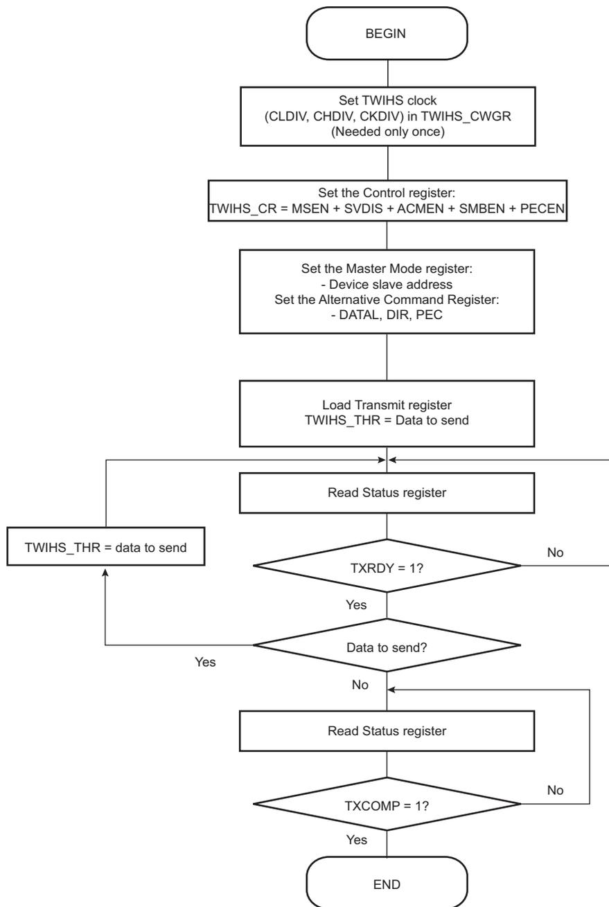
Figure 42-19. TWIHS Write Operation with Multiple Data Bytes and Read Operation with Multiple Data Bytes (Sr)
