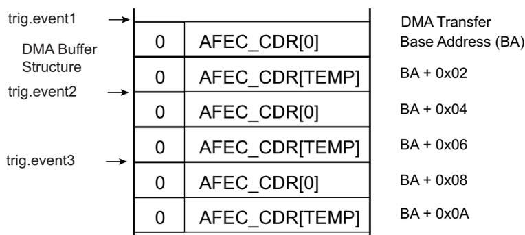
The temperature factor has a slow variation rate and may be different from other conversion channels. As a result, the AFEC allows a different way of triggering temperature measurement when the bit RTCT is set in the AFEC\_TEMP\_MR but the CH11 is cleared in the AFEC\_CHSR.
