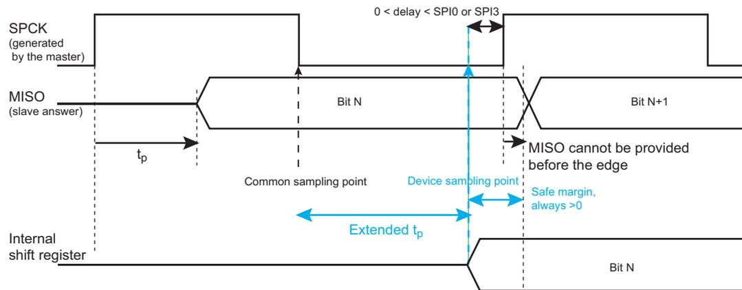
**Figure 56-20. SPI Master Mode with (CPOL= NCPHA = 0) or (CPOL= NCPHA= 1)**
