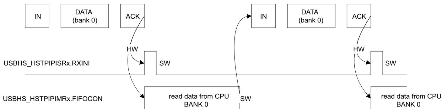
**Figure 37-20. Example of an IN Pipe with two Data Banks**
