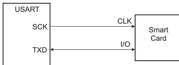
When operating in ISO7816, either in T = 0 or T = 1 modes, the character format is fixed. The configuration is 8 data bits, even parity and 1 or 2 stop bits, regardless of the values programmed in the CHRL, MODE9, PAR and CHMODE fields. MSBF can be used to transmit LSB or MSB first. Parity Bit (PAR) can be used to transmit in Normal or Inverse mode. Refer to Section 45.7.3 "USART Mode Register" and "PAR: Parity Type" .
