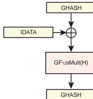
It is possible to process a message with only AAD setting the CLEN field to '0' in the AES\_CLENR, this can be used for  $J_0$  generation when  $\text{len}(IV) \neq 96$  for instance.
