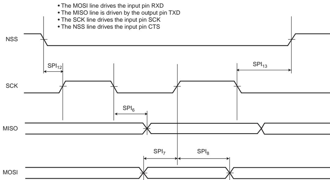
Figure 56-54. USART SPI Slave Mode (Mode 0 or 3)
