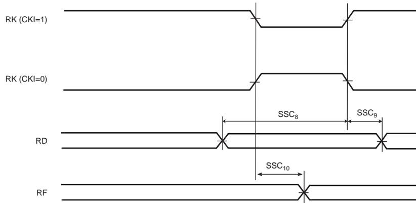
**Figure 56-39. SSC Receiver, RK and RF in Output**
