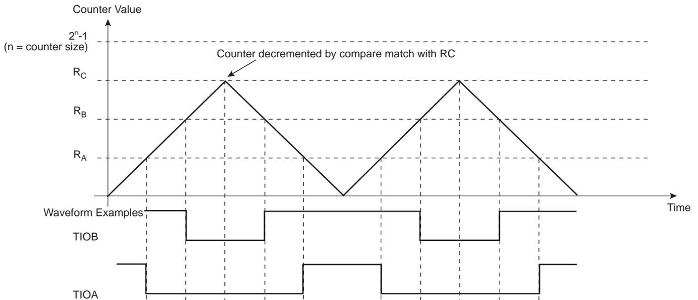
**Figure 48-15. WAVSEL = 11 with Trigger**
