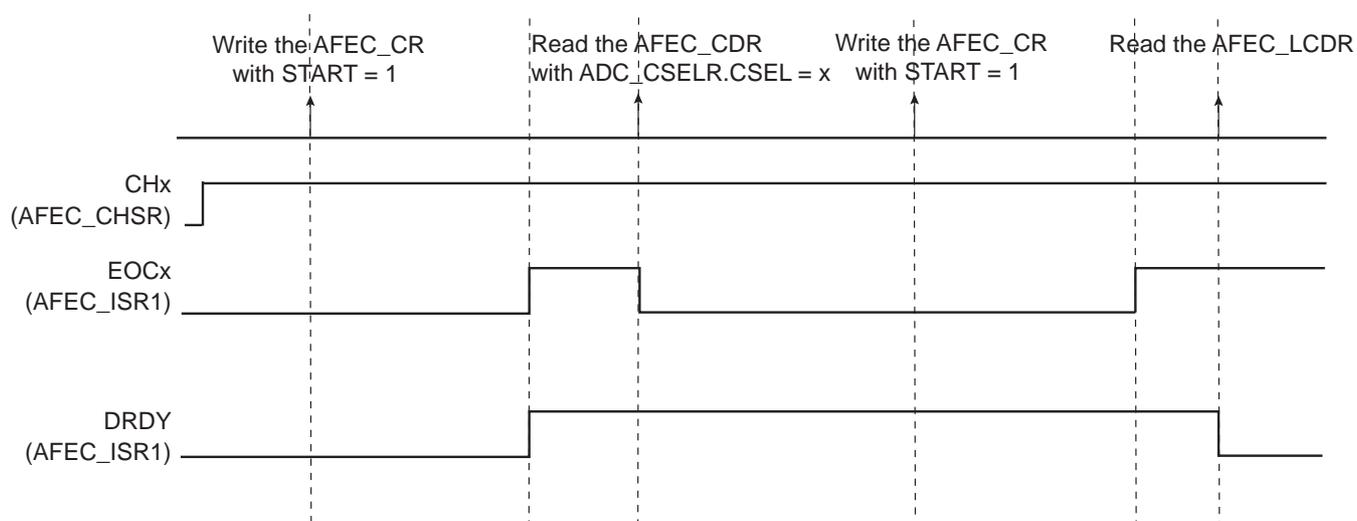
If AFEC\_CDR is not read before further incoming data is converted, the corresponding OVREx flag is set in the Overrun Status Register (AFEC\_OVER).
