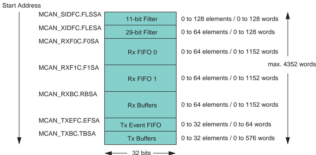
When the MCAN addresses the Message RAM, it addresses 32-bit words, not single bytes. The configurable start addresses are 32-bit word addresses; i.e., only bits 15 to 2 are evaluated, the two least significant bits are ignored.
