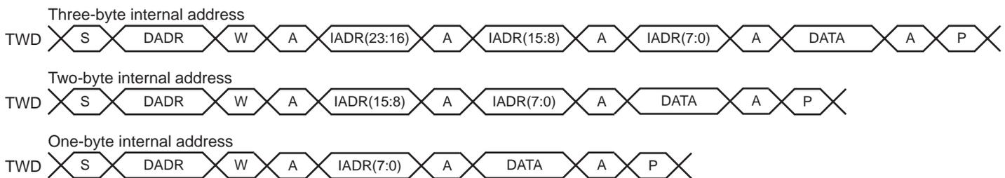
**Figure 42-11. Master Read with One-, Two- or Three-Byte Internal Address and One Data Byte**
