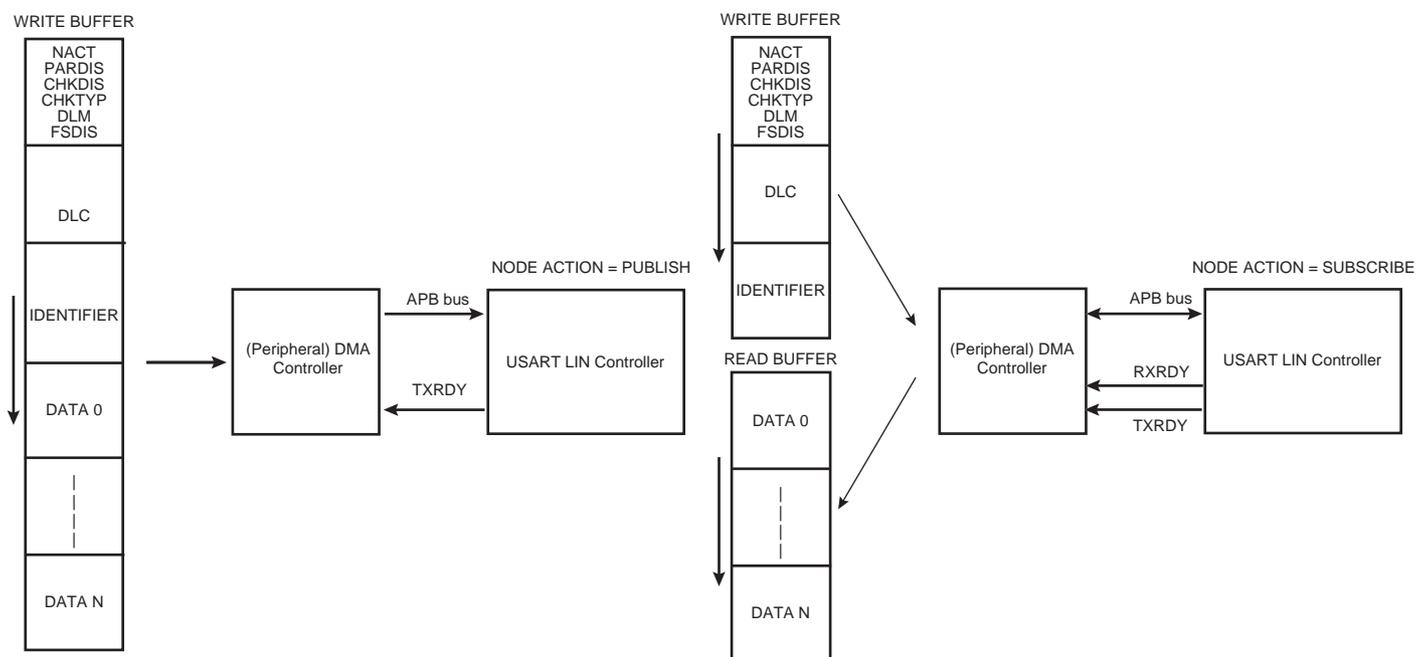
**Figure 45-52. Master Node with DMAC (PDCM = 0)**
