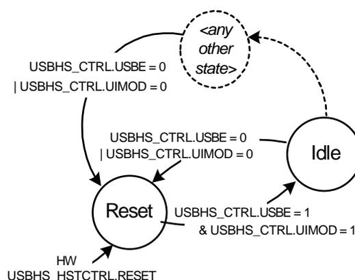
After a hardware reset, the USBHS Device mode is in Reset state. In this state:
