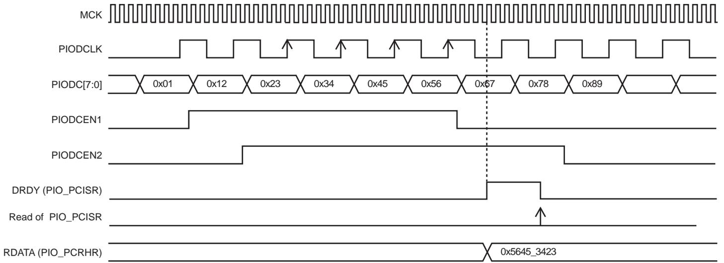
**Figure 32-10. Parallel Capture Mode Waveforms (DSIZE = 2, ALWAYS = 1, HALFS = 0)**
