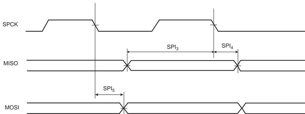
**Figure 56-22. SPI Slave Mode with (CPOL=0 and NCPHA=1) or (CPOL=1 and NCPHA=0)**
