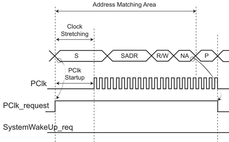
**Figure 42-41. Address Match and Data Match (Data Matching Enabled)**
