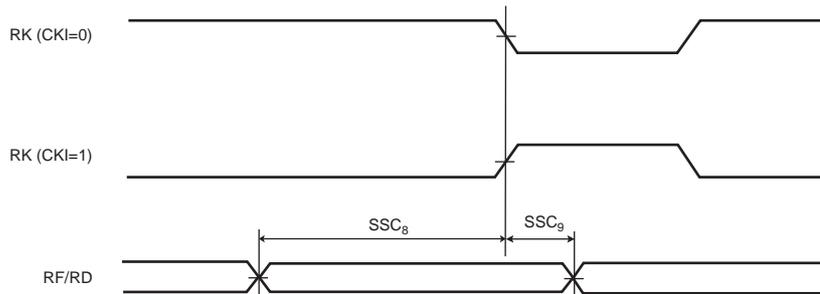
**Figure 56-38. SSC Receiver, RK in Input and RF in Output**
