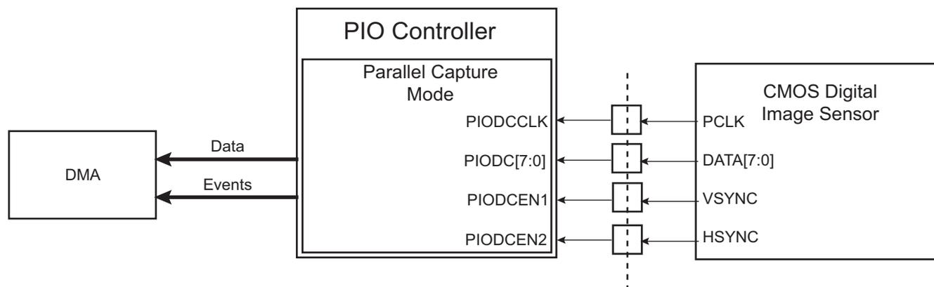
As soon as the parallel capture mode is enabled by writing a one to the PCEN bit in PIO\_PCMR, the I/O lines connected to the sensor clock (PIODCCLK), the sensor data (PIODC[7:0]) and the sensor data enable signals (PIODCEN1 and PIODCEN2) are configured automatically as inputs. To know which I/O lines are associated with the sensor clock, the sensor data and the sensor data enable signals, refer to the I/O multiplexing table(s) in [Section 5. "Package and Pinout"](#).
