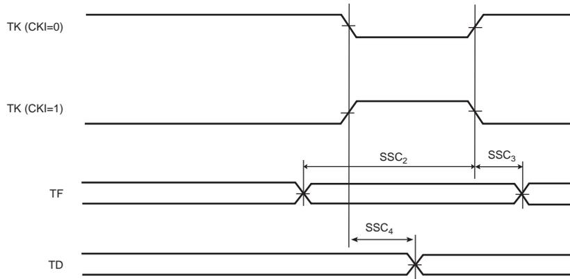
**Figure 56-62. SSC Transmitter, TK and TF in Input**
