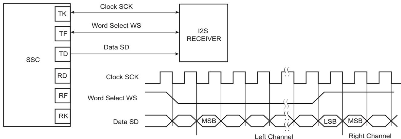
**Figure 43-4. Codec Application Block Diagram**
