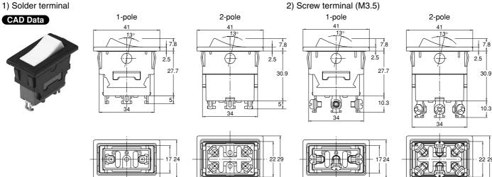
Remarks: 1. ON-OFF type does not have terminal No. 2 and 5. 2. Dimensions of actuator: 1-pole: 12.6  $\times$  29, 2-pole: 17.4  $\times$  29
