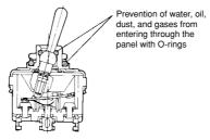
• Terminal-sealed type Both switch body and terminals have been sealed to protect from dust and gas that enters from the panel. (Panel front: IP67\*; Inside of panel: IP60)
