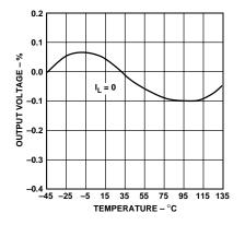
Figure 6. Output Voltage Variation % vs. Temperature
