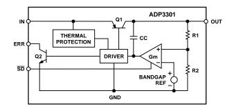
The ADP3301 operates with a wide input voltage range from 3 V to 12 V and delivers a load current in excess of 100 mA. It features an error flag that signals when the device is about to lose regulation or when the short circuit or thermal overload protection is activated. Other features include shutdown and optional noise reduction capabilities. The ADP330x anyCAP<sup>TM\*</sup> LDO family offers a wide range of output voltages and output current levels from 50 mA to 200 mA:
