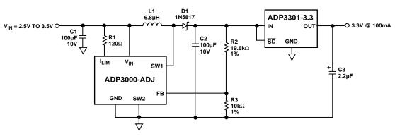
Figure 23. Step-Up/Step-Down Post Regulator
