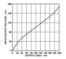
Figure 8. Dropout Voltage vs. Output Current
