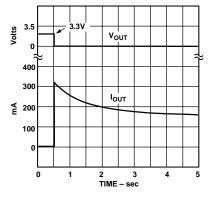
Figure 15. Short Circuit Current
