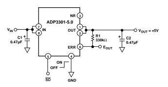
Figure 1. Typical Application Circuit
