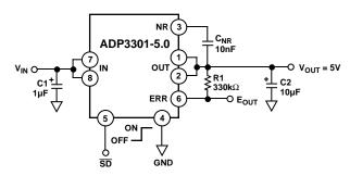
Figure 20. Noise Reduction Circuit
