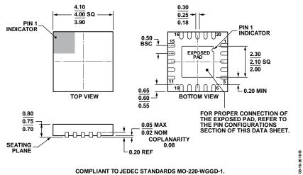
20-Lead Lead Frame Chip Scale Package [LFCSP\_WQ] 4 mm × 4 mm Body, Very Very Thin Quad (CP-20-6) Dimensions shown in millimeters
