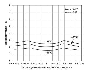
TPC 5. ON Resistance as a Function of  $V_D$  ( $V_S$ ) for Different Temperatures, Dual Supply
