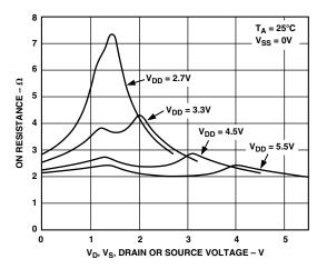
TPC 1. ON Resistance as a Function of  $V_{\text{D}}$  (V\_{\text{S}}) for Single Supply
