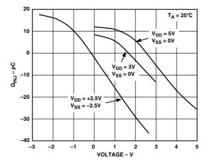
TPC 15. Charge Injection vs. Source Voltage
