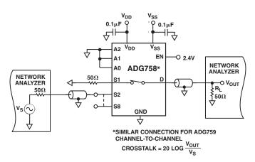
Test Circuit 10. Channel-to-Channel Crosstalk
