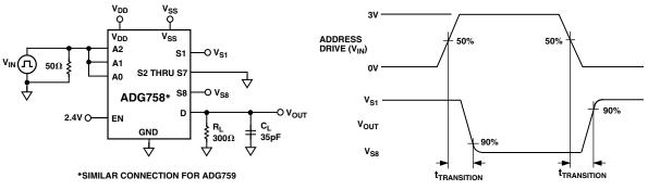
Test Circuit 5. Switching Time of Multiplexer, t<sub>TRANSITION</sub>
