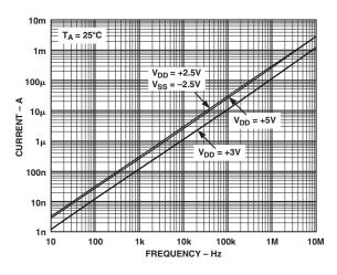
TPC 11. Supply Current vs. Input Switching Frequency
