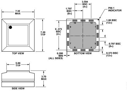
Figure 24. 12-Terminal Land Grid Array [LGA] (CC-12-1) Dimensions shown in millimeters
