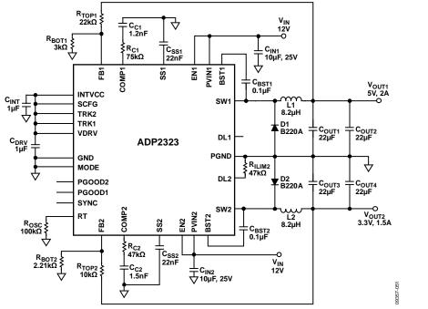
Figure 51. Using External Diode Application,  $V_{IN1} = V_{IN2} = 12 V$ ,  $V_{OUT1} = 5 V$ ,  $I_{OUT1} = 2 A$ ,  $V_{OUT2} = 3.3 V$ ,  $I_{OUT2} = 1.5 A$ ,  $f_{SW} = 600 \text{ kHz}$
