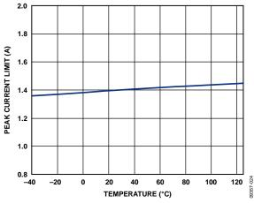
Figure 24. Current-Limit Threshold vs. Temperature,  $R_{ILIM} = 15 k\Omega$
