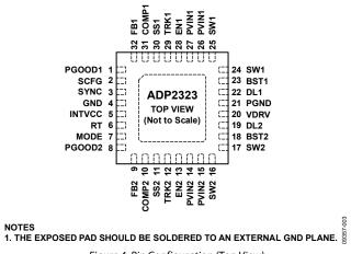
Figure 4. Pin Configuration (Top View)
