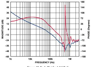
Figure 48. Bode Plot for 1.2 V Rail
