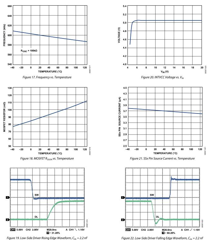
Figure 22. Low-Side Driver Falling Edge Waveform,  $C_{DL} = 2.2 \text{ nF}$
