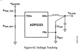
A common application is coincident tracking, which is shown in Figure 44. Coincident tracking limits the slave output voltage to be the same as the master voltage until it reaches regulation. For coincident tracking, set  $R_{TRK}$  TOP =  $R_{TOP}$  and  $R_{TRK}$  BOT =  $R_{BOT}$ .
