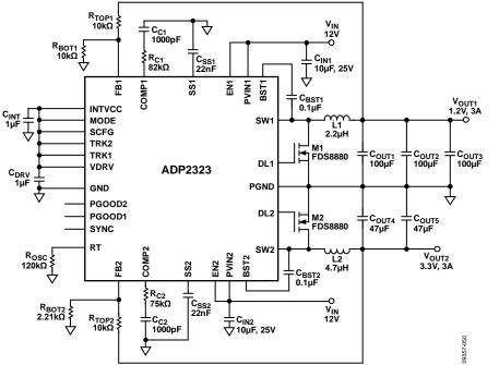
Figure 50. Using External MOSFET Application,  $V_{IN1} = V_{IN2} = 12 V$ ,  $V_{OUT1} = 1.2 V$ ,  $I_{OUT1} = 3 A$ ,  $V_{OUT2} = 3.3 V$ ,  $I_{OUT2} = 3 A$ ,  $f_{SW} = 500 \text{ kHz}$
