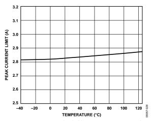
Figure 26. Current-Limit Threshold vs. Temperature,  $R_{\rm ILIM}$  = 47 k $\Omega$
