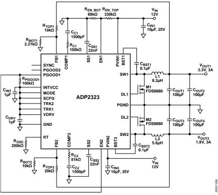
Figure 56. Programmable  $V_{IN\_RISING} = 8.7 V$ ,  $V_{IN\_FALLING} = 6.7 V$ , 3.3 V Start Up Before 1.8 V,  $V_{IN1} = V_{IN2} = 12 V$ ,  $V_{OUT1} = 3.3 V$ ,  $I_{OUT1} = 3 A$ ,  $V_{OUT2} = 1.8 V$ ,  $I_{OUT2} = 3 A$ ,  $f_{SW} = 300 \text{ kHz}$
