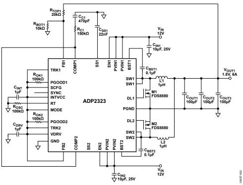
Figure 52. Parallel Single Output Application,  $V_{IN} = 12 V$ ,  $V_{OUT} = 1.8 V$ ,  $I_{OUT} = 6 A$ ,  $f_{SW} = 600 \text{ kHz}$
