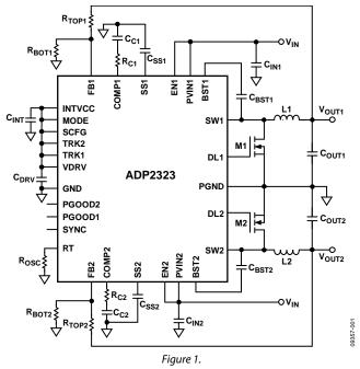
inputs and power good outputs provide reliable power sequencing. To enhance system reliability, the device also includes undervoltage lockout (UVLO), overvoltage protection (OVP), overcurrent protection (OCP), and thermal shutdown (TSD).
