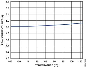
Figure 23. Current-Limit Threshold vs. Temperature, R<sub>ILIM</sub> = Floating
