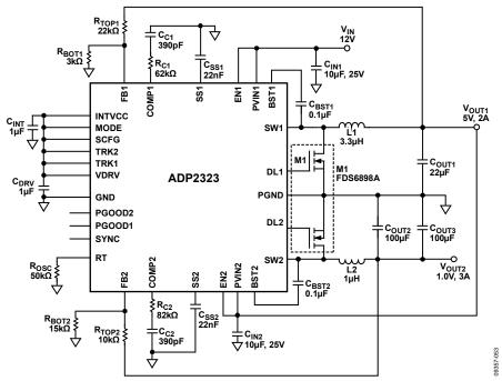
Figure 53. Cascading Supply Application, V<sub>IN1</sub> = 12 V, V<sub>OUT1</sub> = 5 V, I<sub>OUT1</sub> = 2 A, V<sub>OUT2</sub> = 1 V, I<sub>OUT2</sub> = 3 A, f<sub>SW</sub> = 1.2 MHz
