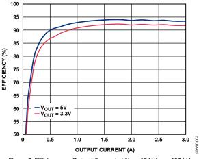
Figure 2. Efficiency vs. Output Current at  $V_{IN} = 12 V$ ,  $f_{SW} = 600 kHz$
