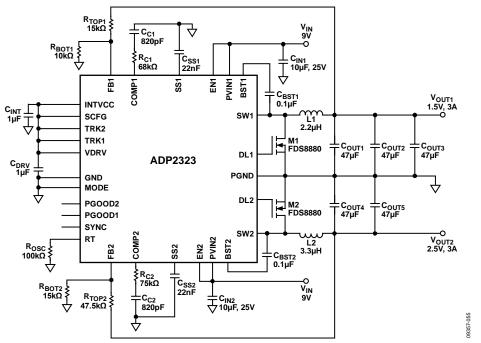
Figure 55. Enable PFM Mode with MODE Pin Pulled to GND,  $V_{IN1} = V_{IN2} = 9 V$ ,  $V_{OUT1} = 1.5 V$ ,  $I_{OUT1} = 3 A$ ,  $V_{OUT2} = 2.5 V$ ,  $I_{OUT2} = 3 A$ ,  $f_{SW} = 600 \text{ kHz}$
