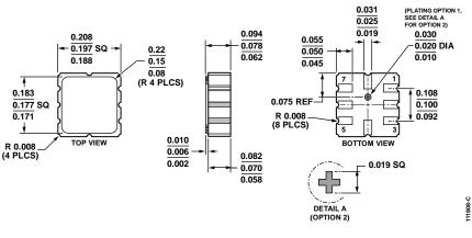
Figure 23. 8-Terminal Ceramic Leadless Chip Carrier [LCC] (E-8-1) Dimensions shown in inches
