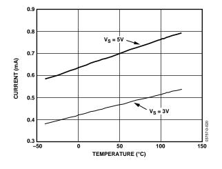
Figure 15. Supply Current vs. Temperature
