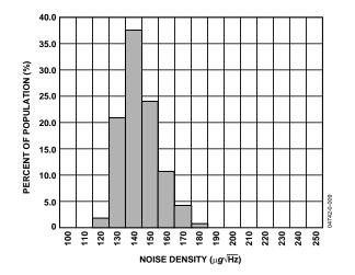
Figure 10. X Axis Noise Density at 25°C
