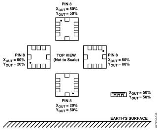
Figure 21. Output Response vs. Orientation
