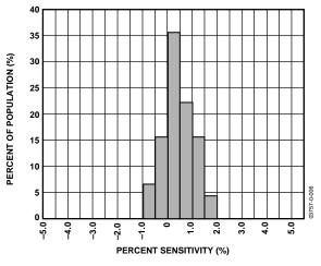
Figure 14. Z vs. Y Cross-Axis Sensitivity
