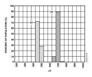
Figure 18. Supply Current at 25°C
