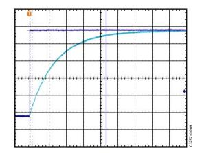
Figure 20. Turn-On Time –  $C_{X_r} C_Y = 0.1 \mu F$ , Time Scale = 2 ms/div
