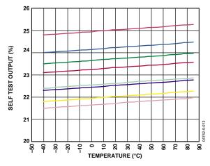
Figure 17. Self Test Response vs. Temperature
