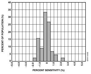
Figure 11. Z vs. X Cross-Axis Sensitivity
