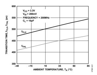
Figure 18. Transition Time vs. Ambient Temperature
