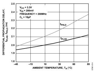
Figure 11. Differential Propagation Delay vs. Ambient Temperature
