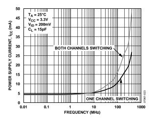
Figure 9. Power Supply Current vs. Frequency
