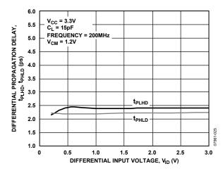
Figure 14. Differential Propagation Delay vs. Differential Input Voltage
