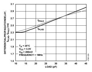
Figure 19. Differential Propagation Delay vs. Load at 1 MHz
