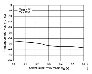
Figure 8. Threshold Voltage vs. Power Supply Voltage
