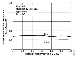
Figure 12. Differential Propagation Delay vs. Common-Mode Voltage
