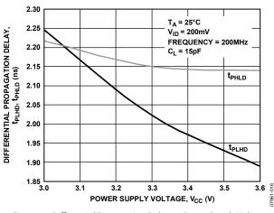
Figure 13. Differential Propagation Delay vs. Power Supply Voltage
