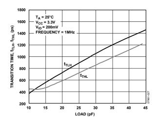
Figure 20. Transition Time vs. Load
