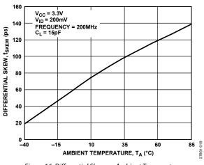
Figure 16. Differential Skew vs. Ambient Temperature
