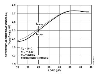
Figure 21. Differential Propagation Delay vs. Load at 200 MHz
