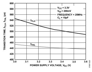
Figure 17. Transition Time vs. Power Supply Voltage
