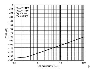
Figure 24. THD vs. Frequency, ±15 V Dual Supply
