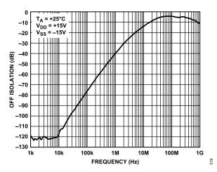
Figure 19. Off Isolation vs. Frequency, ±15 V Dual Supply
