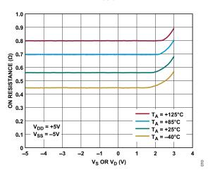
Figure 10. On Resistance vs.  $V_S$  or  $V_D$  for Various Temperatures,  $\pm 5$  V Dual Supply
