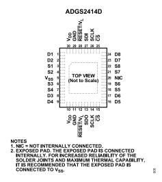
Figure 5. Pin Configuration
