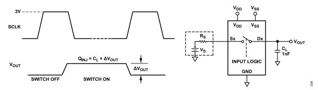
Figure 39. Charge Injection,  $Q_{INJ}$  ( $\Delta V_{OUT}$  = Change in Output Voltage)
