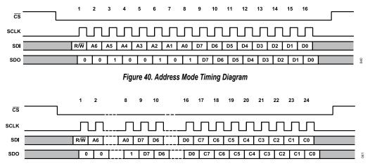
Figure 41. Timing Diagram with CRC Enabled
