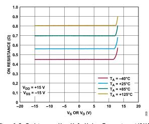
Figure 9. On Resistance vs.  $V_S$  or  $V_D$  for Various Temperatures,  $\pm 15$  V Dual Supply
