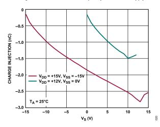
Figure 20. Charge Injection vs. V<sub>S</sub>
