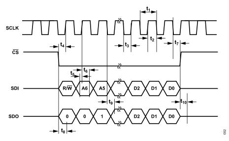
Figure 2. Address Mode Timing Diagram
