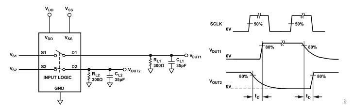
Figure 37. Break-Before-Make Time Delay, t<sub>D</sub>
