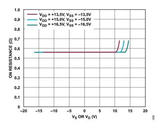
Figure 6. On Resistance vs. V<sub>S</sub> or V<sub>D</sub> for ±15 V Dual Supply
