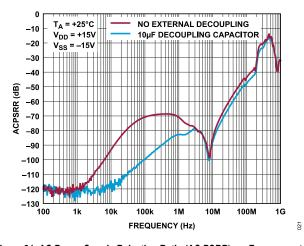
Figure 21. AC Power Supply Rejection Ratio (AC PSRR) vs. Frequency, ±15 V Dual Supply
