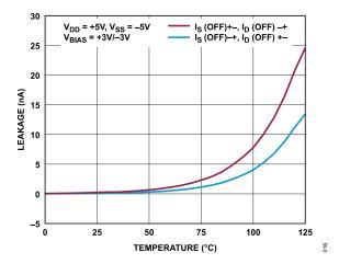
Figure 16. On Leakage Currents vs. Temperature, ±5 V Dual Supply
