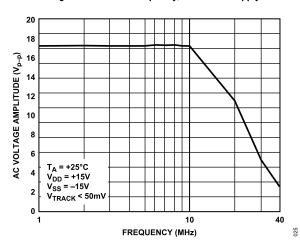
Figure 25. Large AC Signal Voltage vs. Frequency
