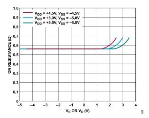
Figure 7. On Resistance vs. V<sub>S</sub> or V<sub>D</sub> for ±5 V Dual Supply
