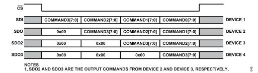
Figure 45. Example of an SPI Frame Where Four ADGS2414D Devices Connect in Daisy-Chain Mode
