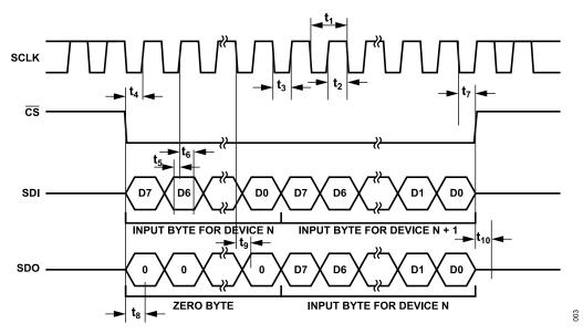
Figure 3. Daisy-Chain Timing Diagram
