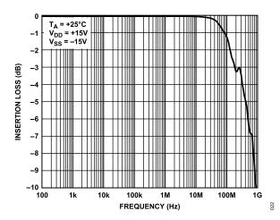
Figure 22. Insertion Loss vs. Frequency, ±15 V Dual Supply
