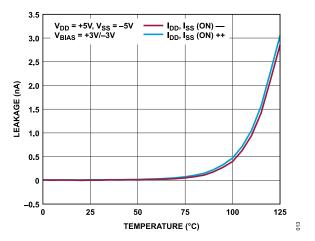
Figure 13. On Leakage Currents vs. Temperature, ±5 V Dual Supply
