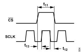
Figure 4. SCLK and CS Timing Relationship
