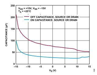
Figure 26. Capacitance vs. V<sub>S</sub>, ±15 V Dual Supply
