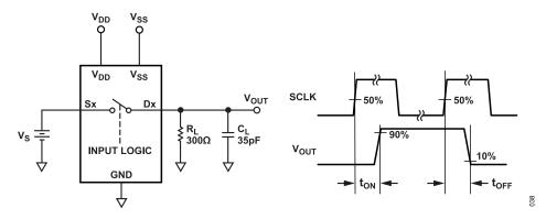
Figure 38. Switching Times,  $t_{\text{ON}}$  and  $t_{\text{OFF}}$
