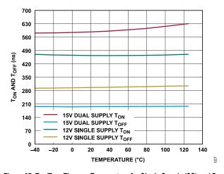
Figure 27.  $T_{ON}/T_{OFF}$  Time vs. Temperature for Single Supply (SS) and Dual Supply (DS)
