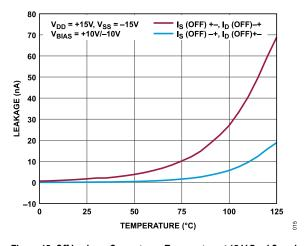
Figure 15. Off Leakage Currents vs. Temperature, ±15 V Dual Supply
