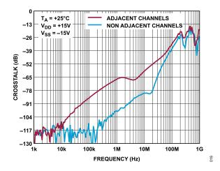
Figure 18. Crosstalk vs. Frequency, ±15 V Dual Supply
