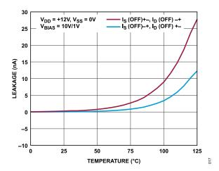
Figure 17. On Leakage Currents vs. Temperature, +12 V Single Supply
