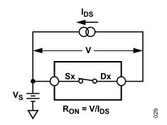
Figure 29. On Resistance ( $I_{DS}$  = Drain and Source Current)
