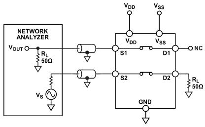
CHANNEL TO CHANNEL CROSSTALK = 20 log  $\frac{V_{OUT}}{V_S}$
