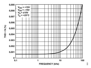
Figure 23. THD + N vs. Frequency, ±15 V Dual Supply
