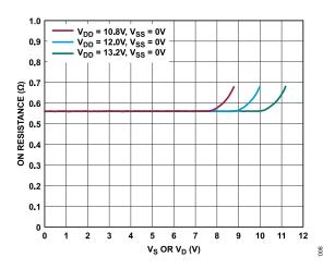
Figure 8. On Resistance vs. V<sub>S</sub> or V<sub>D</sub> for +12 V Single Supply
