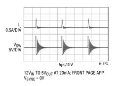
Figure 2. Burst Mode Operation
