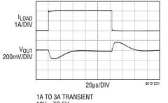
1A TO 3A TRANSIEN 12V<sub>IN</sub> TO 5V<sub>OUT</sub> C<sub>OUT</sub> = 2×47µF FRONT PAGE APP
