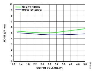
Figure 42. RMS Output Noise vs. Output Voltage, Load Current = 100 mA
