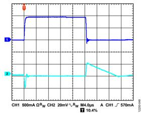
Figure 47. Load Transient Response,  $I_{LOAD} = 10$  mA to 1 A,  $V_{OUT} = 5$  V,  $V_{IN} = 5.5$  V, CH1 =  $I_{LOAD}$ , CH2 =  $V_{OUT}$
