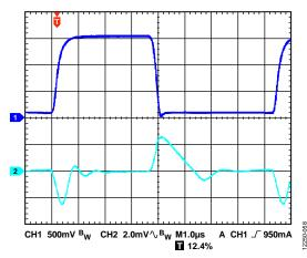
Figure 57. Output Transient Response,  $V_{OUT} = 5 V$ ,  $C_{OUT} = 4.7 \mu F$
