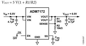
Figure 56. Typical Adjustable Output Voltage Application Schematic
