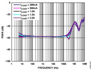
Figure 36. Power Supply Rejection Ratio (PSRR) vs. Frequency, 800 mV Headroom,  $V_{OUT} = 5 V$
