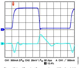
Figure 48. Load Transient Response,  $I_{LOAD} = 100$  mA to 1.6 A,  $V_{OUT} = 5$  V,  $V_{IN} = 5.5$  V,  $CH1 = I_{LOAD}$ ,  $CH2 = V_{OUT}$
