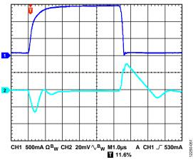
Figure 50. Load Transient Response,  $I_{LOAD} = 100$  mA to 1.6 A, Adjustable Version,  $V_{OUT} = 1.2$  V,  $V_{IN} = 2.5$  V,  $CH1 = I_{LOAD}$ ,  $CH2 = V_{OUT}$
