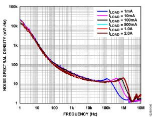
Figure 45. Output Noise Spectral Density,  $V_{OUT} = 5 V$
