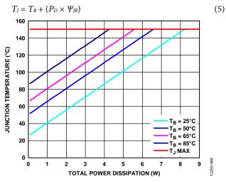
Figure 67. LFCSP Power Dissipation for Various Board Temperatures
