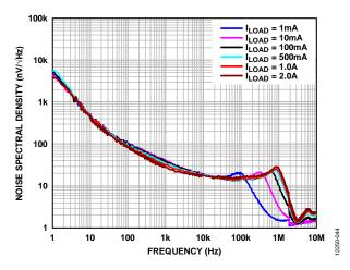
Figure 43. Output Noise Spectral Density, Adjustable Version,  $V_{OUT} = 1.2 V$
