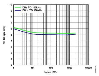
Figure 39. RMS Output Noise vs. Load Current ( $I_{LOAD}$ ), Adjustable Version,  $V_{OUT} = 1.2 V$
