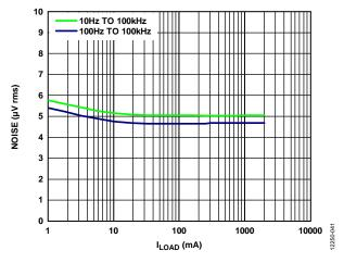
Figure 40. RMS Output Noise vs. Load Current (ILOAD), VOUT = 3 V
