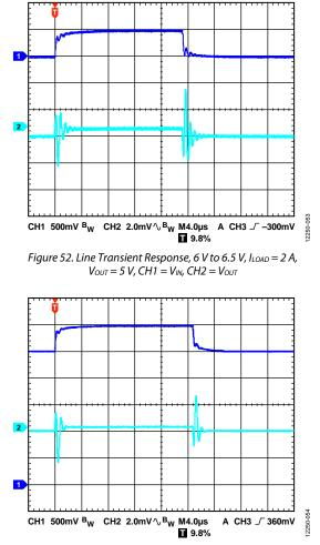
Figure 53. Line Transient Response, 2.5 V to 3 V,  $I_{LOAD} = 500$  mA, Adjustable Version,  $V_{OUT} = 1.2$  V,  $CH1 = V_{IN}$ ,  $CH2 = V_{OUT}$
