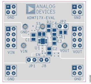
Figure 70. Example LFCSP PCB Layout
