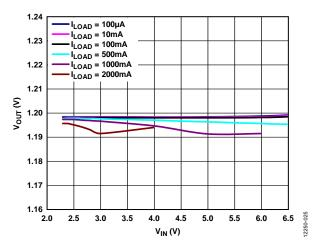
Figure 25. Output Voltage ( $V_{OUT}$ ) vs. Input Voltage ( $V_{IN}$ ), Adjustable Version,  $V_{OUT} = 1.2 V$
