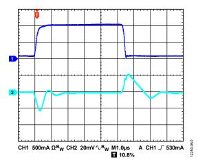
Figure 49. Load Transient Response,  $I_{LOAD} = 10$  mA to 1 A, Adjustable Version,  $V_{OUT} = 1.2$  V,  $V_{IN} = 2.5$  V,  $CH1 = I_{LOAD}$ ,  $CH2 = V_{OUT}$
