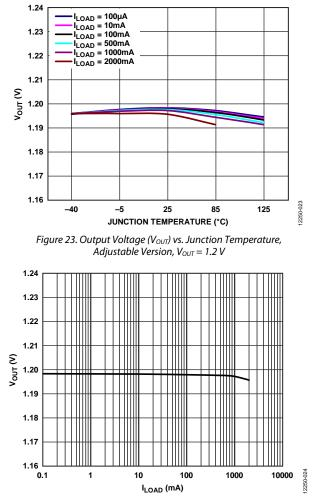
Figure 24. Output Voltage (V\_{OUT}) vs. Load Current (I\_LOAD), Adjustable Version,  $V_{OUT} = 1.2 V$
