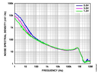
Figure 46. Output Noise Spectral Density, Different Output Voltages, Load Current = 100 mA
