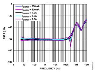
Figure 32. Power Supply Rejection Ratio (PSRR) vs. Frequency, 800 mV Headroom, Vour = 3 V
