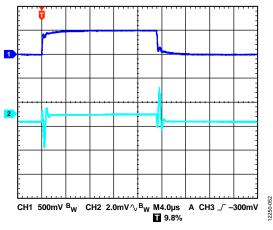
Figure 51. Line Transient Response, 6 V to 6.5 V,  $I_{LOAD} = 500 \text{ mA}$ ,  $V_{OUT} = 5 \text{ V}$ , CH1 =  $V_{IN}$ , CH2 =  $V_{OUT}$
