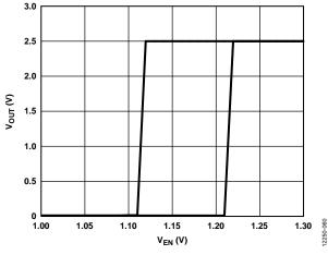
Figure 59. Typical VOUT Response to EN Pin Operation
