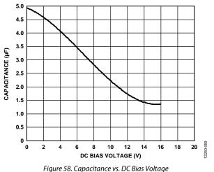
Use Equation 1 to determine the worst-case capacitance accounting for capacitor variation over temperature, component tolerance, and voltage.
