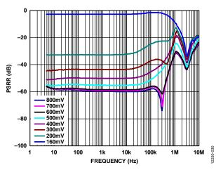
Figure 30. Power Supply Rejection Ratio (PSRR) vs. Frequency, V<sub>OUT</sub> = 3 V, 2 A Load Current, Various Headroom Voltages
