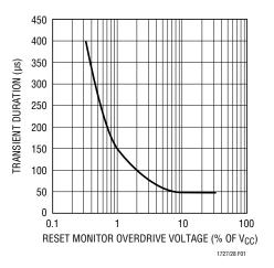
Figure 1. Transient Duration vs Comparator Overdrive
