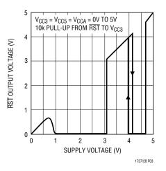
Figure 3. RST Voltage vs Supply Voltage
