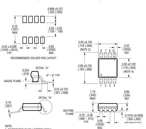
**MS8** Package 8-Lead Plastic MSOP (Reference LTC DWG # 05-08-1660 Rev G)
