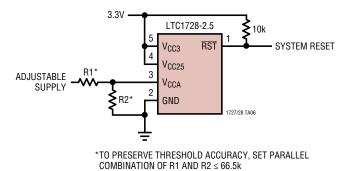
Using  $V_{CCA}$  Tied to DC/DC Feedback Divider
