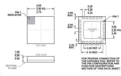
24-Terminal Ceramic Leadless Chip Carrier [LCC] (E-24-1)
