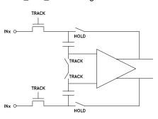
Figure 11: Input configuration
