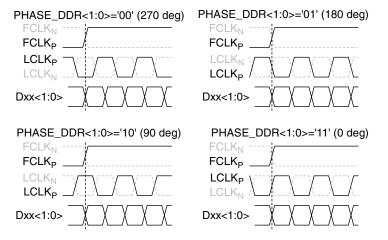
Figure 10: Phase programmability modes for LCLK
