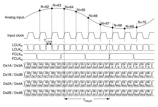
Figure 5: Dual channel - LVDS timing 8-bit output
