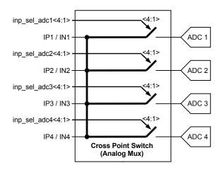
Figure 8: ADC input signals through Cross Point Switch
