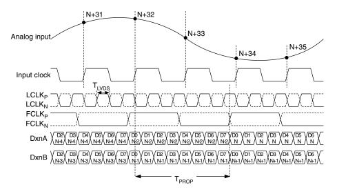
Figure 4: Quad channel - LVDS timing 8-bit output
