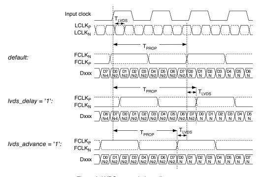
Figure 9: LVDS output timing adjustment
