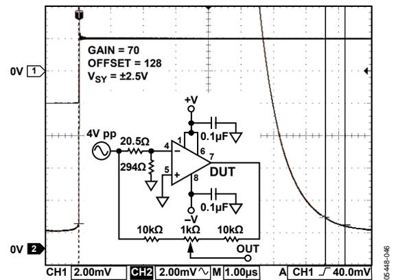
Figure 45. Settling Time 0.01%
