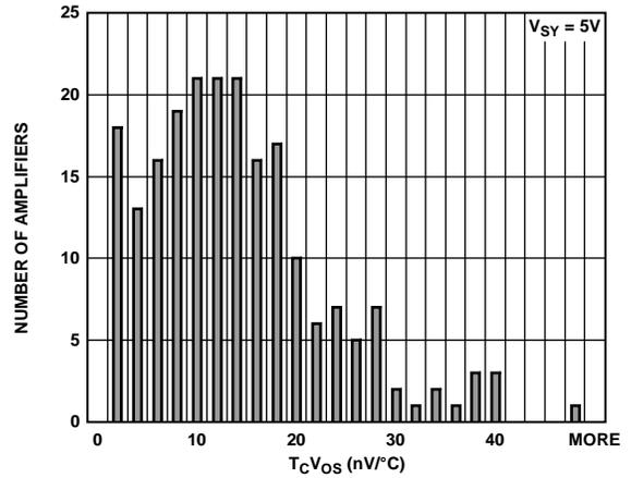
Figure 7. TcV<sub>Os</sub> at V<sub>Sy</sub> = 5V
