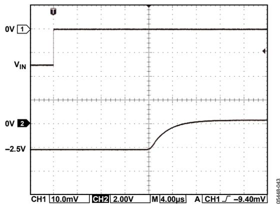
Figure 42. Negative Overload Recovery (Gain = 1280)
