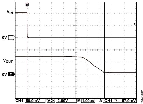
Figure 41. Positive Overload Recovery (Gain = 70)
