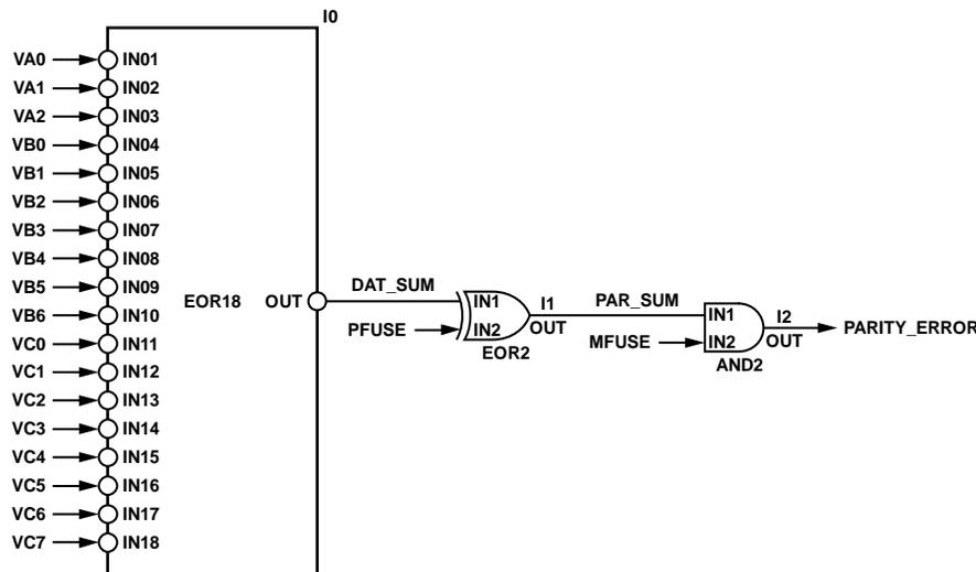
Figure 50. Functional Circuit of AD8556 Parity Check
