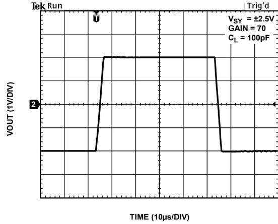
Figure 37. Large Signal Response at  $C_L = 100\text{ pF}$
