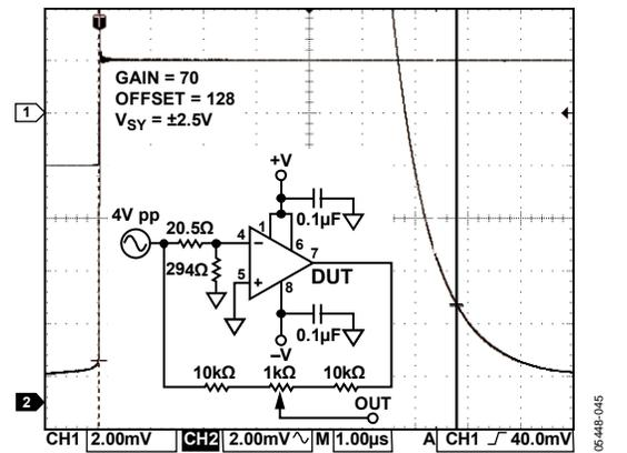
Figure 44. Settling Time 0.1%
