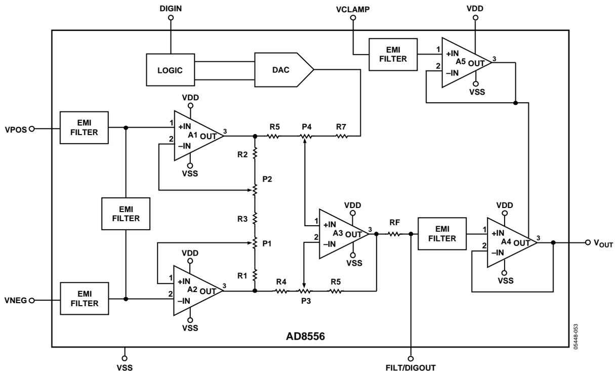
Figure 51. Block Diagram Showing EMI/RFI Built-In Filters
