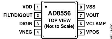
Figure 2. 8-Lead SOIC\_N Pin Configuration
