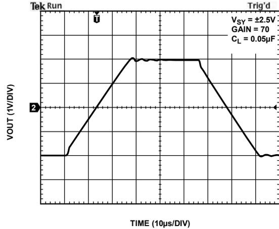
Figure 38. Large Signal Response at  $C_L = 0.05\text{ }\mu\text{F}$
