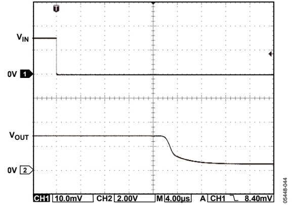
Figure 43. Positive Overload Recovery (Gain = 1280)
