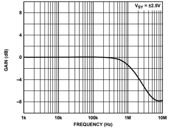
Figure 25. Output Buffer Gain vs. Frequency
