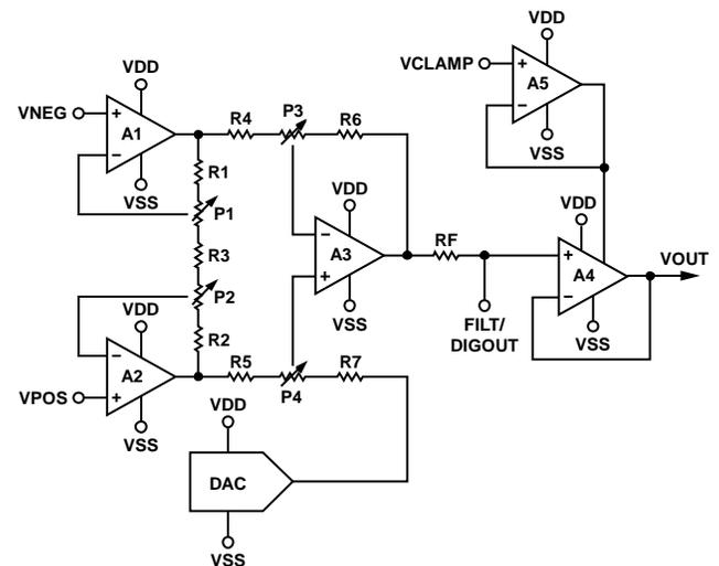
Figure 47. Functional Schematic
