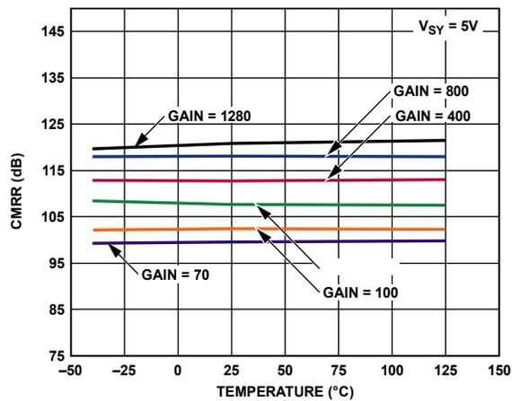
Figure 18. CMRR vs. Temperature at Different Gains
