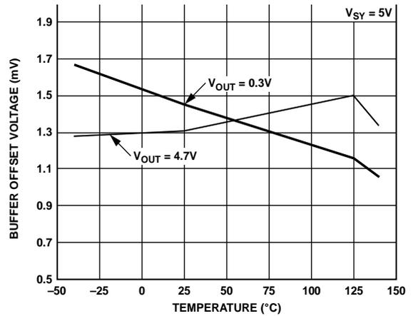
Figure 8. Output Buffer Offset Voltage vs. Temperature
