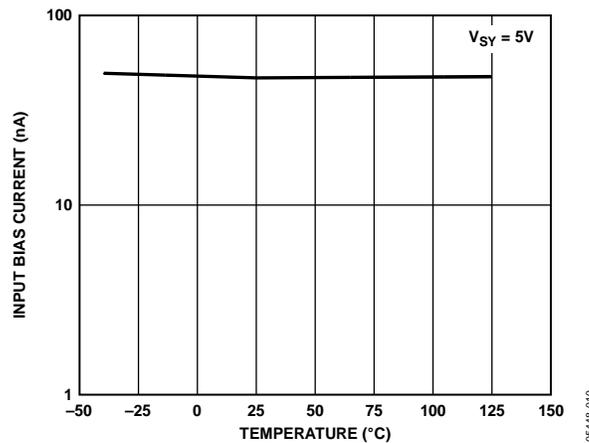
Figure 9. Input Bias Current at V<sub>POS</sub>, V<sub>NEG</sub> vs. Temperature
