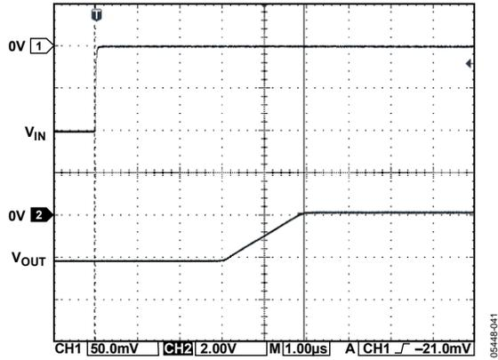
Figure 40. Negative Overload Recovery (Gain = 70)
