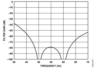
Figure 69. 16.667 SPS ODR, 60 ms Settling Time (40 – 70 Hz)
