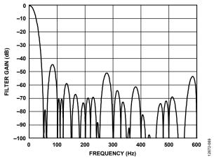
Figure 68. 16.667 SPS ODR, 60 ms Settling Time
