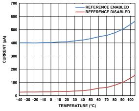
Figure 37. Current Consumption vs. Temperature (Standby Mode)
