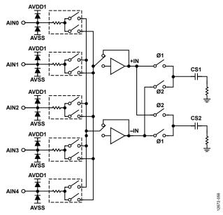
Figure 54. Simplified Analog Input Circuit
