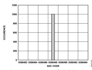
Figure 14. Histogram (Analog Input Buffers Enabled,  $V_{REF} = 5 V$ , Output Data Rate = 1.25 SPS)
