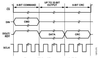
Figure 74. SPI Read Transaction with CRC
