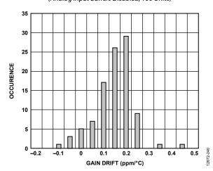
Figure 34. Gain Drift Distribution Histogram (Analog Input Buffers Enabled, 100 Units)
