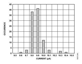
Figure 39. Burnout Current Distribution Histogram (100 Units)
