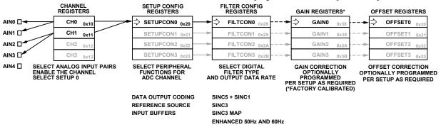
Figure 50. Two Fully Differential Inputs, Both Using a Single Setup (SETUPCONO; FILTCONO; GAINO; OFFSETO)
