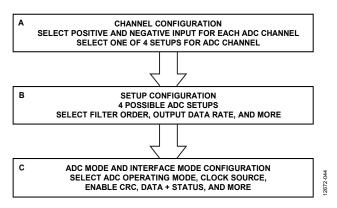
Figure 48. Suggested ADC Configuration Flow
