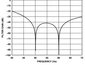
Figure 65. 27.27 SPS ODR, 36.67 ms Settling Time (40 – 70 Hz)
