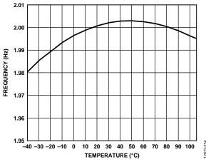
Figure 28. Internal Oscillator Frequency vs. Temperature
