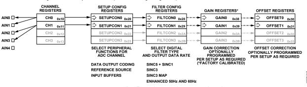
Figure 51. Two Fully Differential Inputs with a Setup per Channel
