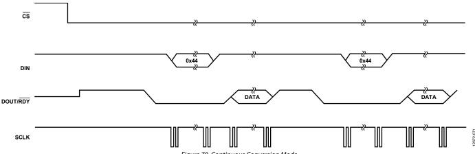
Figure 70. Continuous Conversion Mode
