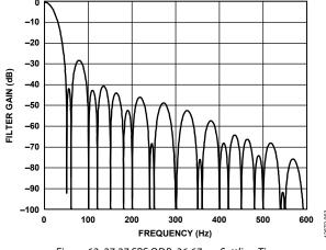
Figure 62. 27.27 SPS ODR, 36.67 ms Settling Time
