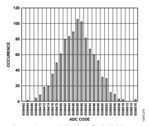
Figure 15. Histogram (Analog Input Buffers Enabled,  $V_{REF} = 5 V$ , Output Data Rate = 2.6 kSPS)
