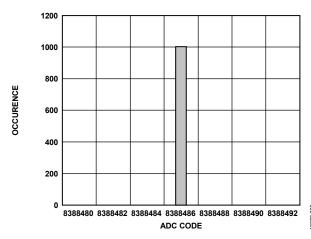
Figure 8. Histogram (Analog Input Buffers Disabled, V<sub>REF</sub> = 5 V, Output Data Rate = 1.25 SPS)
