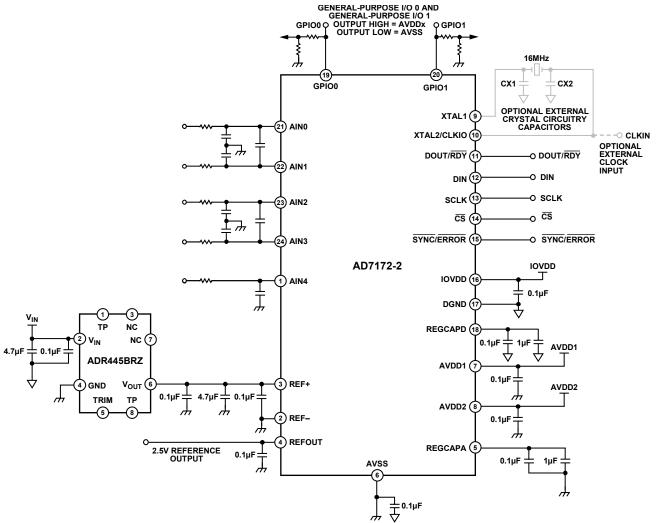
Figure 42. Typical Connection Diagram
