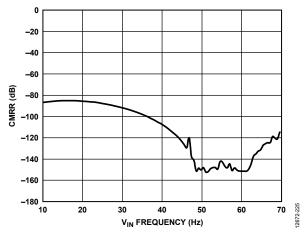
Figure 19. Common-Mode Rejection Ratio (CMRR) vs.  $V_{IN}$  Frequency ( $V_{IN} = 0.1 \text{ V}$ , 10 Hz to 70 Hz, Output Data Rate = 20 SPS, Enhanced Filter)
