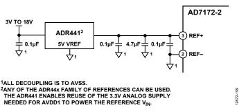
Figure 55. External Reference (ADR441) Connected to AD7172-2 Reference Pins
