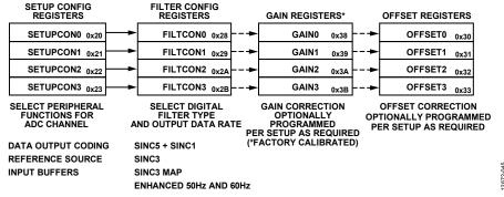
Figure 49. ADC Setup Register Grouping
