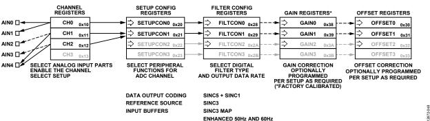
Figure 52. Mixed Differential and Single-Ended Configuration Using Multiple Shared Setups Rev. A | Page 26 of 60
