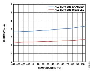
Figure 36. Current Consumption vs. Temperature (Continuous Conversion Mode)
