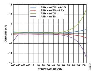
Figure 41. Analog Input Current vs. Temperature
