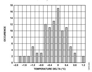
Figure 38. Temperature Sensor Distribution Histogram (Uncalibrated, 100 Units)
