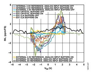
Figure 21. Integral Nonlinearity (INL) vs. V<sub>IN</sub> (Differential Input)
