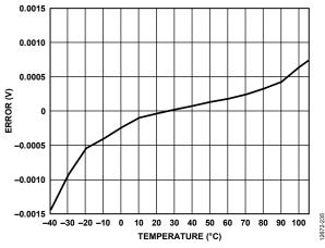
Figure 29. Absolute Reference Error vs. Temperature
