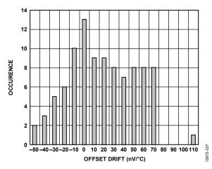
Figure 31. Offset Error Drift Distribution Histogram (Internal Short, 100 Units)
