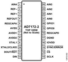
Figure 4. Pin Configuration
