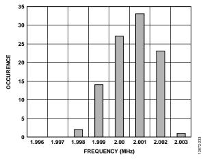
Figure 27. Internal Oscillator Frequency Distribution Histogram (100 Units)
