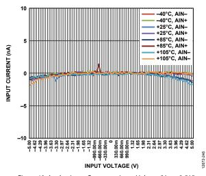
Figure 40. Analog Input Current vs. Input Voltage ( $V_{CM} = 2.5 V$ )
