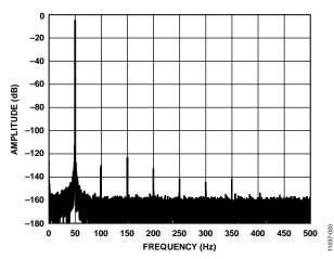
Figure 15. 50 Hz Input Tone, -6 dBFS Input FFT ( $V_{REF} = 2.5 V$  Output Data Rate = 1 kSPS)
