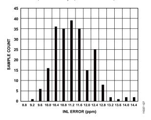
Figure 27. Integral Nonlinearity (INL) Distribution Histogram (Differential Input,  $V_{REF} = 2.5 \text{ V Internal}$ )
