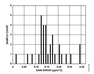
Figure 34. Gain Error Drift Distribution Histogram
