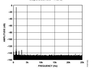
Figure 16. 1 kHz Input Tone, -6 dBFS Input FFT ( $V_{REF} = 2.5 V$ , Output Data Rate = 50 kSPS)
