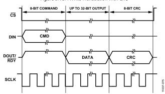
Figure 68. SPI Read Transaction with CRC
