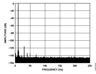
Figure 14. 1 kHz Input Tone, -0.5 dBFS Input FFT ( $V_{REF} = 2.5 V$ , Output Data Rate = 50 kSPS)
