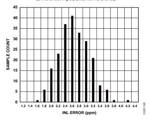
Figure 25. Integral Nonlinearity (INL) Distribution Histogram (Differential Input,  $V_{REF} = 2.5V$  External)
