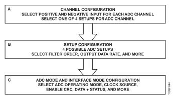
Figure 41. Suggested ADC Configuration Flow
