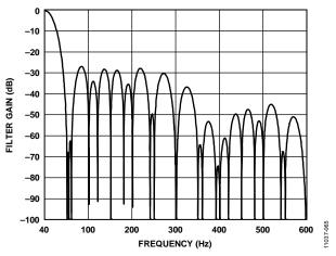
Figure 57. 25 SPS ODR, 40 ms Settling Time
