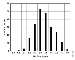
Figure 26. Integral Nonlinearity (INL) Distribution Histogram (Differential Input, V<sub>REF</sub> = 5 V External)
