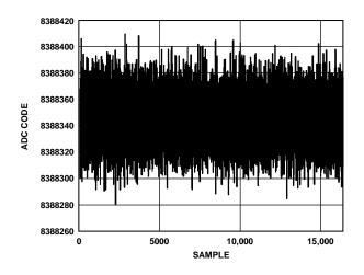
Figure 7. Noise ( $V_{REF} = 5 V$ , Output Data Rate = 250 kSPS)
