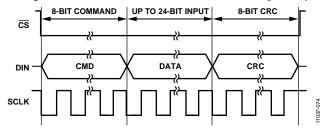
Figure 67. SPI Write Transaction with CRC
