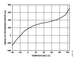
Figure 30. Absolute Reference Error vs. Temperature
