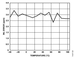
Figure 28. Integral Nonlinearity (INL) vs. Temperature (Differential Input,  $V_{REF} = 2.5 V$ )
