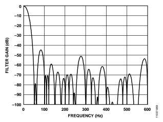
Figure 62. 16.667 SPS ODR, 60 ms Settling Time
