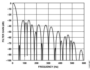
Figure 58. 20 SPS ODR, 50 ms Settling Time
