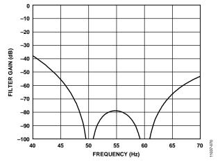
Figure 63. 16.667 SPS ODR, 60 ms Settling Time
