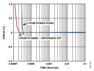
Figure 21. Internal Reference Settling Time
