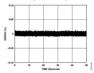
Figure 19. Internal Reference Settling Time (Extended)
