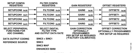
Figure 42. ADC Setup Register Grouping
