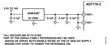
Figure 49. External Reference ADR445 Connected to AD7176-2 Reference Pins
