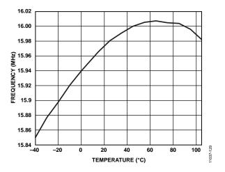
Figure 29. Internal Oscillator Frequency vs. Temperature
