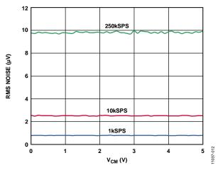
Figure 11. Noise vs. Common-Mode Input Voltage  $(V_{REF} = 2.5 V)$
