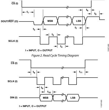
Figure 3. Write Cycle Timing Diagram Rev. D | Page 7 of 68
