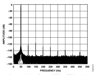
Figure 13. 50 Hz Input Tone, -0.5 dBFS Input FFT ( $V_{REF} = 2.5 V$ , Output Data Rate = 1 kSPS)
