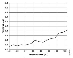
Figure 35. Current Consumption vs Temperature (Continous Conversion Mode)
