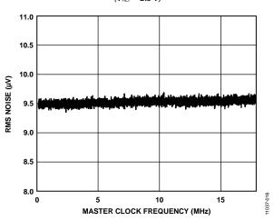
Figure 12. Noise vs. Master Clock  $(V_{REF} = 2.5 V)$
