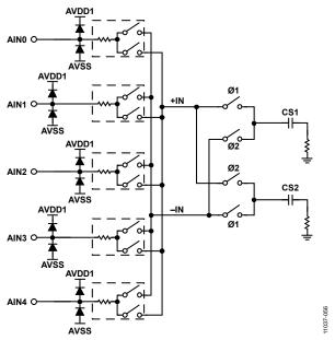
Figure 46. Simplified Analog Input Circuit
