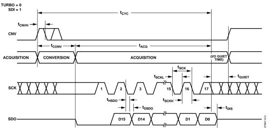
Figure 29. CS Mode, 3-Wire with Busy Indicator Serial Interface Timing (SDI High)
