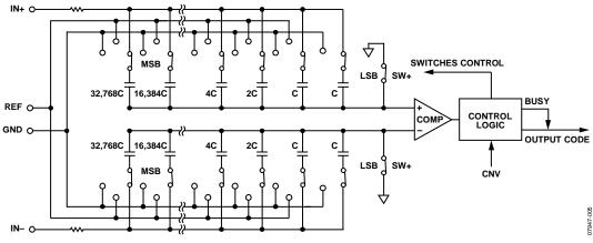
Figure 21. ADC Simplified Schematic
