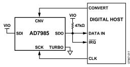
*Figure 28.* CS *Mode, 3-Wire with Busy Indicator Connection Diagram (SDI High)*
