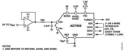
Figure 23. Typical Application Diagram with Multiple Supplies
