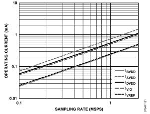
*Figure 25. Operating Current vs. Sampling Rate in Normal Mode*
