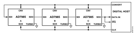
Figure 36. Chain Mode with Busy Indicator Connection Diagram
