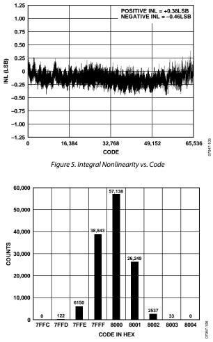
Figure 6. Histogram of DC Input at Code Center (External Reference)
