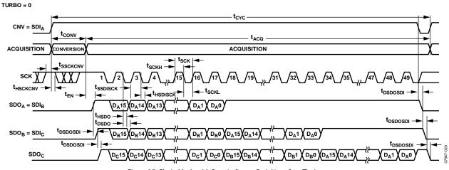
Figure 37. Chain Mode with Busy Indicator Serial Interface Timing
