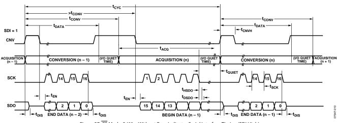
Figure 27. CS Mode, 3-Wire Without Busy Indicator Serial Interface Timing (SDI High)
