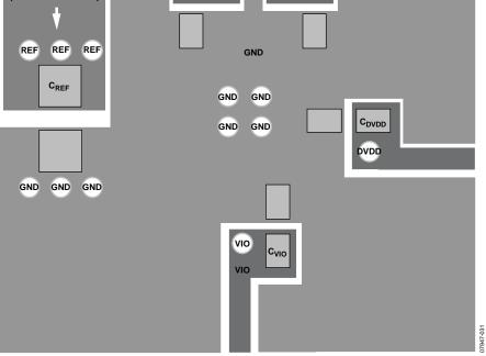
Figure 39. Example Layout of the AD7985 (Bottom Layer)
