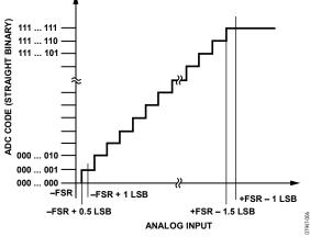
Figure 22. ADC Ideal Transfer Function
