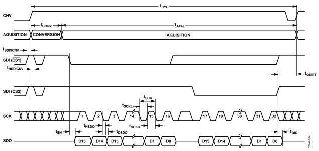
Figure 31. CS Mode, 4-Wire Without Busy Indicator Serial Interface Timing
