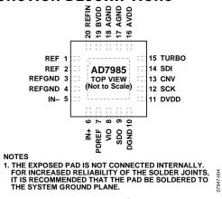
Figure 4. Pin Configuration
