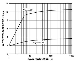
Figure 1. Output Swing vs. Load Resistance
