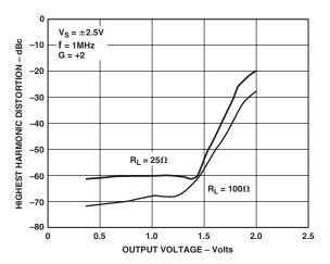
TPC 15. Distortion vs. Output Voltage,  $V_S = \pm 2.5 \text{ V}$ , G = +2, f = 1 MHz
