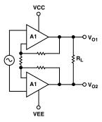
Figure 8. Differential Driver Simplified Circuit Schematic
