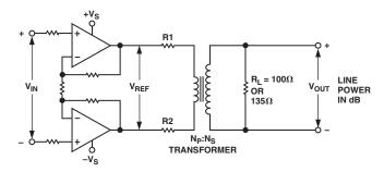
Figure 2. Differential Drive Circuit for xDSL Applications
