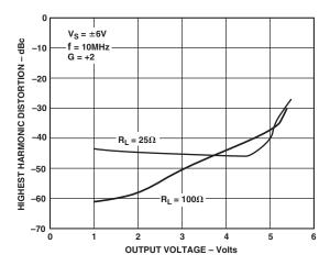
TPC 13. Distortion vs. Output Voltage,  $V_S = \pm 6 \text{ V}$ , G = +2, f = 10 MHz
