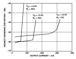
TPC 10. Distortion vs. Output Current;  $V_S = \pm 2.5 \text{ V}$ , f = 1 MHz, G = +2
