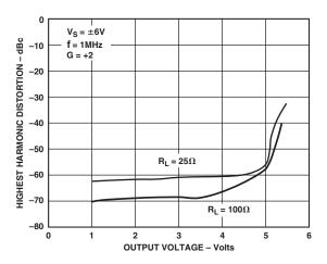
TPC 12. Distortion vs. Output Voltage,  $V_S = \pm 6 \text{ V}$ , G = +2, f = 1 MHz
