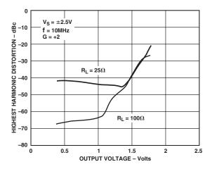
TPC 16. Distortion vs. Output Voltage,  $V_S = \pm 2.5 \text{ V}$ , G = +2, f = 10 MHz
