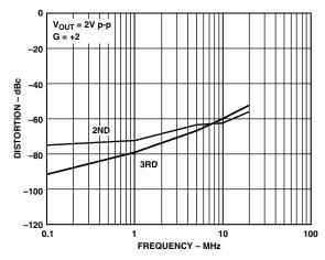
TPC 8. Distortion vs. Frequency;  $V_S$  =  $\pm 2.5$  V,  $R_L$  = 100  $\Omega$
