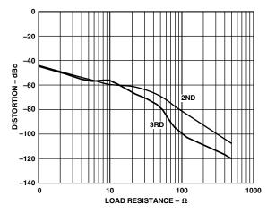
TPC 14. Distortion vs.  $R_L$ ,  $V_S = \pm 2.5$  V, G = +2,  $V_{OUT} = 2$  V p-p, f = 1 MHz
