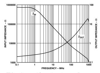
TPC 31. Input and Output Impedance vs. Frequency
