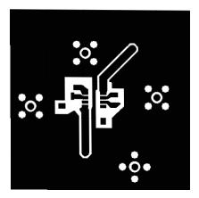
Figure 12. Universal SOIC Noninverter Bottom
