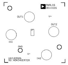
Figure 10. Universal SOIC Noninverter Top Silkscreen
