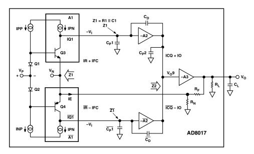
Figure 6. Simplified Block Diagram
