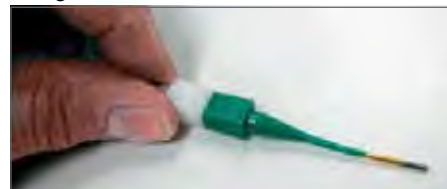
Plastic tool with contact in proper position.
