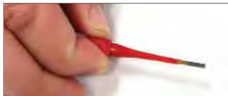
Plastic tool with contact in proper position.
