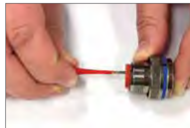
Plastic tool with contact in proper position.
