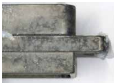
After 1560 Hours Salt Spray of Durmalon Plated Micro-D Shell
