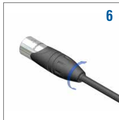
Thread the nut (Backshell) onto the shell (Torque 0.8Nm - 1.2Nm) to activate the cable clamp and close the connector assembly.
