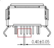
**4.** For market trend of high durability, shell material changed to stainless steel can meet more than 10000 cycle times.
