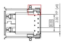
**3.** Decreasing the width of terminal to aviod damage while connector mounting on PCB.
