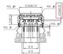
**2.** The gap increasing between shell and PCB is to avoid short circuit and raise safety factor, and stand-off area change of housing is to avoid soldering overlapping.
