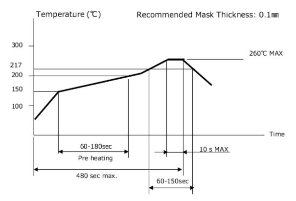
Temperature on the surface of PWB
