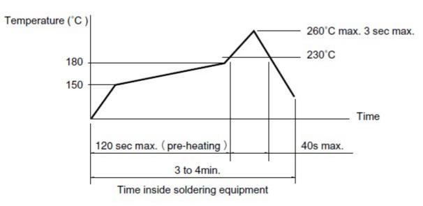
(1) The above temperature shall be measured of the top of switch. There are cases where PC board's temperature greatly differs from that of the switch, depending on the material, size, thickness of PC board's and others. Care, should be taken to prevent the switch's surface temperature from exceeding  $260^{\circ}$ C.
