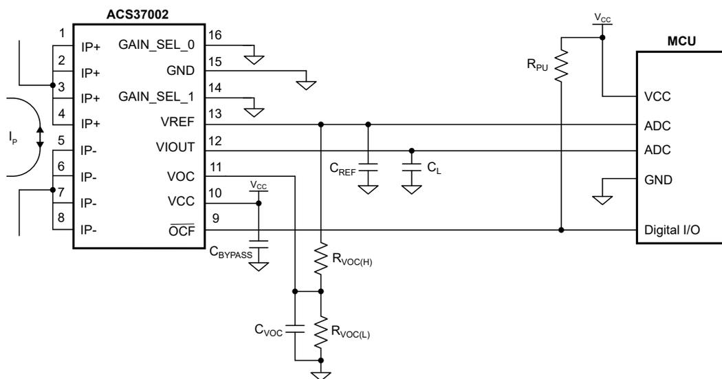
**Figure 1: Typical Bidirectional Application Showing 00 Gain Select Configuration.**
