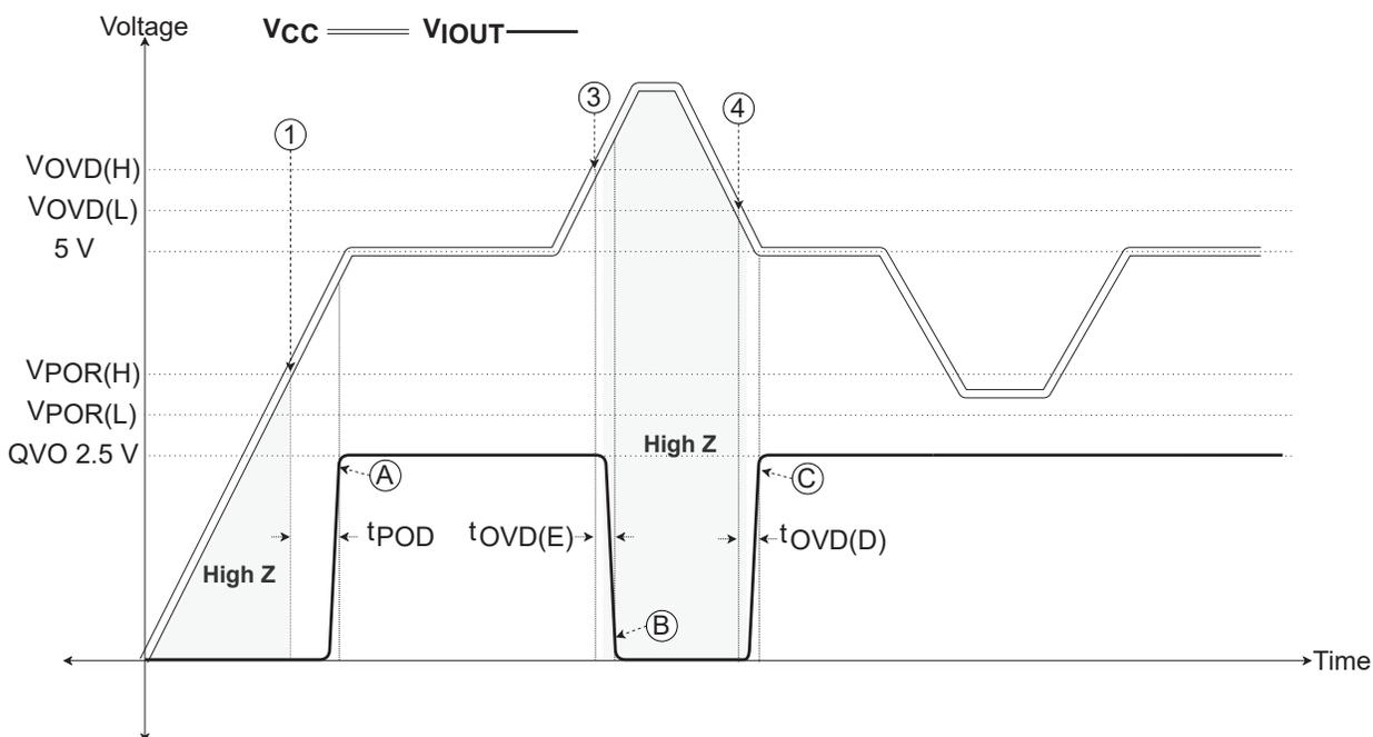
Figure 6:  $t_{POD}$  and  $t_{OVD(E/D)}$  with  $R_L = \text{Pull-Up}$
