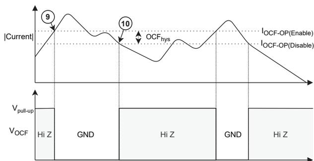
Figure 11: Fault Thresholds and OCF Pin Functionality
