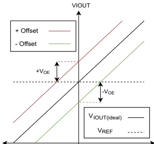
Figure 7: Offset ( $V_{OE}$ ) Between  $V_{IOUT}$  and  $V_{REF}$
