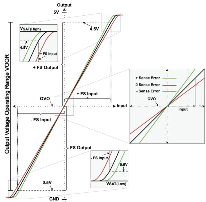
Figure 8:  $V_{OOR}$ ,  $V_{SAT}$  and SENS with Full Scale
