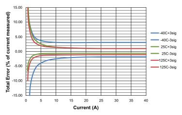
Figure 3: Predicted Total Error as a Function of Sensed Current for the ACS723KMATR-40AB
