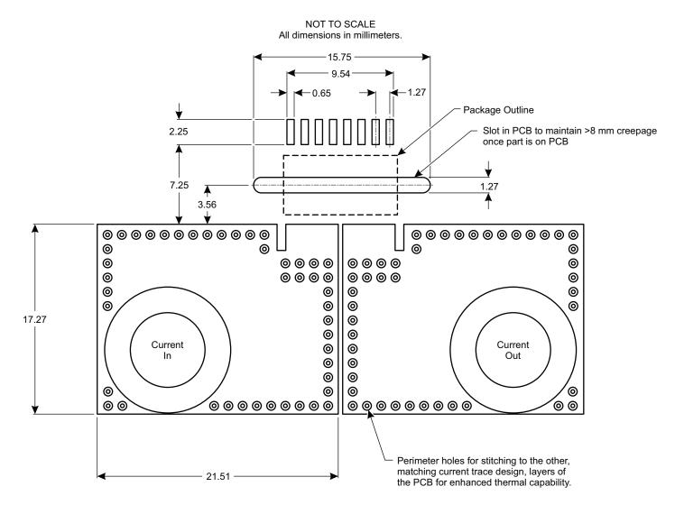
Figure 7: High-Isolation PCB Layout
