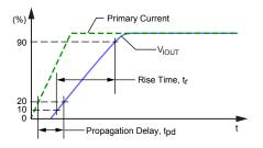
Figure 5: Rise Time and Propagation Delay
