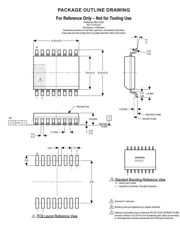
Figure 8: Package MA, 16-pin SOICW
